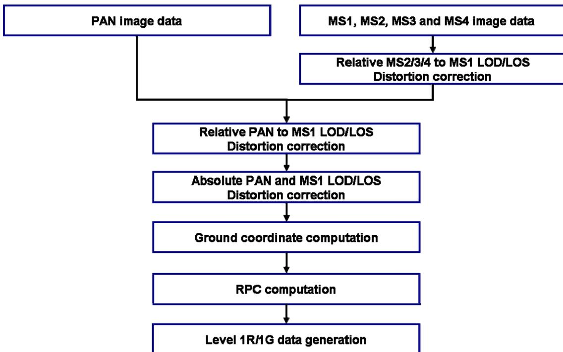
Figure 5 Workflow of KOMPSAT-2 geometric correction preprocessing
