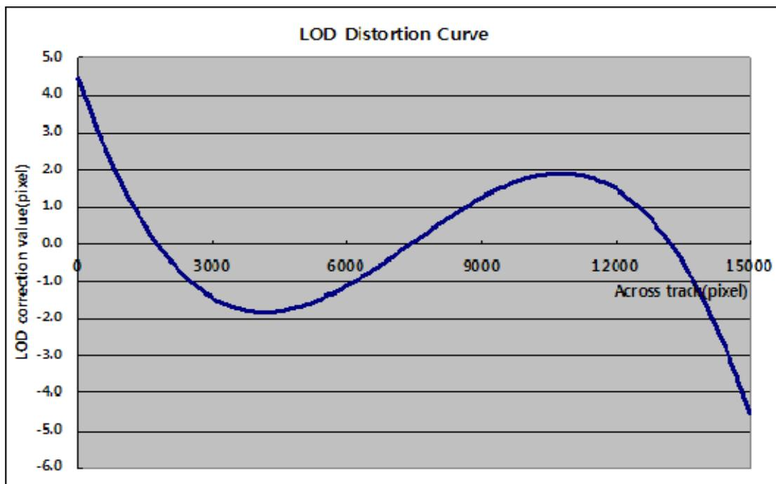
Figure 7 Absolute PAN LOD distortion curve
