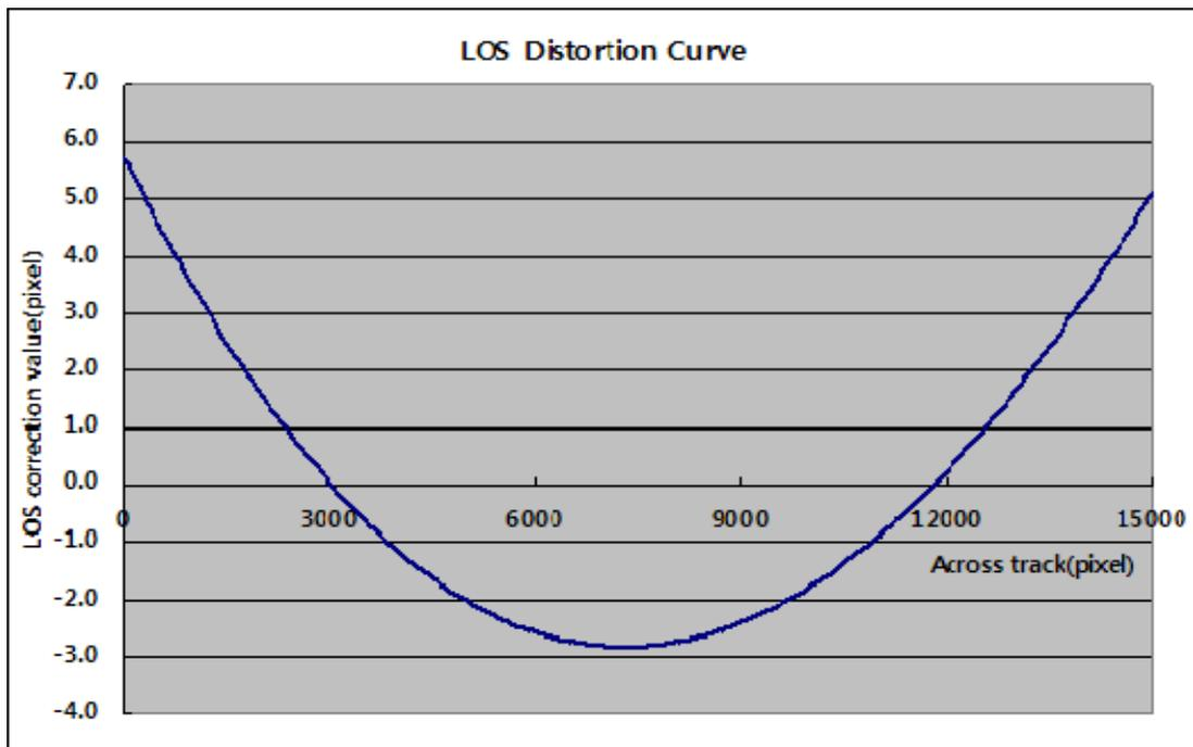
Figure 6 Absolute PAN LOS distortion curve
