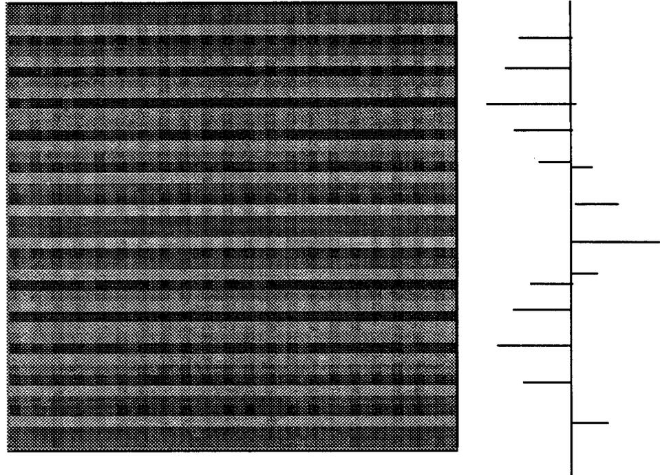
**FIGURE 5. VNIR band 1, zoom x 12, horizontal striping**
