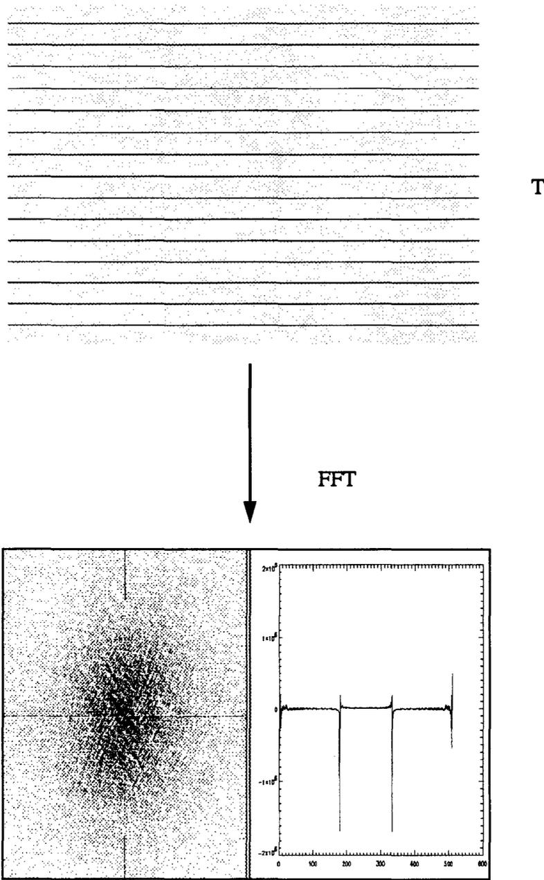
**FIGURE 6.** an horizontal two-dimension signal, and its FFT
