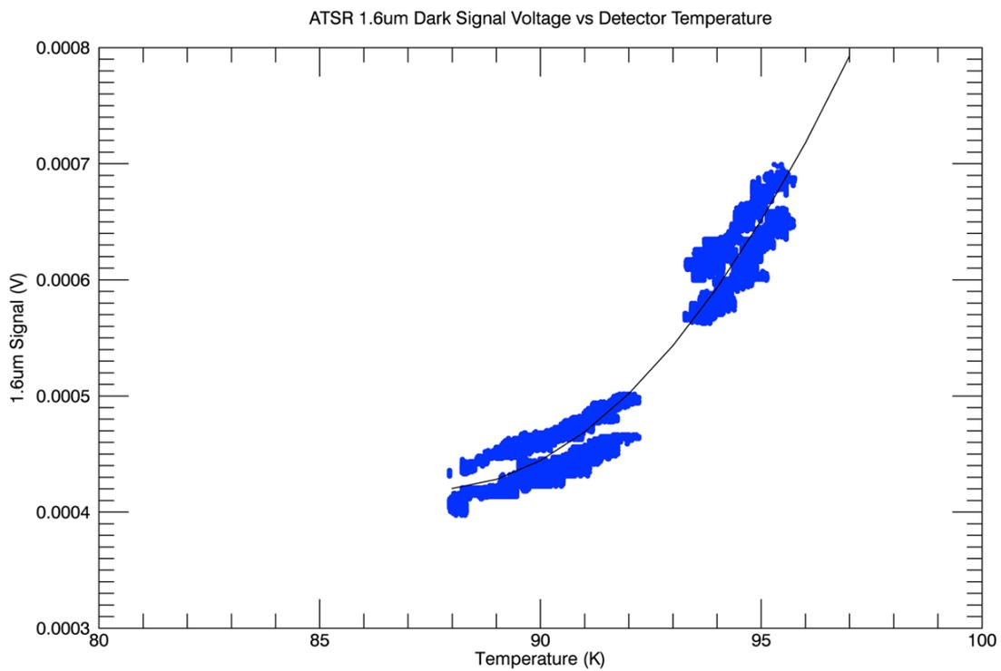
Figure 7: Detector voltage dependence on temperature, from sample 1991 data
