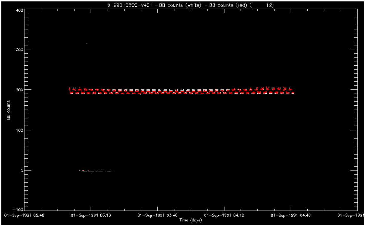
Figure 9: Derived 1.6 $\mu$ m cold blackbody counts (in red) from 01-Sep-1991 (1 orbit). Measured +BB values are shown in white. Processed by v401 development code; all cold blackbody values are derived.
