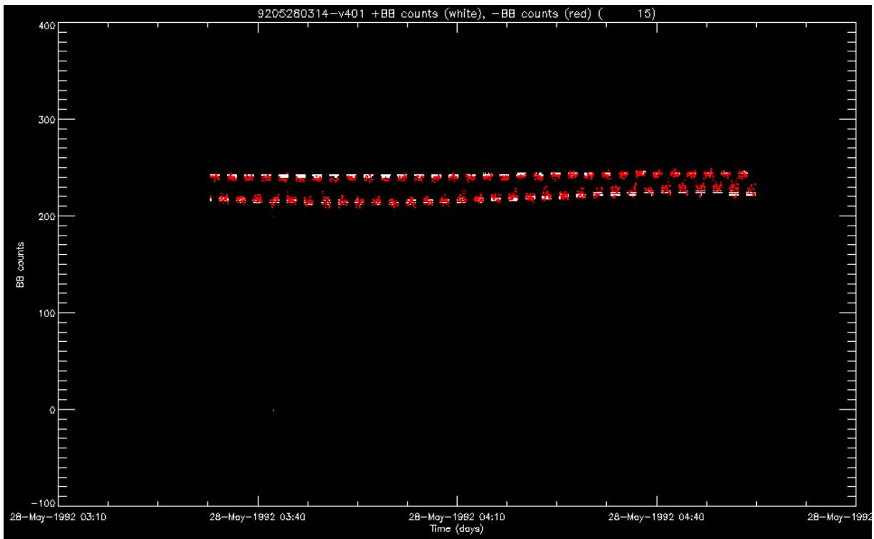
Figure 10: Derived 1.6 $\mu$ m cold blackbody counts (in red) from 28-May-1992 (1 orbit). Measured +BB values are shown in white. Processed by v401 development code; all cold blackbody values are derived.
