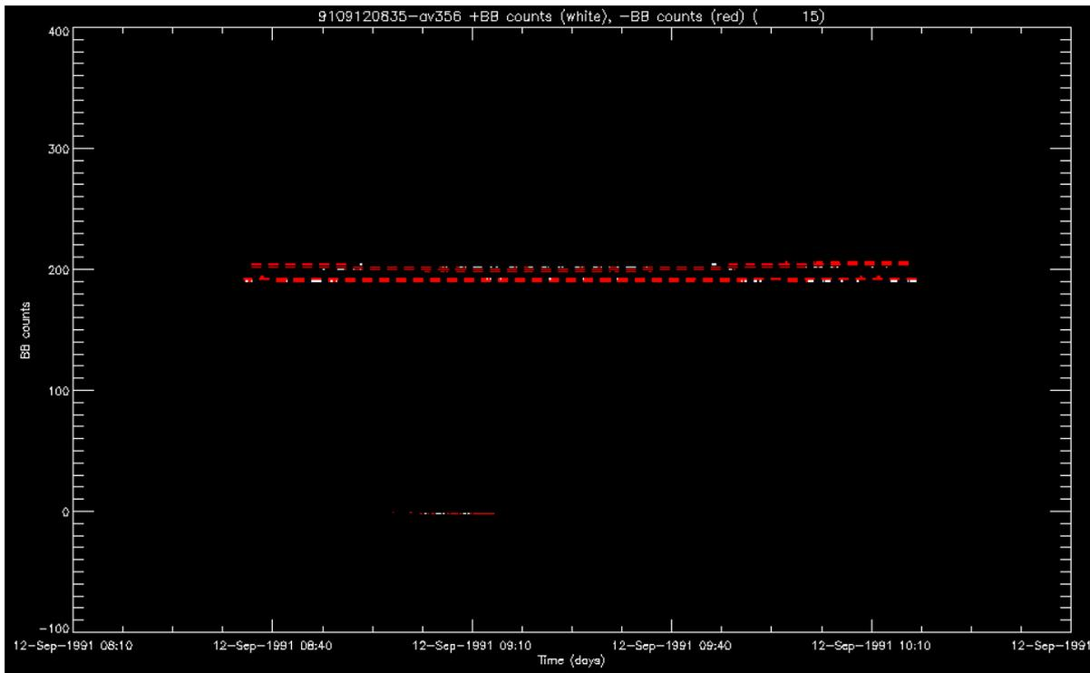
Figure 2: Typical 1.6µm blackbody values from 12-Sep-1991, 1 orbit with ascending node crossing time 08:35UTC.
