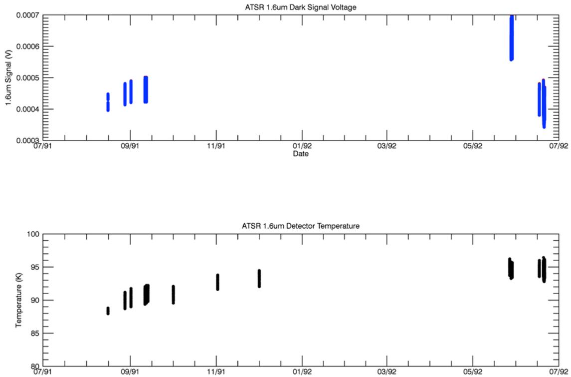
Figure 6: 1.6 $\mu$ m blackbody detector counts from sample days (top panel) and variation with detector temperature
