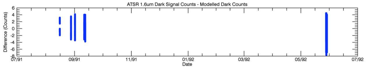
Figure 8: difference between derived and actual 1.6 $\mu$ m blackbody counts for sample days in 1991 and 1992
