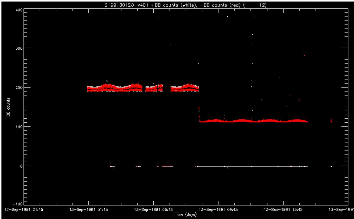
Figure 11: Derived 1.6 $\mu$ m cold blackbody counts (in red) from 13-Sep-1991 (full day). Measured +BB values are shown in white. Processed by v401 development code; all cold blackbody values are derived.
