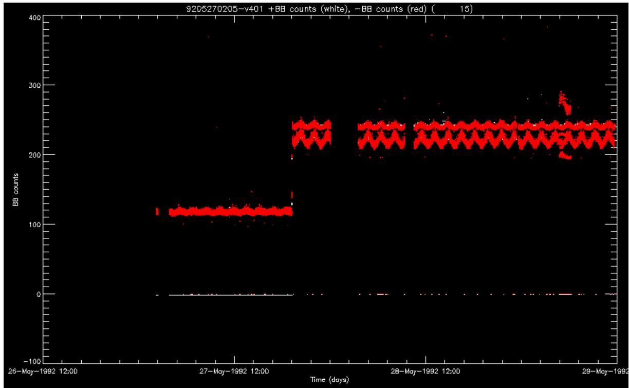
Figure 12: Derived 1.6 $\mu$ m cold blackbody counts (in red) from 27 to 29-May-1992. Measured +BB values are shown in white. Processed by v401 development code; all cold blackbody values are derived.
