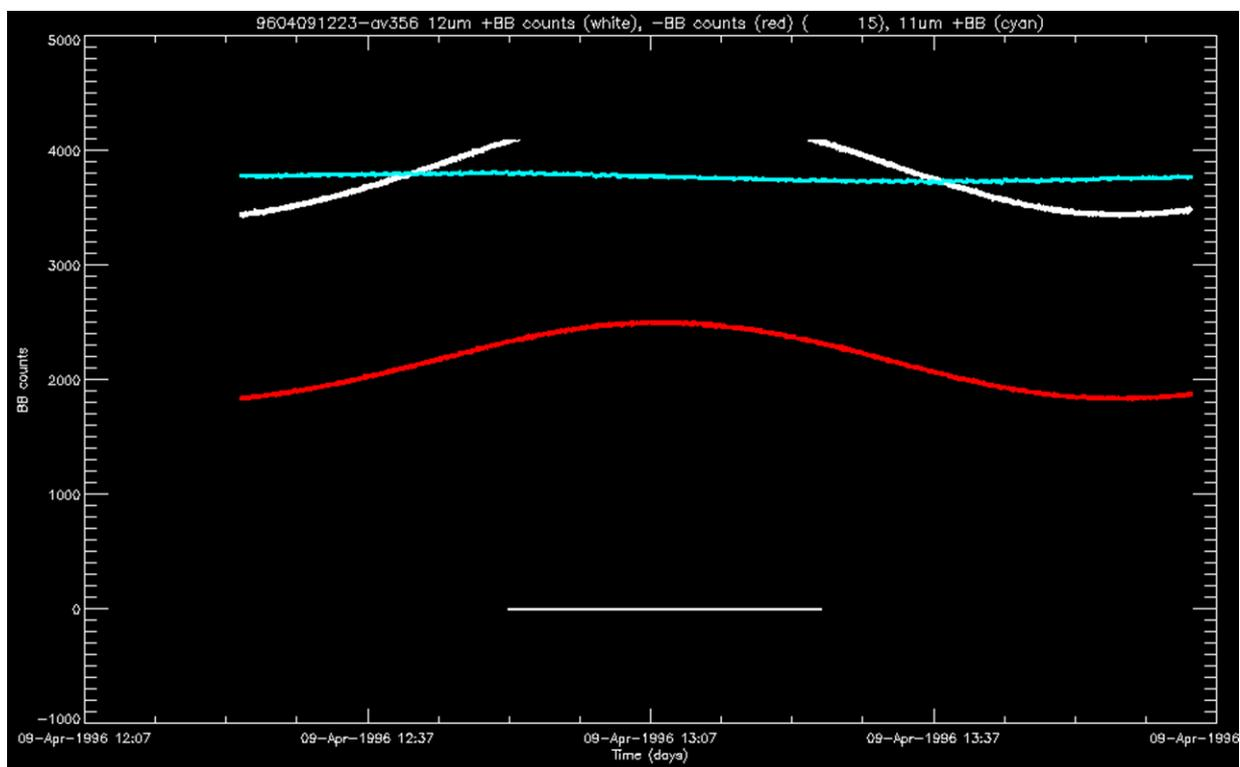
Figure 1: Counts from the 12 $\mu$ m channel warm (white) and cold (red) blackbodies and from the 11 $\mu$ m channel warm blackbody (cyan), for the orbit at 12:23 09-Apr-1996.
