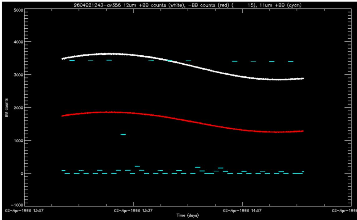
Figure 13: Counts from the 12µm channel warm (white) and cold (red) blackbodies and from the 11µm channel warm blackbody, for the orbit at 02-Apr-1996 12:43.
