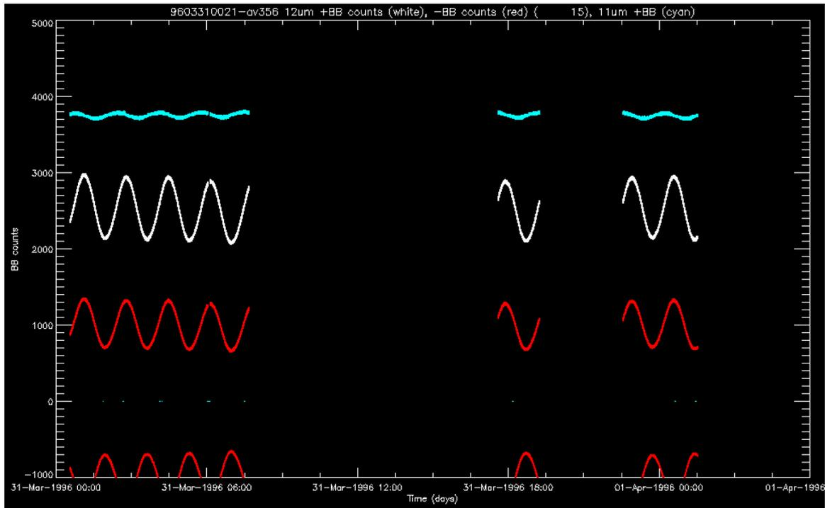
Figure 11: Counts from the 12µm channel warm (white) and cold (red) blackbodies and from the 11µm channel warm blackbody, for several orbits on 1996-03-31
