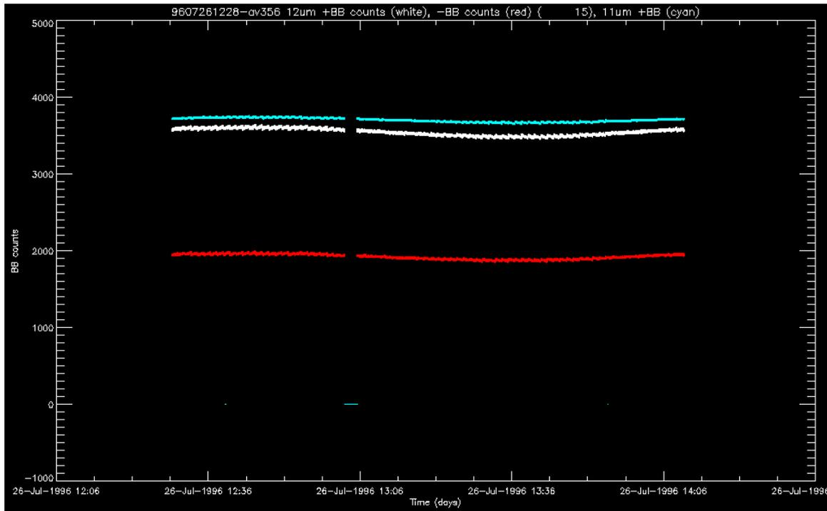
Figure 19: Counts from the 12µm channel warm (white) and cold (red) blackbodies and from the 11µm channel warm blackbody, for the orbit at 12:28 26-Jul-1996.
