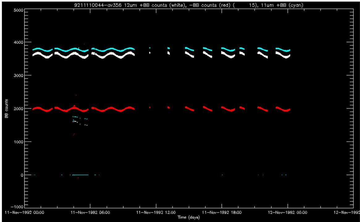
Figure 6: Counts from the 12µm channel warm (white) and cold (red) blackbodies and from the 11µm channel warm blackbody, for all available UBT files on 11-Nov-1992
