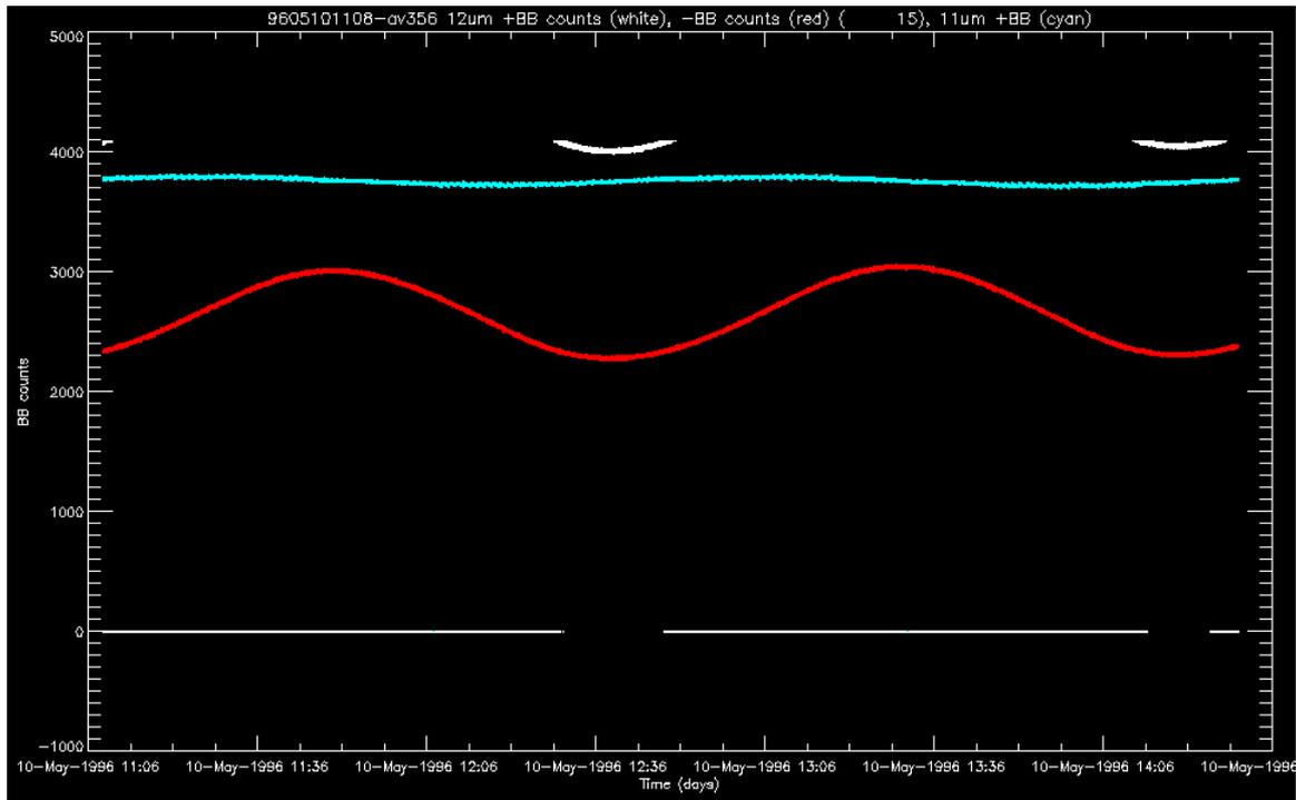
Figure 16: Counts from the 12µm channel warm (white) and cold (red) blackbodies and from the 11µm channel warm blackbody, for the 2 orbits at 11:08 10-May-1996
