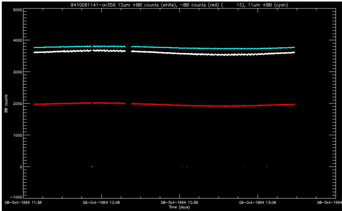
Figure 9: Counts from the 12µm channel warm (white) and cold (red) blackbodies and from the 11µm channel warm blackbody, for the orbit at 11:41 08-Oct-1994
