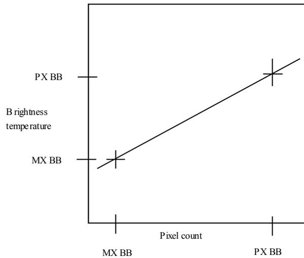
Diagrammatic representation of the linear calibration of pixel counts to brightness temperature
