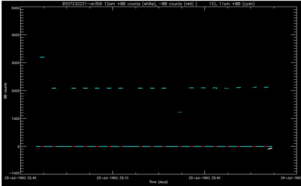
Figure 4: Blackbody counts from the 12µm channel warm (white) and cold (red) blackbodies and from the 11µm channel warm blackbody, for the orbit from 23-Jul-1992 22:21
