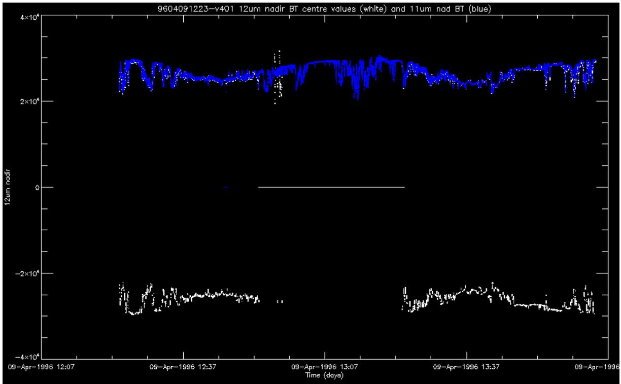
Figure 21: Centre of scan brightness temperatures for the 12µm and 11µm channels, from the updated SUPPLE processor.
