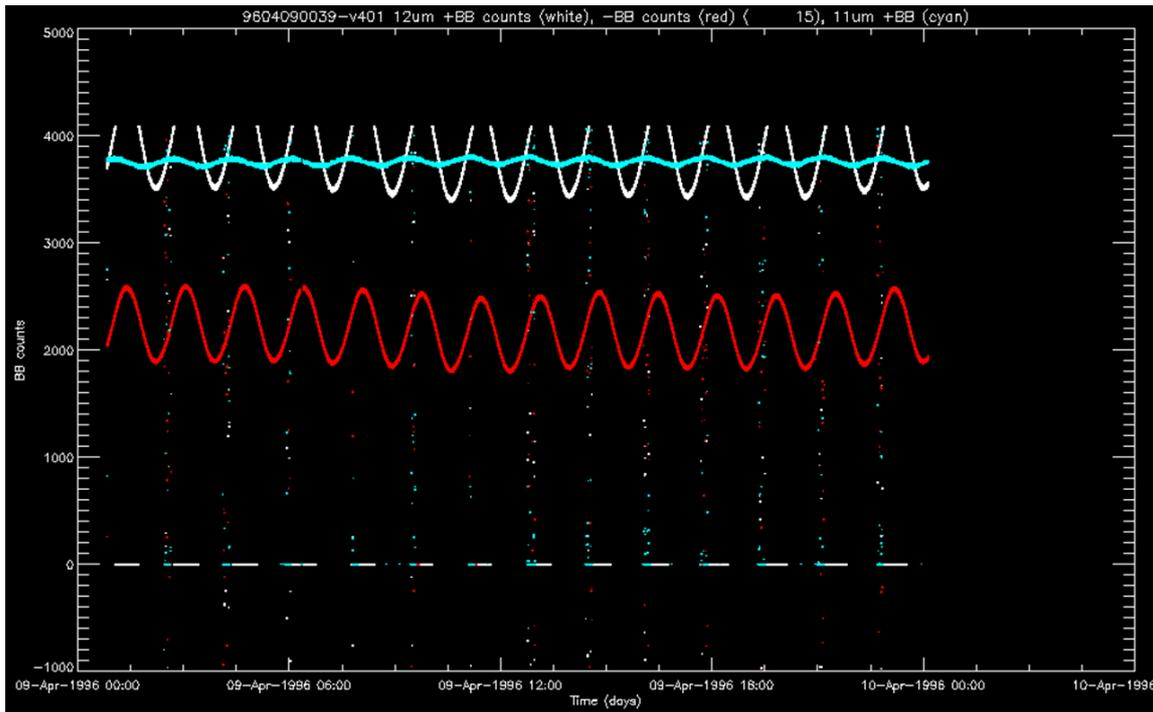
Figure 12: Blackbody values from the full day's data for 09-Apr-1996, showing the extent of blackbody saturation. (Same colours as Figure 1, 12µm warm blackbody counts are shown in white)
