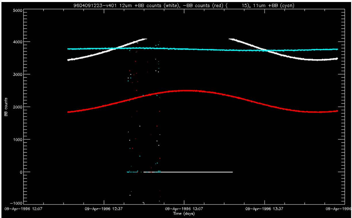
Figure 22: Blackbody counts for the orbit with ascending node time 09-Apr-1996 12:23, from the updated SUPPLE processor.
