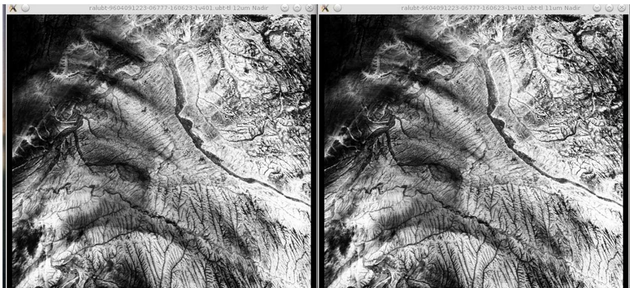
Figure 24: 12µm (left) and 11µm (right) nadir brightness temperatures from reprocessed data for orbit with ascending node time 09-Apr-1996 12:23, scene at along-track distance 06777, acquisition time 12:40:08.
