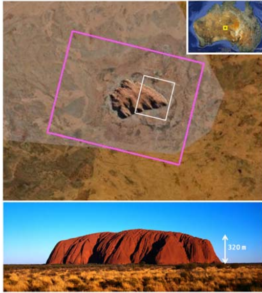
Figure 1. Ayers Rock test site. The footprint of the SAR acquisition is shown in magenta, superimposed over an optical image extracted from Google-Earth. The white borders enclose the area selected for the experiment. The bottom picture reports the estimated height of the plateau.
