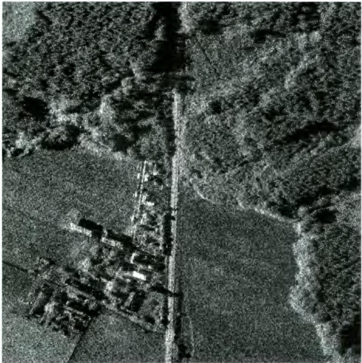
Figure 2. AeS-1 image of Weichselbaum in Germany. Image parameters as Fig. 1. Number of looks: 1, resolution: 2 x 2 m. One can see the rails of the train (vertical lines), the houses of the village and the differentiation between coniferous and pine forest.
