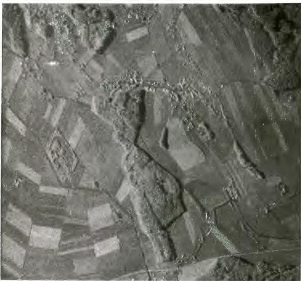
Figure 3. AeS-1 image of Solothurn in Switzerland. Image parameters: flight date: 11.9.96, flight velocity: 54.5 m/s, flight height: 11.000 feet, drift: -0.8 °, azimuth bandwidth: 200 Hz, range bandwidth: 400 Mhz, PRF: 8 kHz, transmitting frequency: 9.6 GHz, number of looks: 8, resolution: 2 x 2 m.
