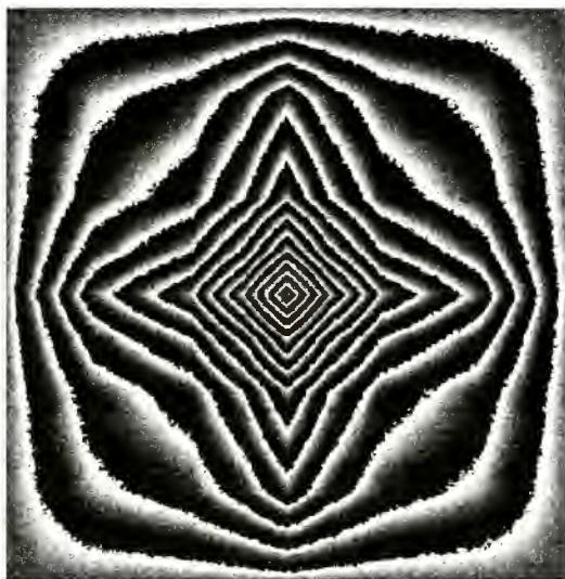
Figure 4 - Interferogram with  $\gamma = 0.9$
