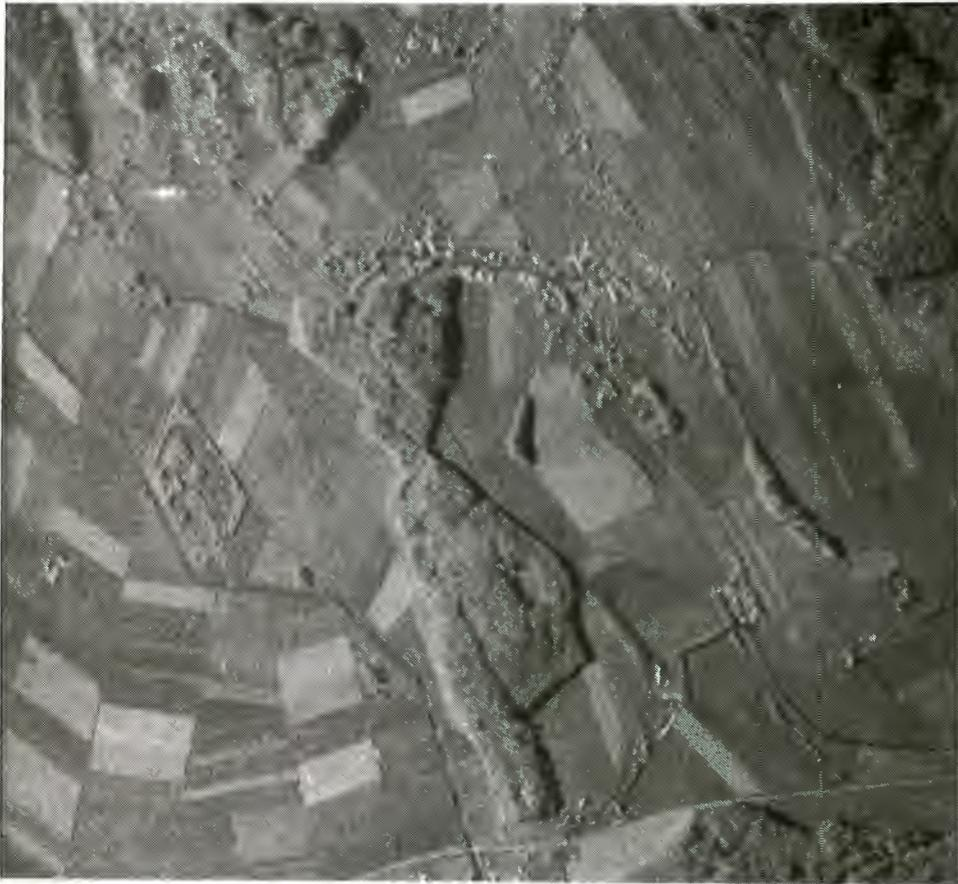
Figure 3. AeS-1 image of Solothurn in Switzerland. Image parameters: flight date: 11.9.96, flight velocity: 54.5 m/s, flight height: 11.000 feet, drift:  $-0.8^\circ$ , azimuth bandwidth: 200 Hz, range bandwidth: 400 Mhz, PRF: 8 kHz, transmitting frequency: 9.6 GHz, number of looks: 8, resolution: 2 x 2 m.
