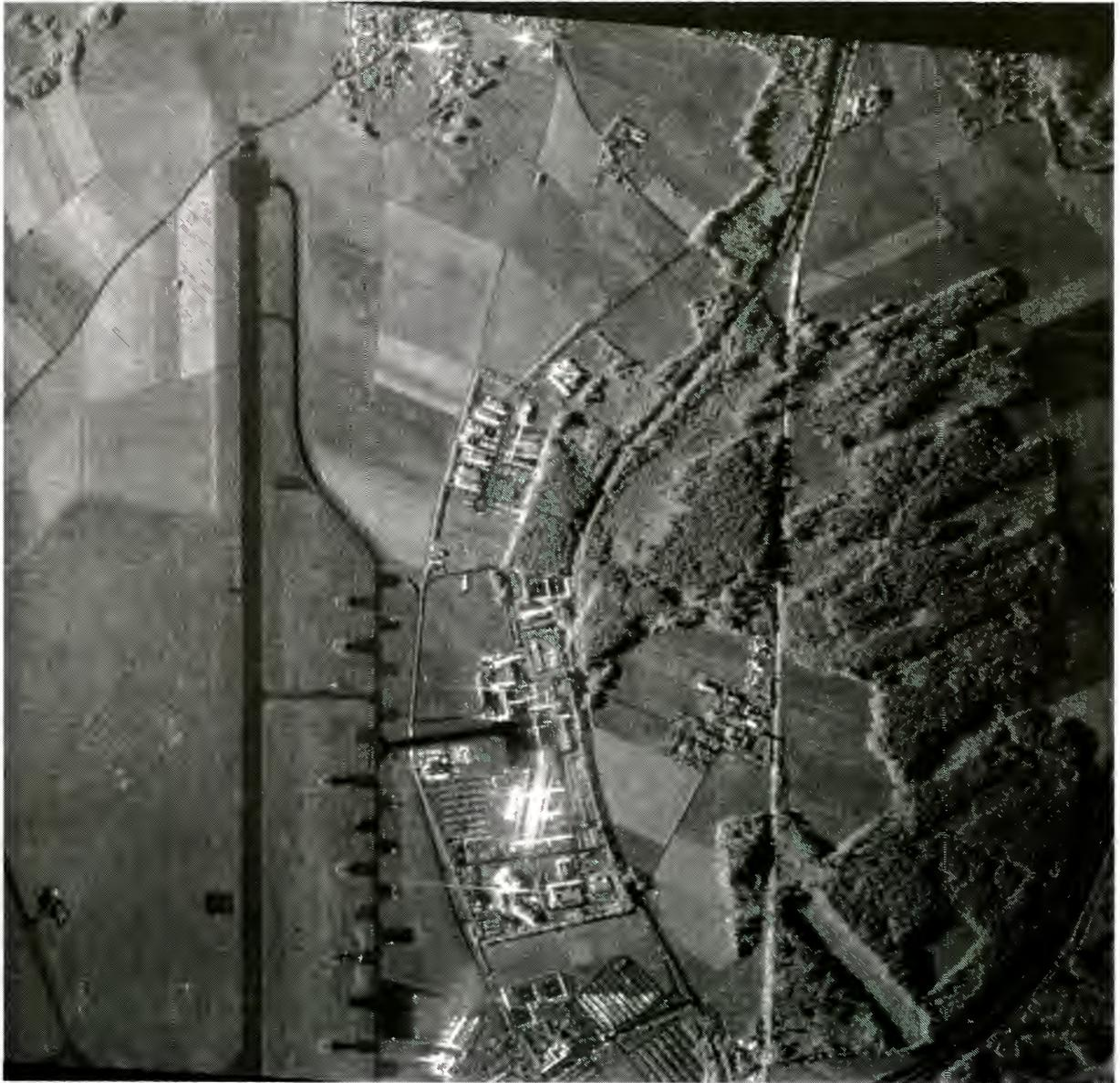
Figure 1. AeS-1 image over the Oberpfaffenhofen area in Germany. Image parameters: flight date: 6.9.96, flight velocity: 70.5 m/s, flight height: 11.000 feet, drift: -5.6 °, azimuth bandwidth: 200 Hz, range bandwidth: 400 Mhz, PRF: 8 kHz, transmitting frequency: 9.6 Ghz, number of looks: 48, resolution: 2 x 2 m.
