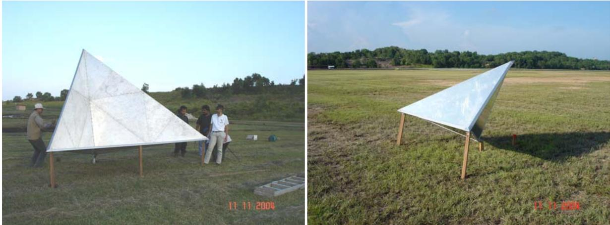
Figure 5.2.4: left: Corner reflector of the size 3m for P-band. Right: Corner reflector of the size 1.5m for X-, C-, and L-band. Both positioned along the runway
