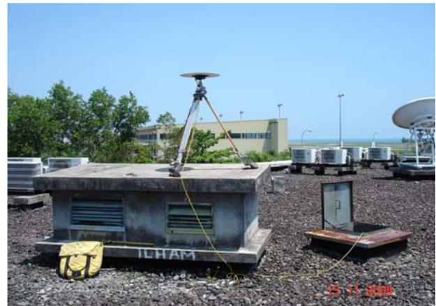
Fig. 5.2.5. Differential GPS installed on the airport building above a reference point.
