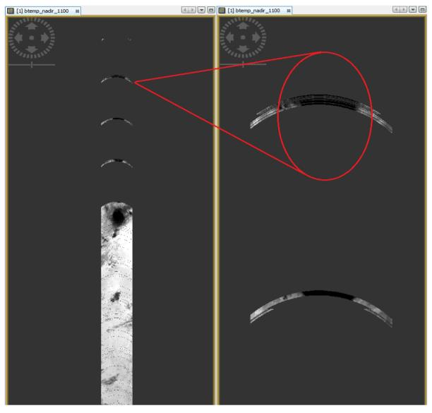
Figure 2 ATSR-2 v3.0.1 (post-June 2003): The fragmented nature of data included in products from this period. Product: AT2\_TOA\_1PURAL20060807\_052205\_000000001118\_00090\_59062\_0000.E2 (nadir view, 11 μm channel).
