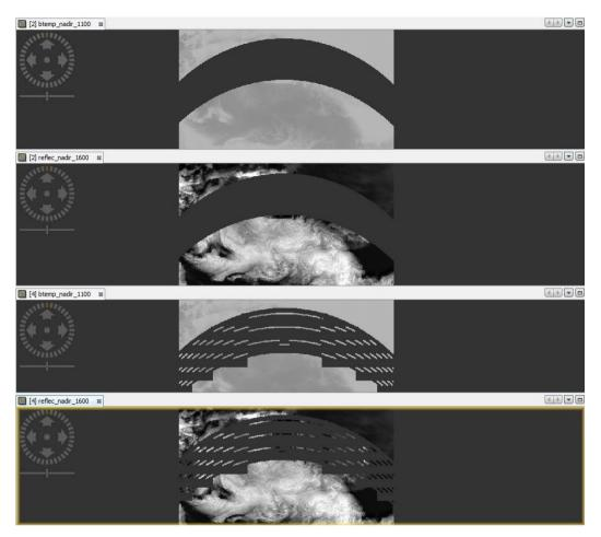
Figure 1 ATSR v3.0.1: Implementation of processing bug fix - data gap present in nadir (1.6 and 11 µm channels), comparison between v3.0.1 (top 2 images) and v3.0 (bottom 2 images). Product:
