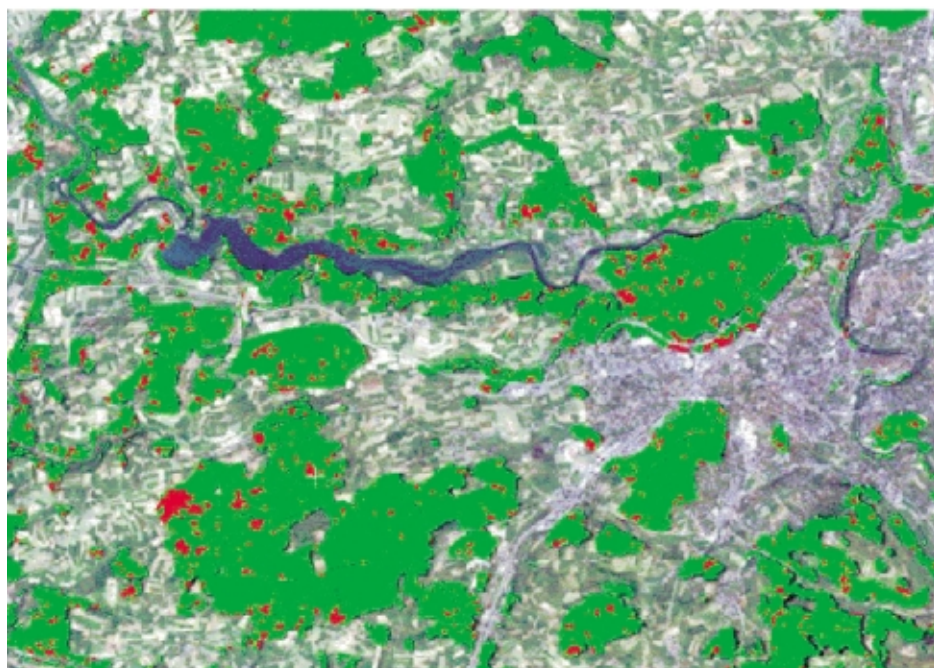
Figure 9. Storm-damage map of Switzerland, from winter 1999/2000, derived from ERS SAR tandem coherence combined with a Landsat TM image as background. Forested areas are in green and damaged forest areas are in red (courtesy of Gamma Remote Sensing, Spot Image, Swiss Federal Institute of Technology Zurich, and SERTIT)
