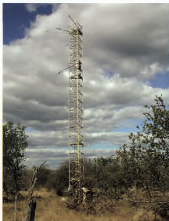
Flux tower for in-situ carbon-dioxide measurements
