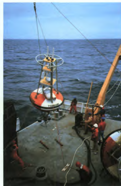
Deployment of a tsunami measuring buoy in the Pacific Ocean
