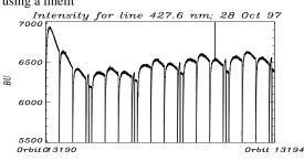
*Figure 3.* intensity (line 427.6 nm) of all products in monthly calibration mode of 5 orbits 28/10/1997, no data filtering
