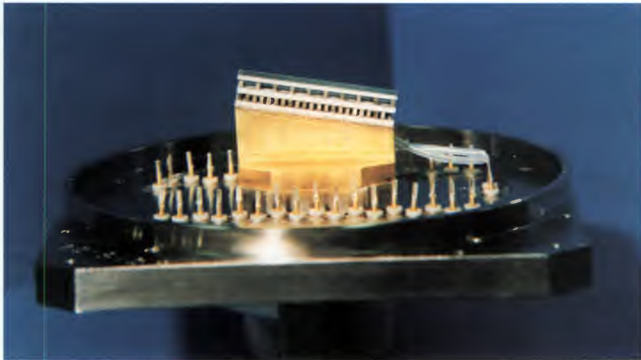
Figure 4.3-3 Side view of pin plate with Peltier element
