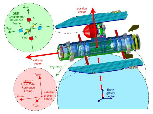
Figure 8 - Trajectory and reference frames.
