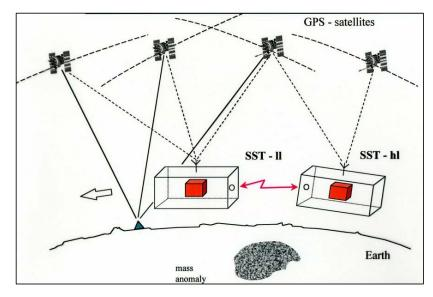
Figure 13 - GRACE - Concept of inter-satellite link (SST-ll) coupled with SST-hl.
