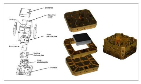
Figure 7 - Schematic and actual views of one accelerometer.
