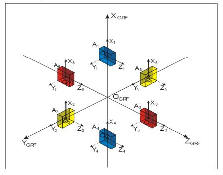
Figure 20 - EGG Accelerometers Configuration.
