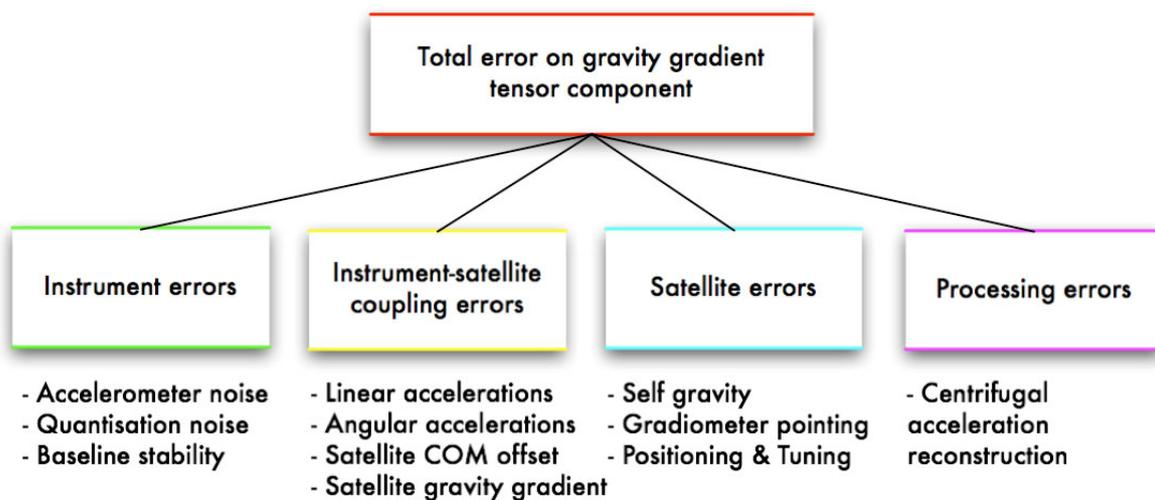
**Figure 4.** Gravity gradiometry error budget overview.
