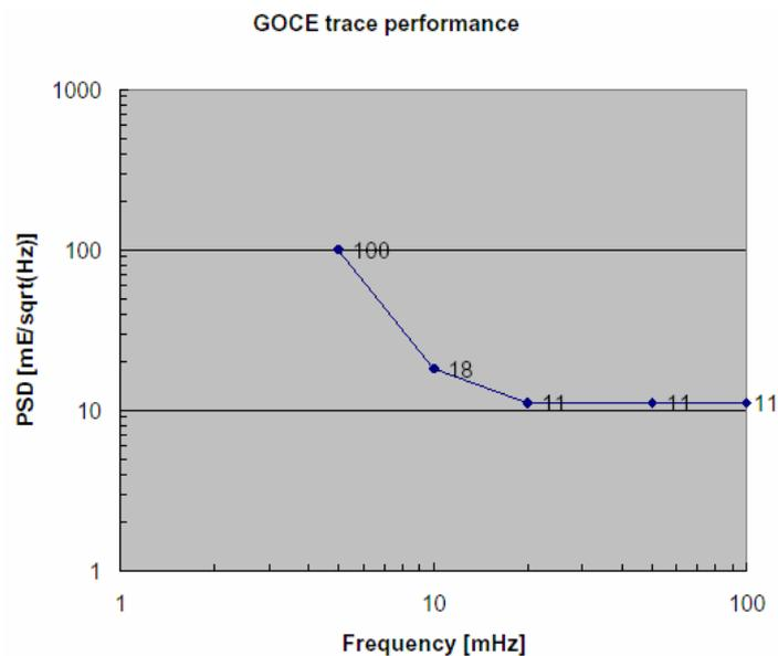
**Figure 6.** The blue curve indicates the trace requirement, based on the yaw-piloting, mode during science measurements ([RD8](#)).
