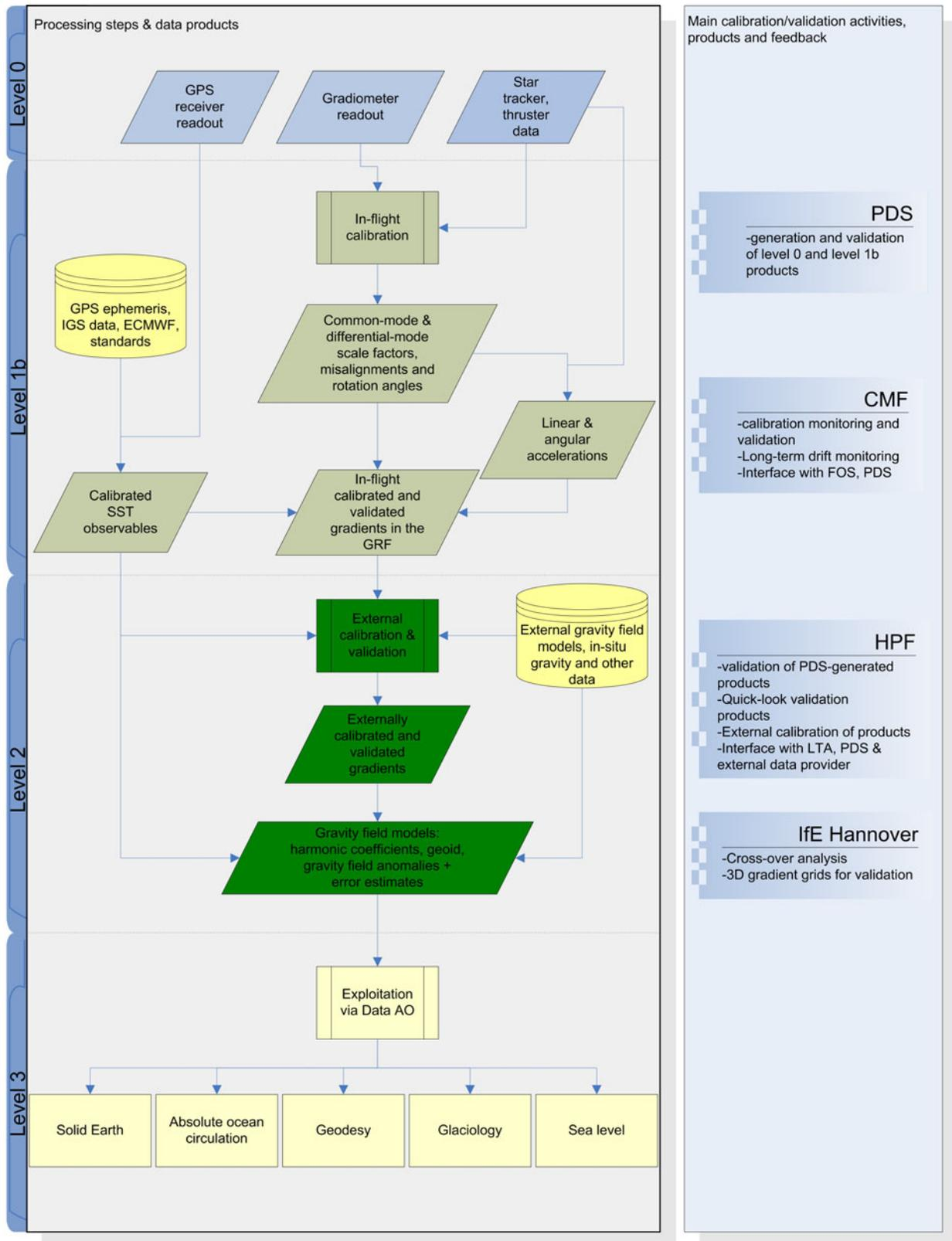
**Figure 9.** Schematic description of data processing steps, products and product flows, together with calibration and validation activities within the Ground Segment and the respective contributions from approved Cal/Val AO Project activities.
