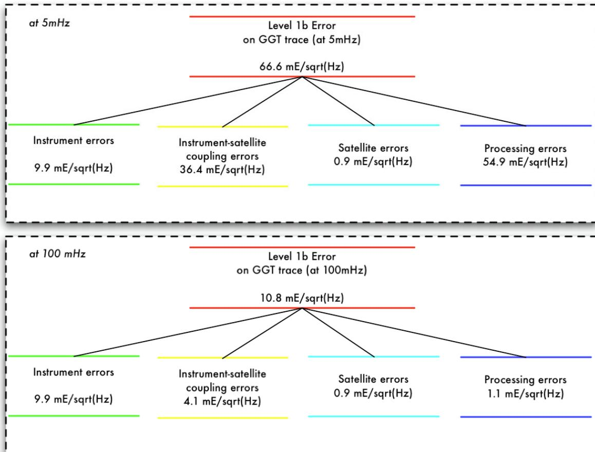
**Figure 5.** Level 1b gradiometry error budget.
