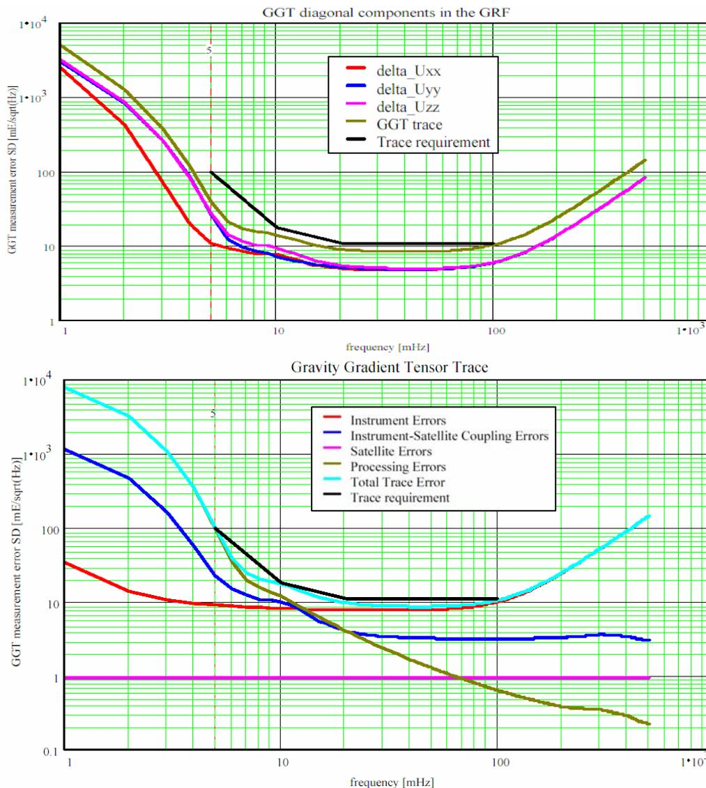
**Figure 7.** Individual contributions to the predicted total Gravity Gradient Trace (GGT) error, based on GOCE system simulations.
