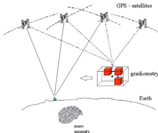
**Figure 2.** Schematic illustration of the combined satellite gravity gradiometer (SGG) and satellite-to-satellite (high-low) tracking mission concept.
