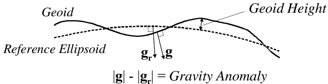
**Figure 1.** Definition of geoid height and gravity anomaly.
