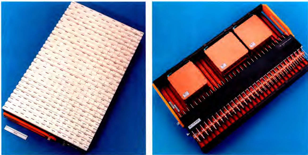
Fig. 3.85 (left): DESA mock-up in front side view (DSS) Fig. 3.86 (right): DESA panel feed network (DSS)
