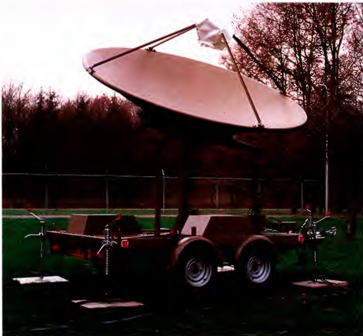
Fig. 3.42. The trailer mounted RAPIDS with 2.7 metre dish for data capture through a 90 degree pass (NRI)
