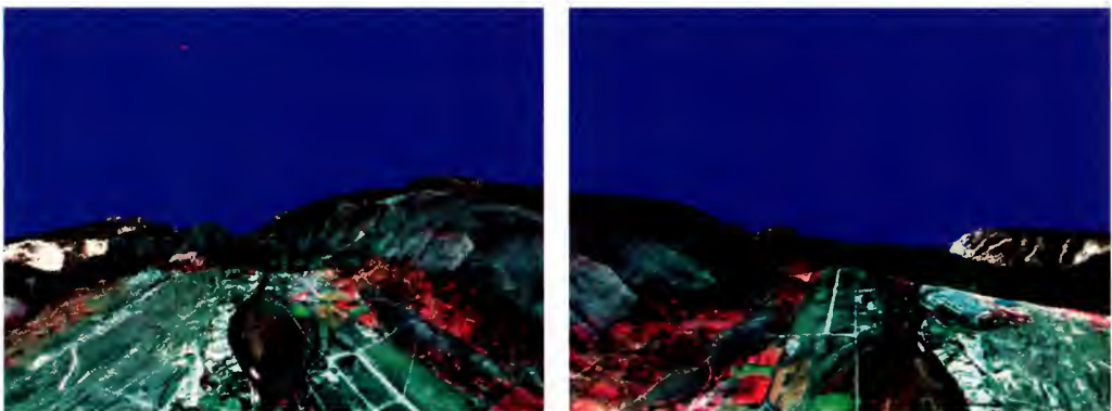
Fig. 3.40: 3-D visualisations of fused image using DEM from ERS Tandem Mission (C Pohl and J Valero, WEU Satellite Centre)
