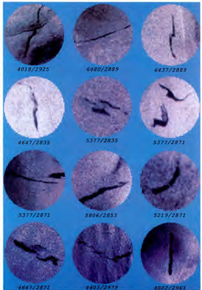
Fig. 3.63: Typical shapes of detected spills on the corresponding ERS-1 SAR orbits and frames (National Centre for Marine Research, Institute of Oceanography, Greece)
