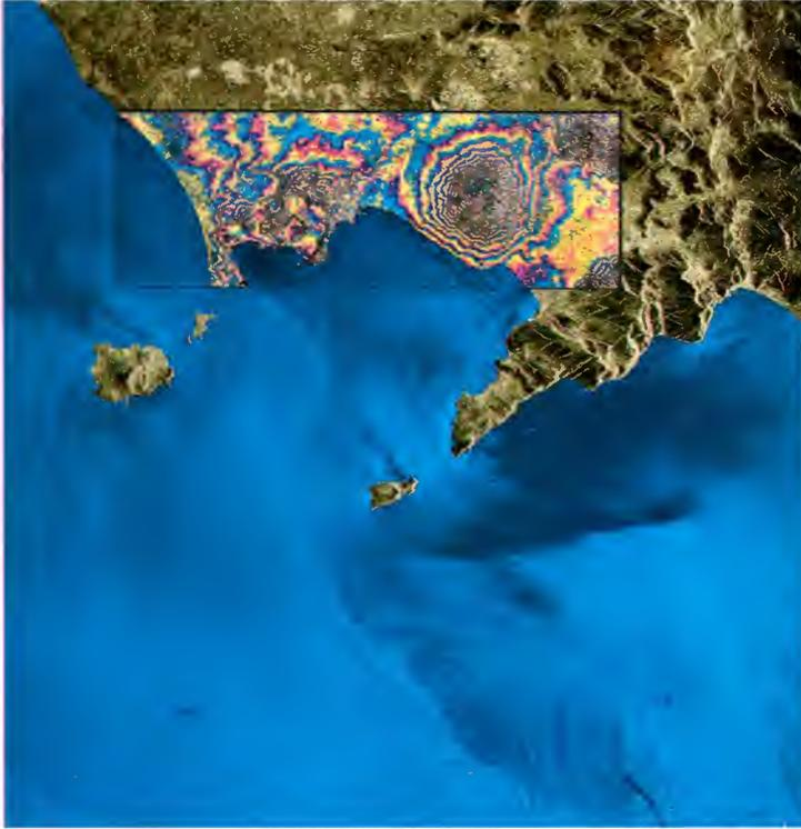
An exciting and promising technique for using ERS-1 data is synthetic aperture radar interferometry. Using interferometry, it is possible to produce detailed three-dimensional relief maps of the Earth's surface with an accuracy of a few metres, direct from ERS-1 data.
