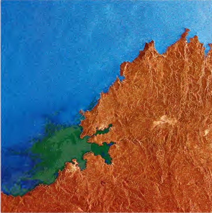
Because oil has a restraining effect on waves – "pouring oil on troubled waters" – the backscattering of radar, which depends on the roughness of the sea surface, reflects this phenomenon. Very large oil spills, like this one from the wreckage of the tanker Aegean Sea near La Coruña in Northern Spain on 3 December 1992, provide spectacular examples of the capabilities of ERS-1.
