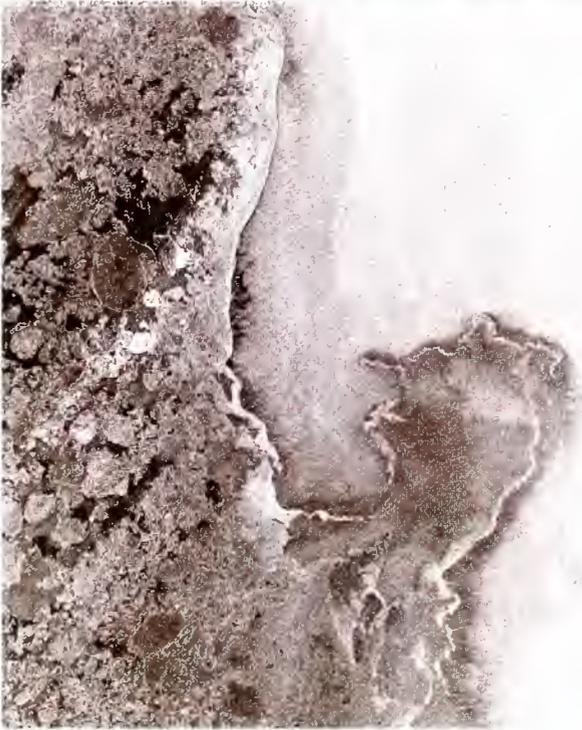
Various different types of ice stand out clearly on ERS-1 images in open water. Accurate ice maps can therefore be made from the images and transmitted to ships via telecommunications satellites to guide them safely through ice-infested waters.
