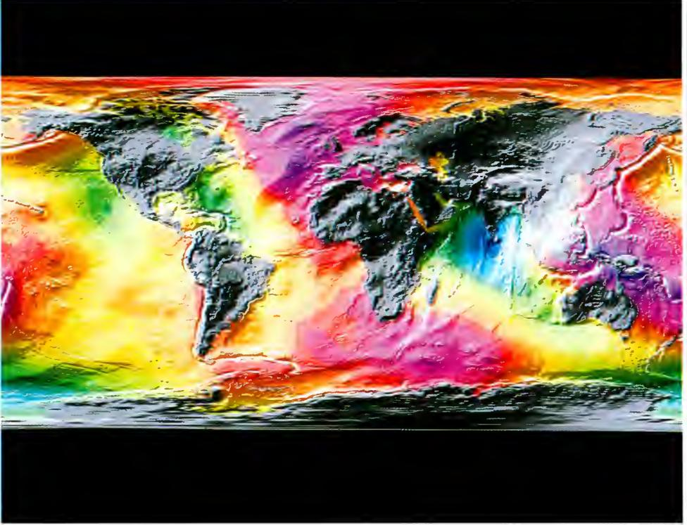
ERS-1's vision is not only global, it is also different from that of the human eye. This world map of the mean sea level was obtained on the basis of one year's measurements by the ERS-1 radar altimeter. This instrument determines, with great accuracy, the distance between the satellite and the surface of the Earth.
