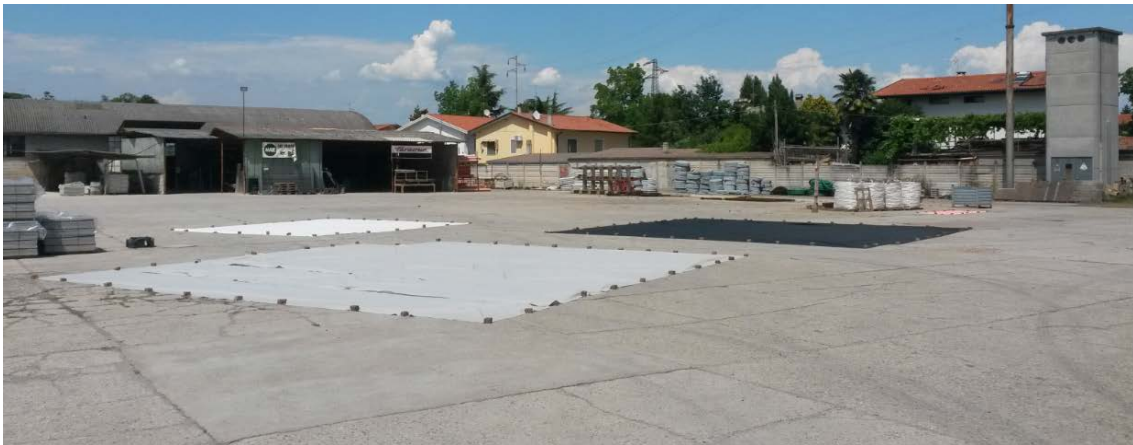
Figure 18: Artificial calibration/validation targets for ground reference measurements.
