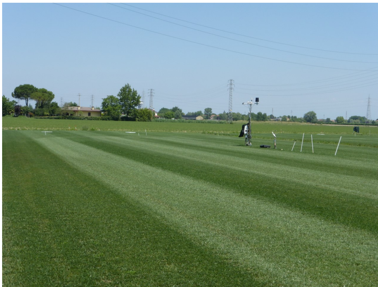
Figure 22: View of one of the two flux towers installed in Latisana (Italy) that operated throughout the field campaign.
