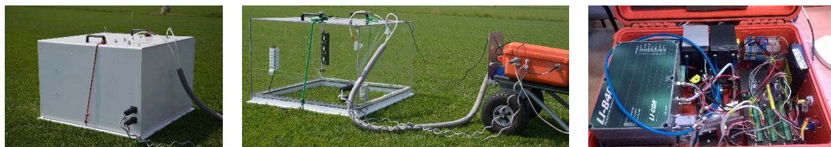
Figure 23: Closed, dynamic-chamber system used for measurements of CO 2 fluxes.
