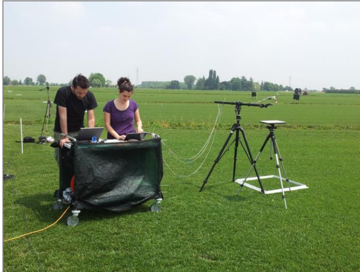
Figure 21: Experimental setup used to collect high-resolution spectral measurements over the grassland plots.
