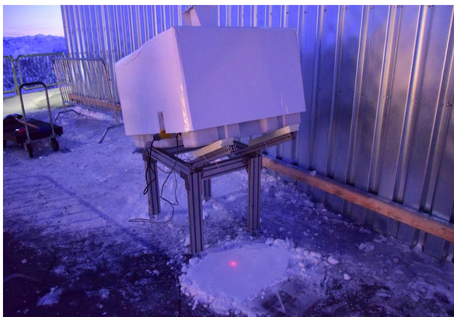
Figure 30 FIRMOS during snow test measurements. The bright red spot in the centre of the FOV is due to the alignment laser
