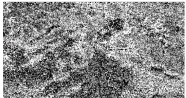
Figure 9. Differential interferogram of image pair of 28/12/2010 – 13/01/2011 with B_n = -446m . (Potenza area)
