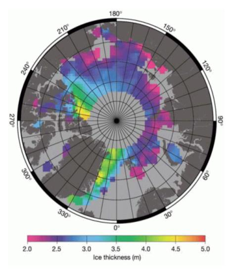
Figure 7: Sea-Ice Thickness derived from Radar Altimeter data
