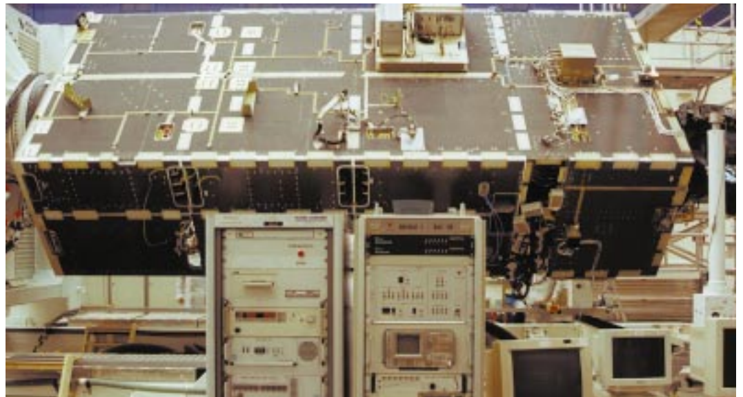
Engineering Model of Polar Platform Payload Module in integration at MMS(B) (GOMOS BB Integrated, RA-2 IEGSE in foreground) (Photo courtesy of MMS(B) )
