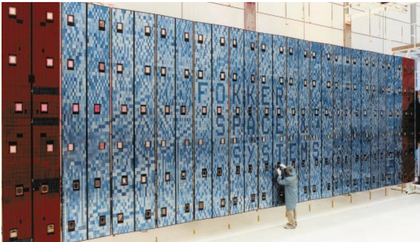
The Development Model of the Solar Array (fully deployed configuration) (Photo courtesy of Fokker)
