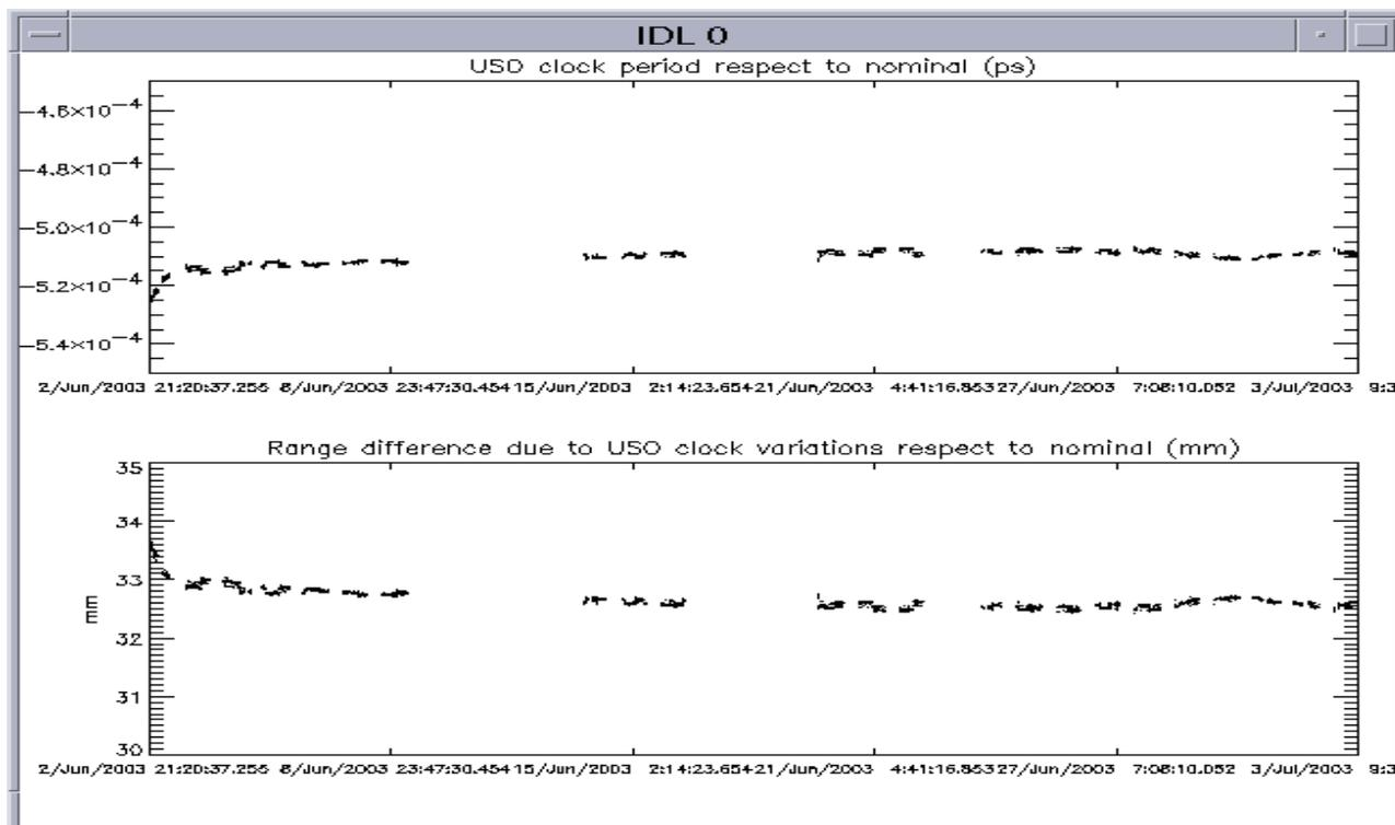
Figure 2: USO clock period and Range difference obtained with the IDL tool over the period 2<sup>nd</sup> June to 7<sup>th</sup> July 2003.
