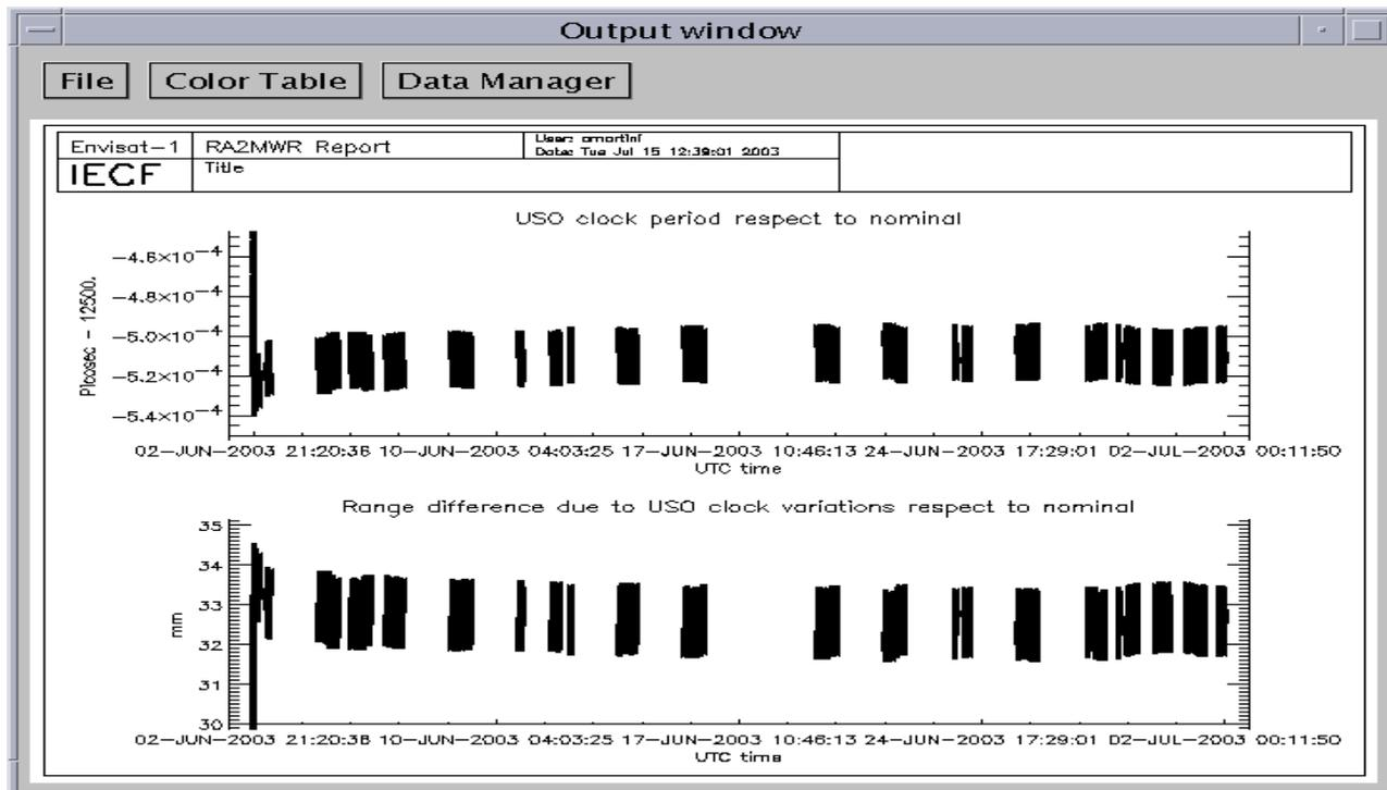
Figure 1: USO clock period and Range difference obtained with the IECF tool over the period 2<sup>nd</sup> June to 7<sup>th</sup> July 2003.
