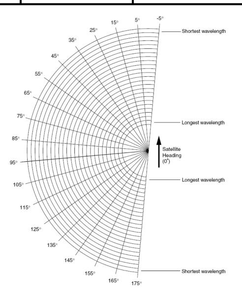
Figure 8.5.5.4.4-1 Wave Mode Cross Spectra Format
