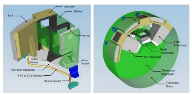
Figure 4.2: Telescope and Fixed Optics Assembly
