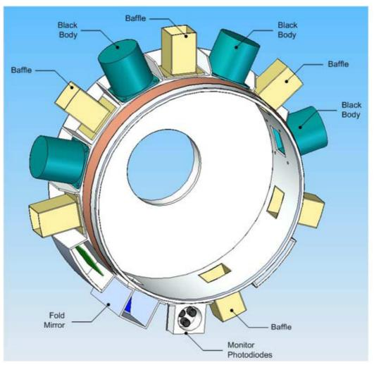
Figure 4.7: Calibration Drum Layout
