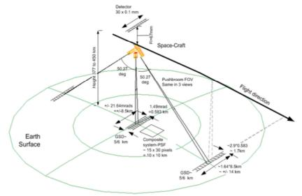
Figure 4.4: Viewing geometry
