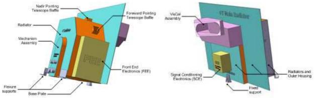
Figure 4.3: External Configuration of Optics Unit (two views)
