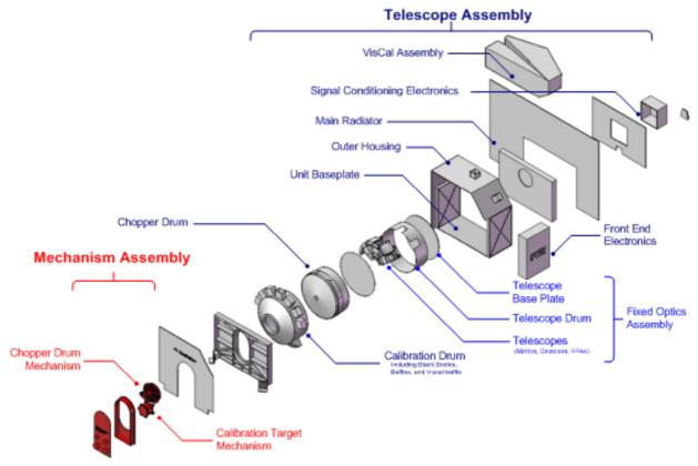
Figure 4.1: BBR Optics Unit Exploded View
