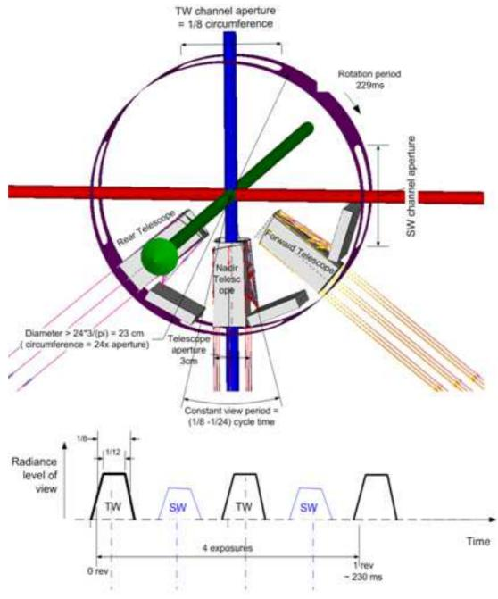
Figure 4.5: Chopper and chopper operation
