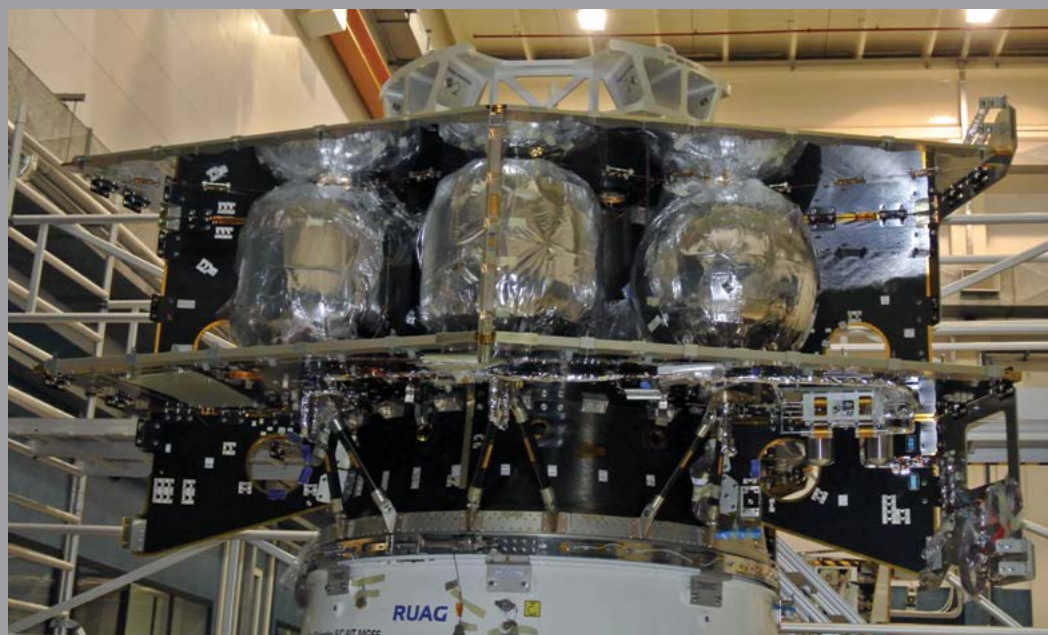
BepiColombo Mercury Transfer Module during system integration and test (Thales Alenia Space Italy)
