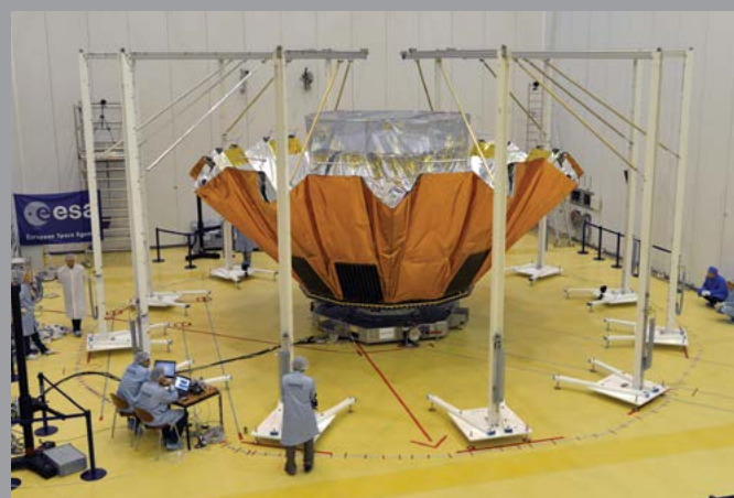
The Gaia spacecraft after last deployment test of the sunshield
