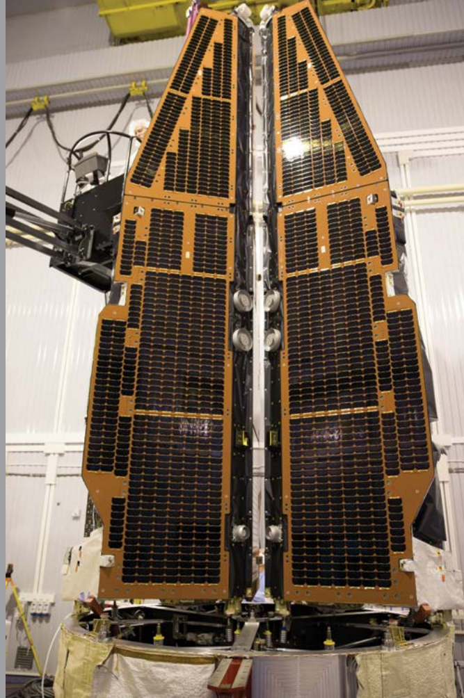
Seen on 8 November, only days before launch, the three Swarm satellites sit just centimetres apart on their tailor-made launch adapter. This novel system keeps the satellites upright within the fairing during launch and allows them to be injected simultaneously into orbit
