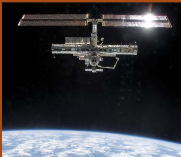
First truss sections added in 2002, this image after the third segment added by STS-113
