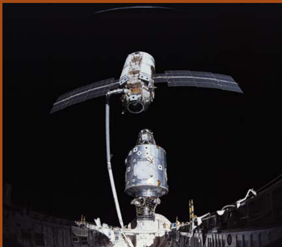
STS-88, the first Space Shuttle mission to the ISS, joining Russian Zarya and US Unity modules
