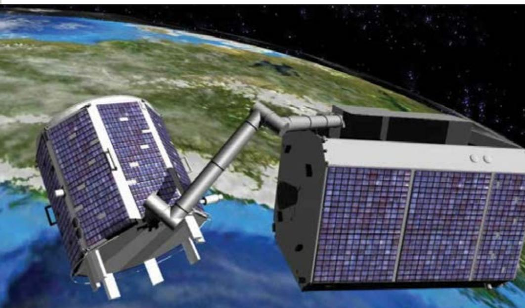
← The proposed German 'Deutsche Orbital Servicing' (DEOS) twin-satellite mission to demonstrate new technologies for the maintenance and disposal of satellites (DLR)
