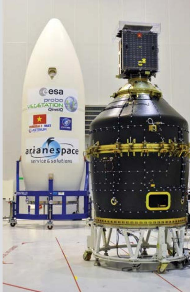
Proba-V on the Vespa payload adaptor, with Vega fairing in background
