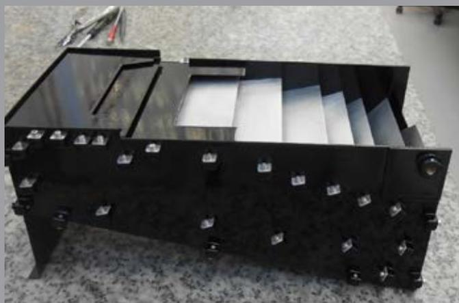
Solar Orbiter SoloHI instrument Baffle Assembly
