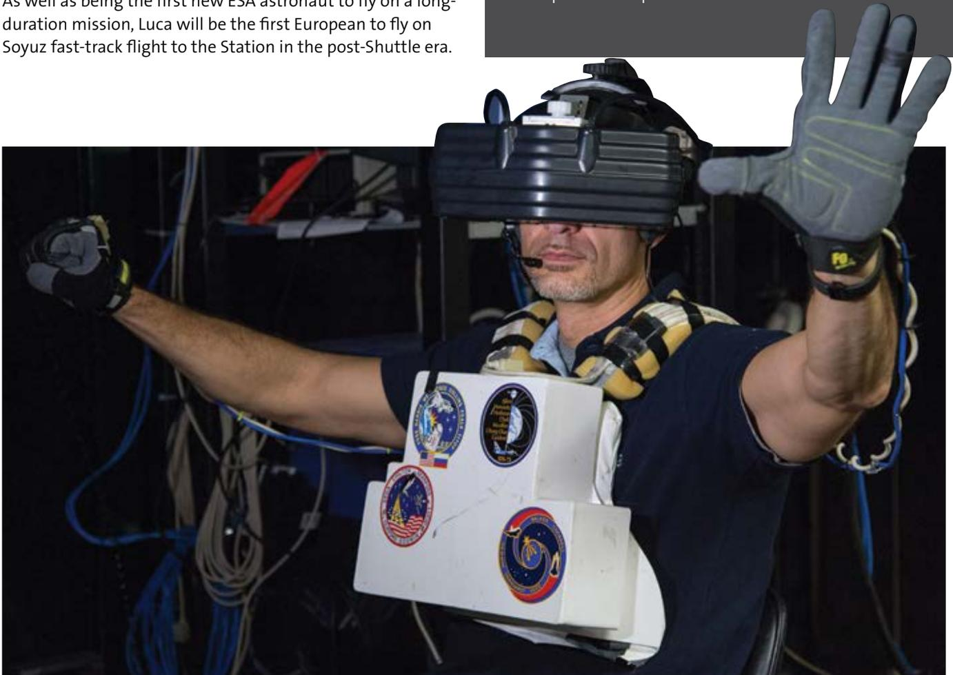
↑ Luca uses virtual reality hardware in the Space Vehicle Mock-up Facility at NASA's Johnson Space Center to rehearse some of his operations on the ISS (NASA)
