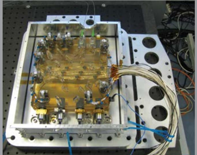
Mounted on its vibration adaptor, the LISA Pathfinder optical bench flight model developed by the Universities of Glasgow and Birmingham and Mullard Space Science Laboratory (UK)
