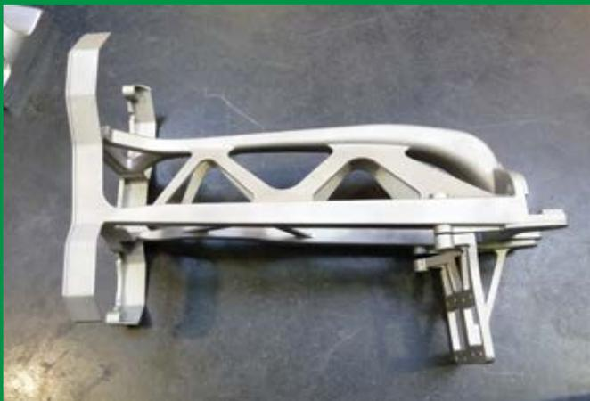
← An alloy antenna support produced in a 3D printing process
