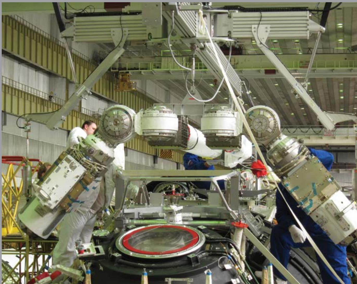
The European Robotic Arm being installed on the Russian Multipurpose Laboratory Module (Khrunichev)
