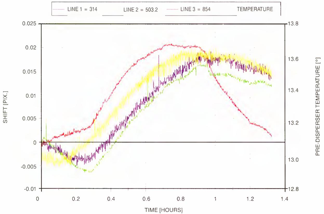
Figure 4. Wavelength shift as a function of orbital temperature variations. The plot shows the relative shifts of three selected lines of the wavelength calibration lamp, in fractions of a detector pixel. One pixel in channel 1 corresponds to 0.1 nm. Also shown is the temperature at the disperser prism, as the most temperature-sensitive optical element (yellow curve)
