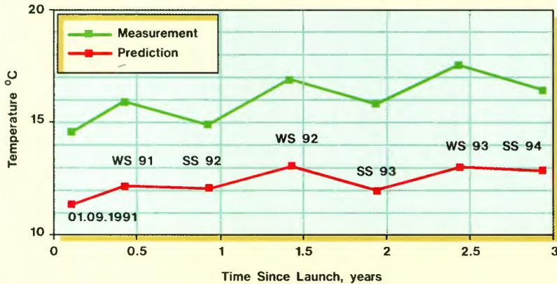
Figure 5. Average payload temperature as a function of lifetime
