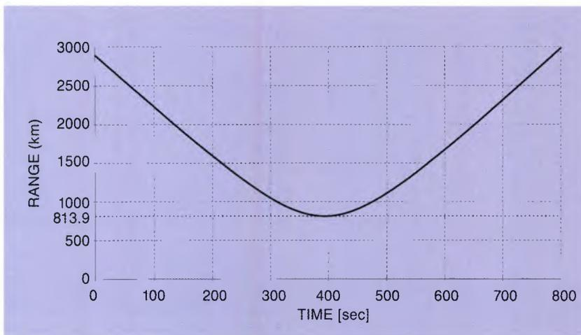
Figure 2. Typical range variation during ground-station contact
