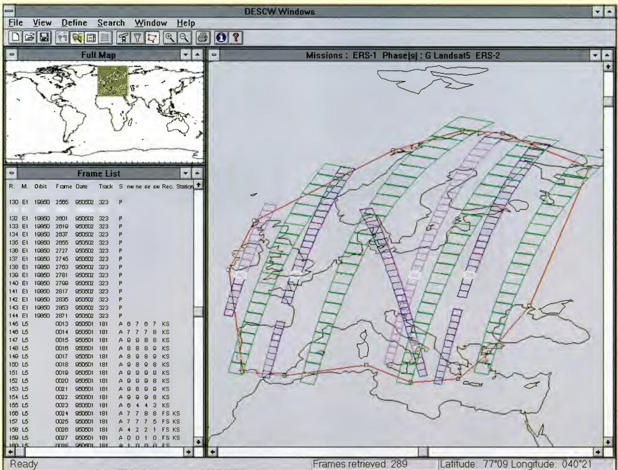
the 'Display ERS-1 SAR Coverage' (DESC) software package. That tool supports the users in defining their requirements for products and services.
