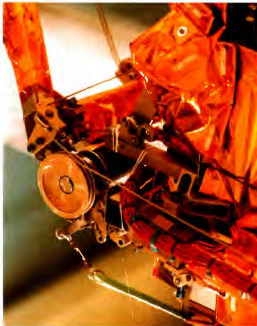
Figure 8b. One of the spring drives for solar-array deployment
