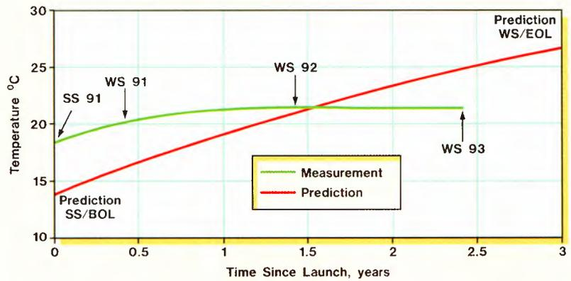
Figure 3. Evolution in the spacecraft platform's average temperature as a function of lifetime
