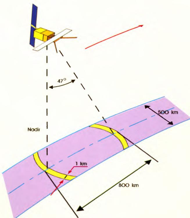
Figure 17. Measurement principle of the Along-Track Scanning Radiometer (ATSR)
