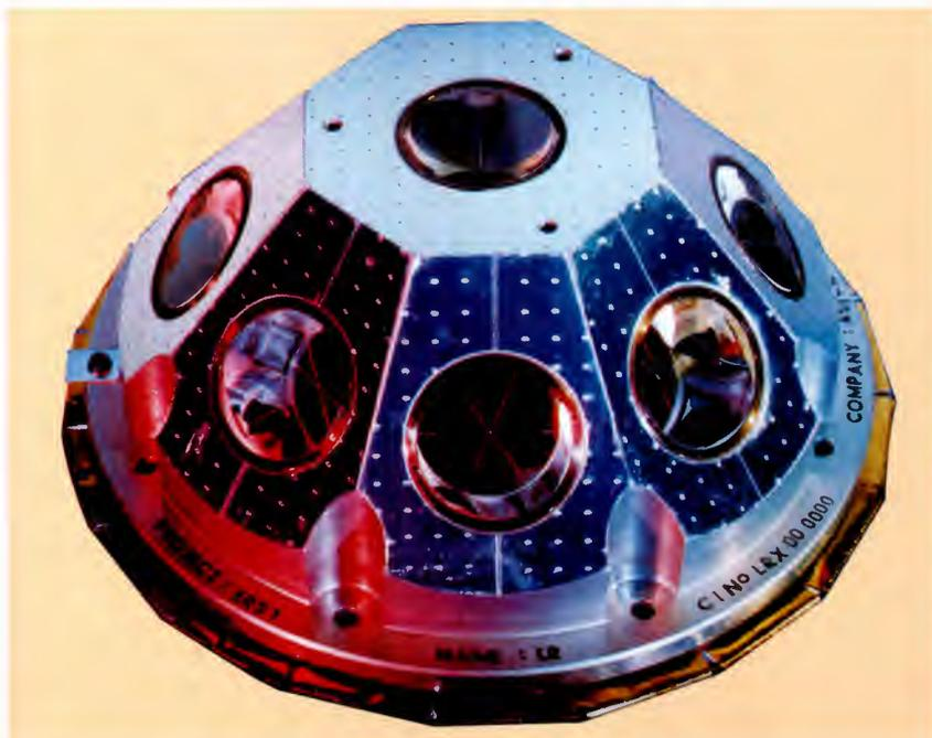
As the instrument is sensitive to the polarisation of the incoming light, a polarisation detector array monitors one polarisation direction in the broadband channels corresponding essentially to the array detector channels 2, 3, and 4.
