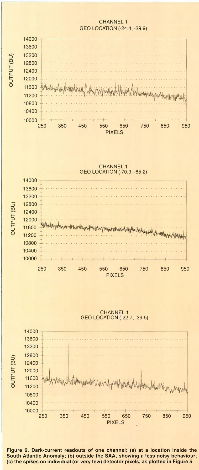
Figure 6. Dark-current readouts of one channel: (a) at a location inside the South Atlantic Anomaly; (b) outside the SAA, showing a less noisy behaviour; (c) the spikes on individual (or very few) detector pixels, as plotted in Figure 5
