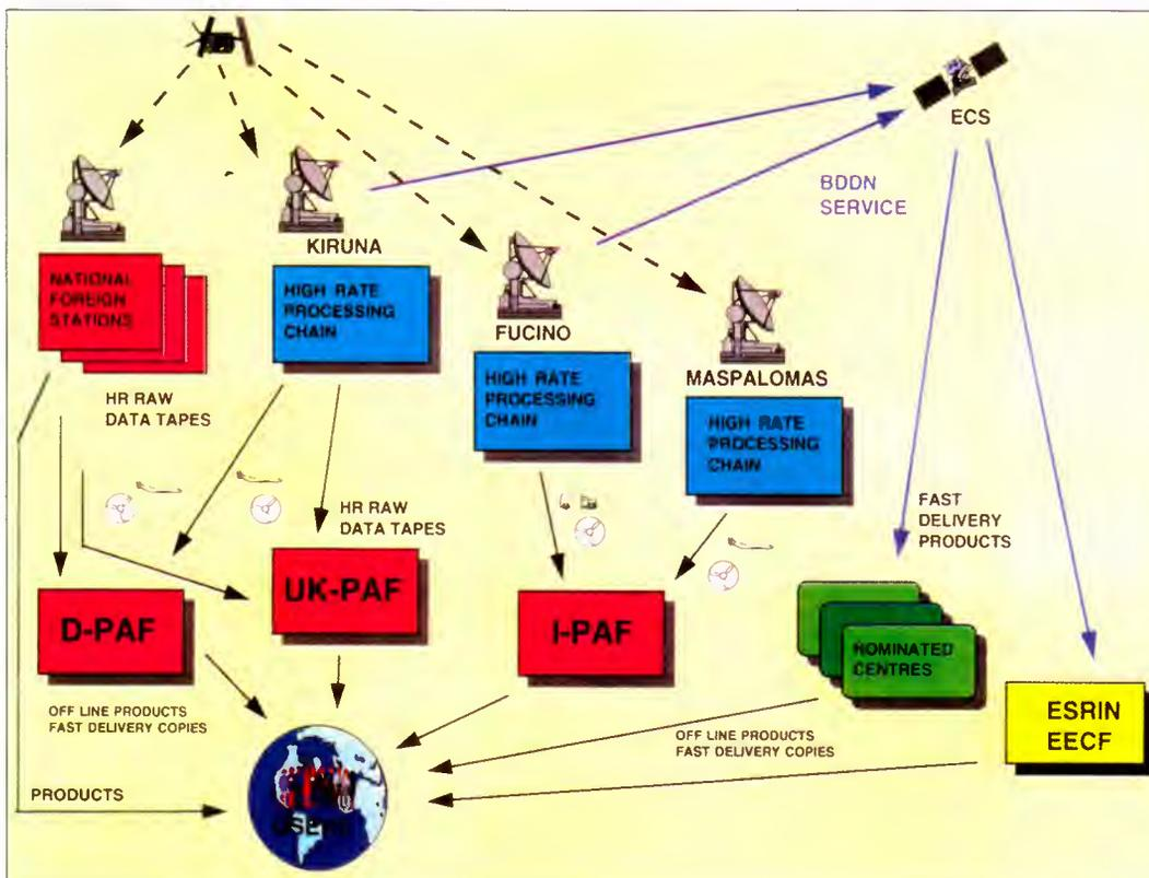
Figure 5. The flow of global high-rate data. To allow the data to reach the users quickly, the SAR images acquired at Kiruna and Fucino are transmitted directly to nominated centres via a Eutelsat satellite link. The centres then distribute the data to the users. In addition, the ground stations send the raw data to the PAFs for the off-line generation of standard products.
