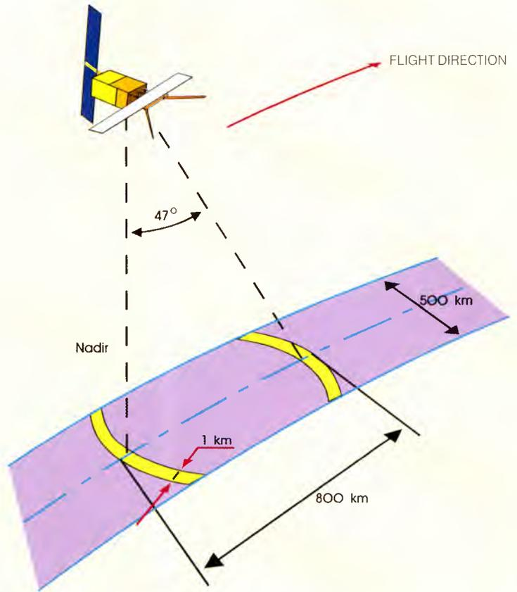
Figure 2. Measurement principle of the Along-Track Scanning Radiometer (ATSR)
