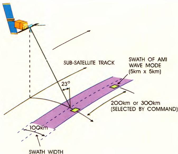
**Figure 13. The SAR Wave Mode**
