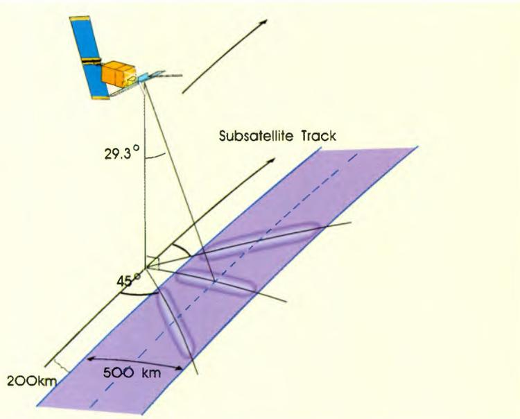
Figure 14. The SAR Wind Mode
