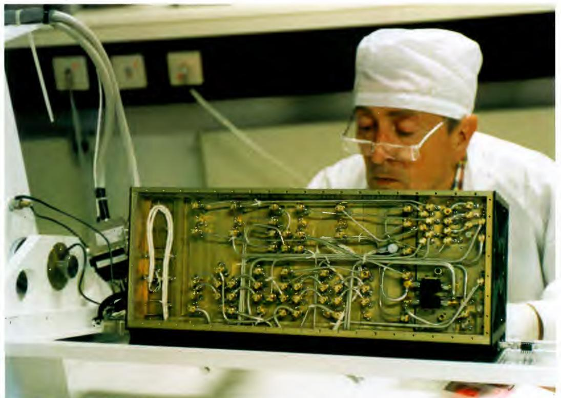
**Figure 1. The PRARE-2 instrument during integration**
