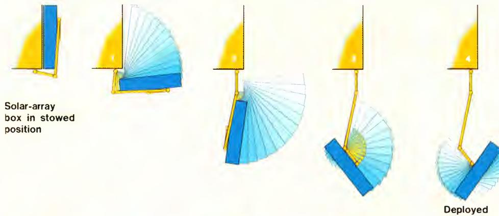
Figure 8a. Deployment of the solar-array arm
