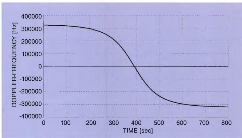
Figure 3. Typical Doppler variation during ground-station contact
