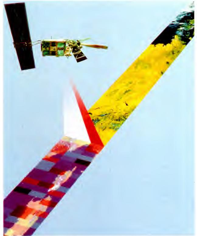
within three days. However, smaller pixel sizes can be commanded by reducing the angular extent of the scan, with spatial coverage reduced accordingly.
