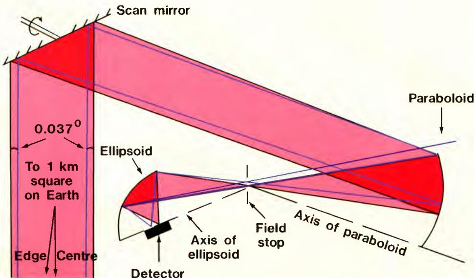
Figure 3. The arrangement of the ATSR's optical components
