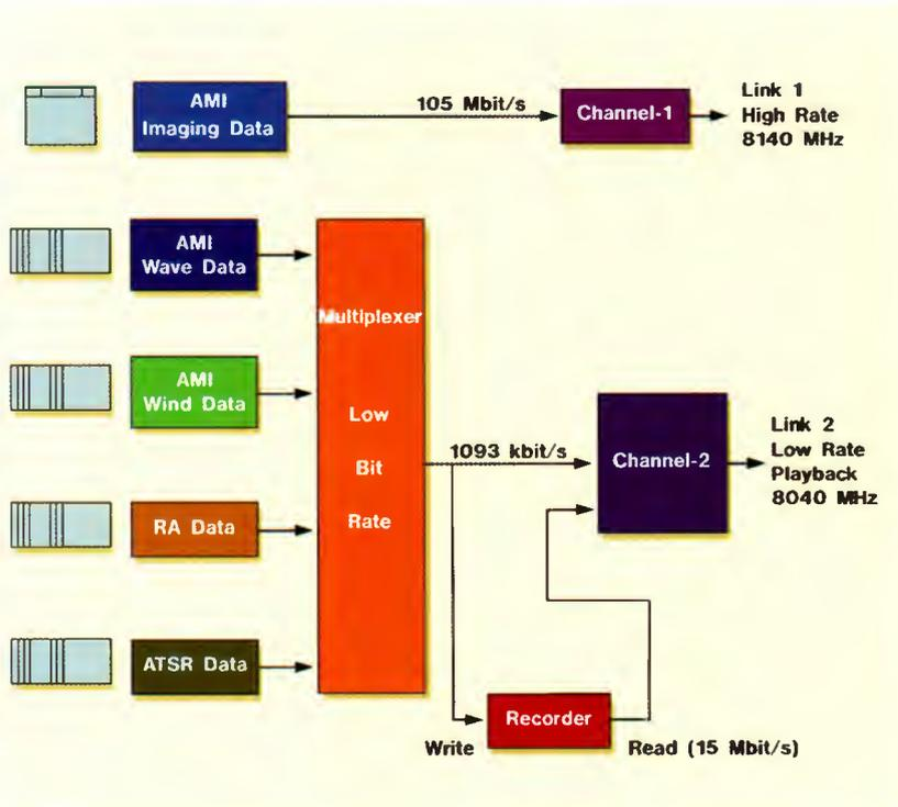
Figure 10. Block diagram of the X-band science data transmission system (IDHT)
