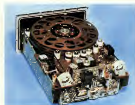
Figure 2.6. One of the two 6.5 Gbit tape recorders, which each hold 3000 ft of 1/4-inch tape. (Photo, ESA)
