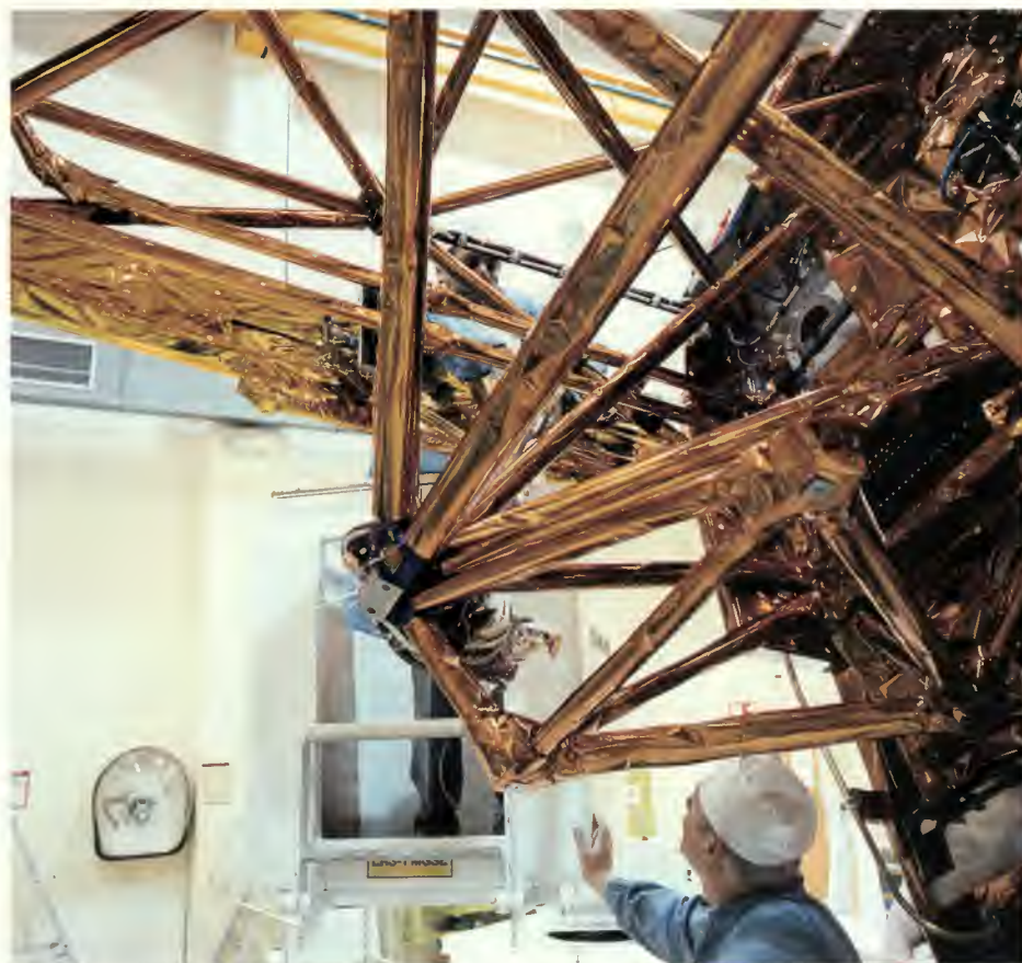
Figure 2.5. Part of the Antenna Support Structure with the antennae removed.
