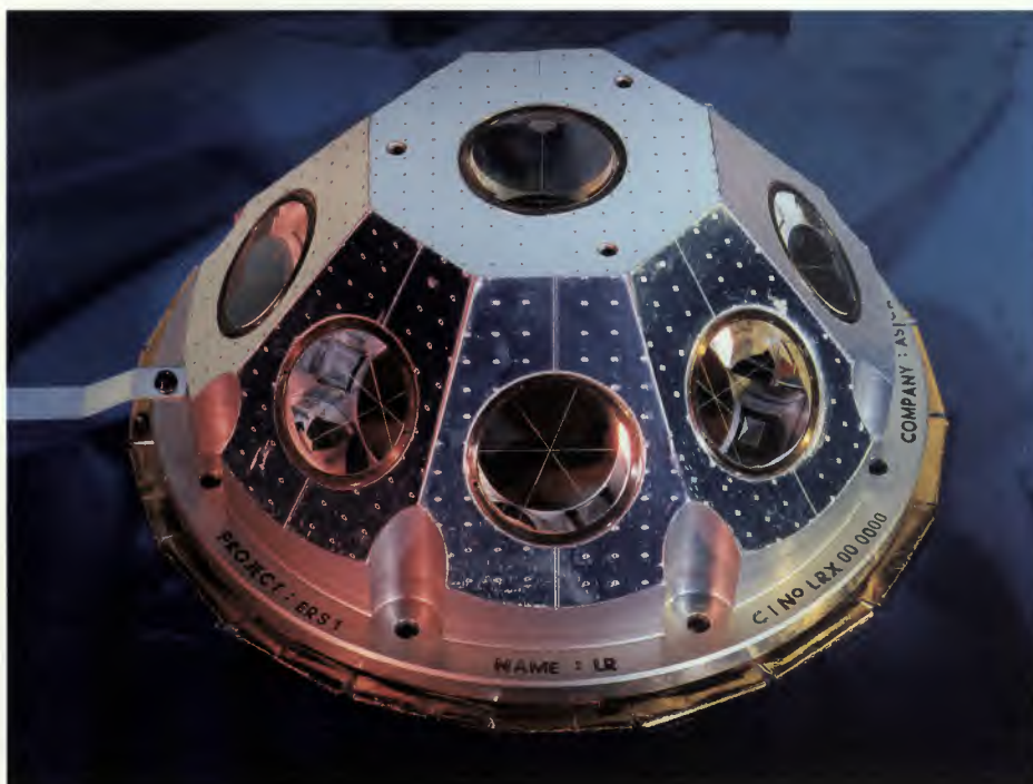
Figure 6.3. The Laser Retro-reflectors. Each corner cube is individually made, to compensate for satellite motion in reflecting incident laser energy back exactly along its incoming path.
