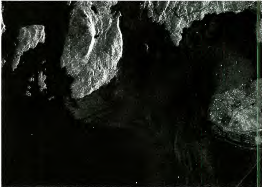
SAR image of Vancouver, Canada, processed from Seasat raw data in 30 minutes using the ERS-1 SAR Fast Delivery Processor.
