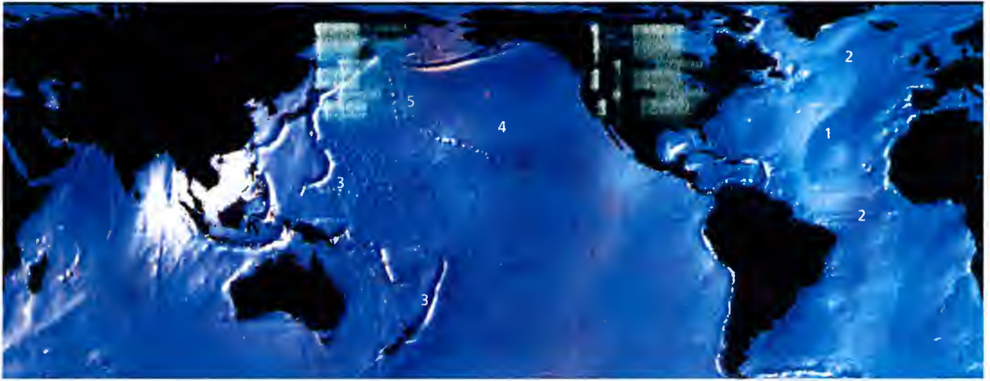
Ocean-Surface Topography. The topography of the ocean floor is reflected in the topography of the ocean surface. This Seasat derived relief map of the ocean reveals the mid-Atlantic ridge (1) and associated fracture zones (2), the Kuril, Marianas and Tonga Trenches (3), the Hawaiian island chain (4) and the older Emperor seamount chain (5). (Photo courtesy NASA).
