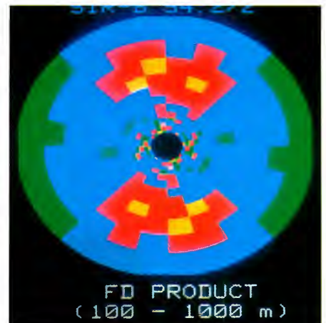
SAR Wave Mode imaggette and derived FD Power spectrum displayed in 'log polar' format with the wave energy colour coded and the radial distance proportional to the ocean wavelength.
