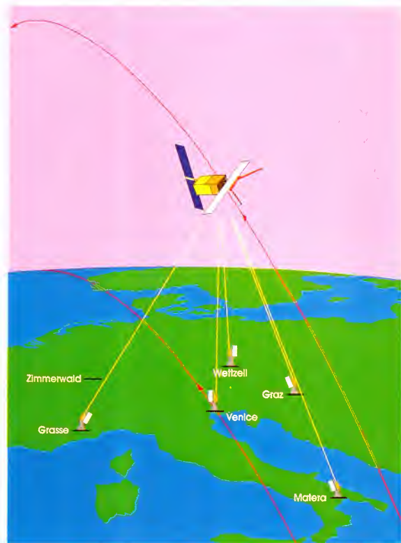
Radar Altimeter calibration using the Venice Tower and satellite laser ranging stations.
