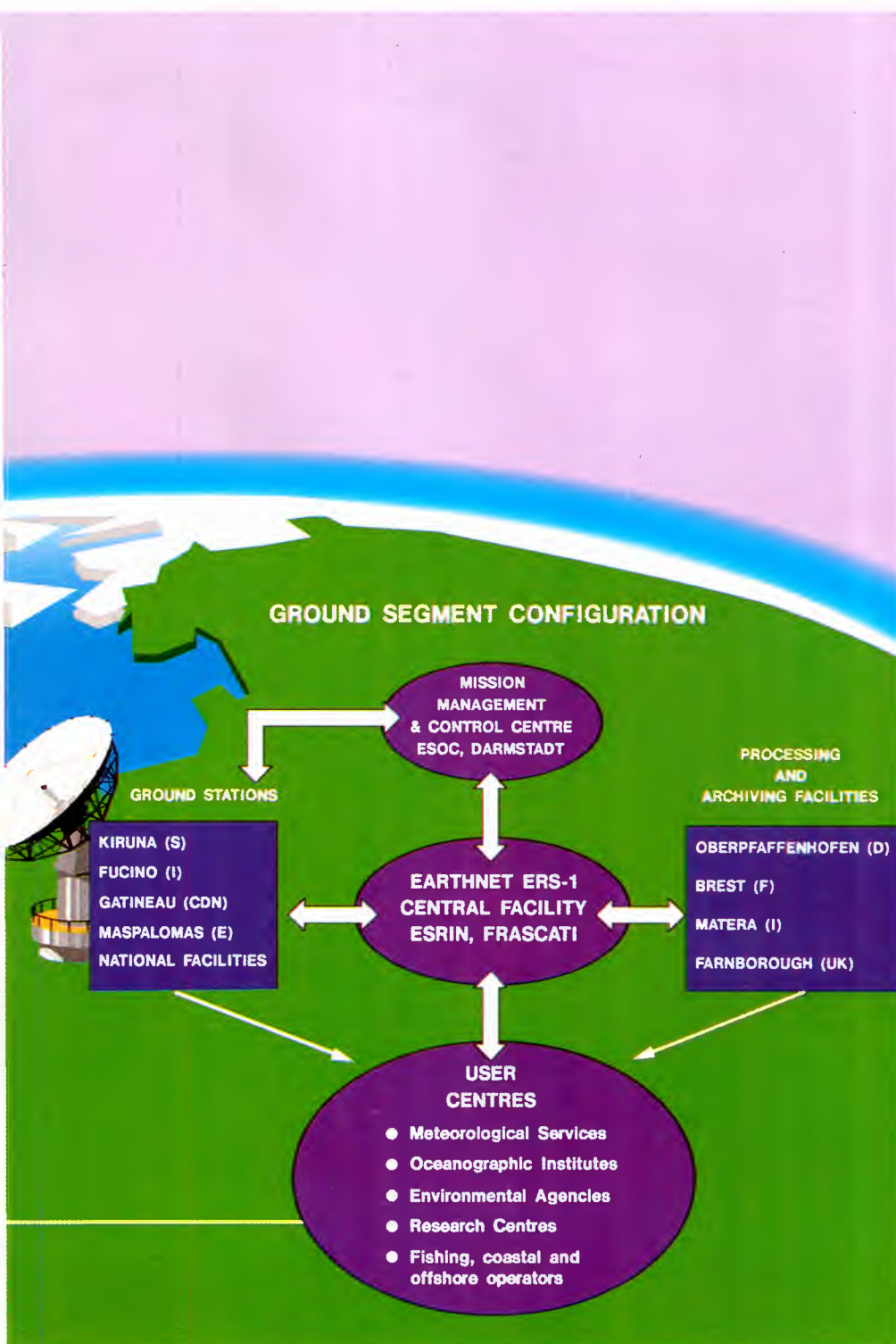
The ERS-1 Ground Segment and User interfaces.
