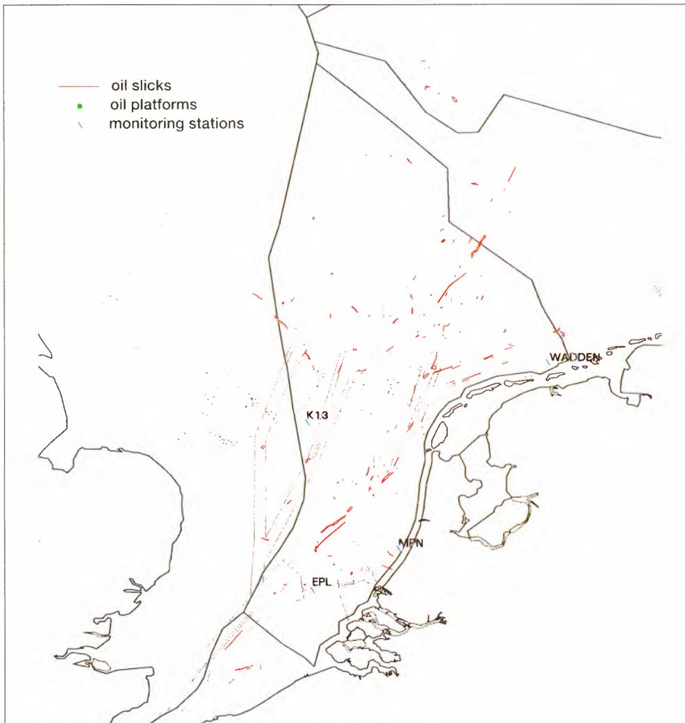
*All slicks detected by ERS-1 in the Dutch North Sea during the second half of 1993 (in red). Green points mark the positions of the oil platforms, whilst blue crosses show the positions of the monitoring stations. A clear correlation is apparent between the positions and directions of the slicks and the locations of the shipping lanes*
