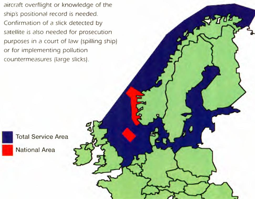
The Norwegian oil-spill-service coverage area (blue) and national high-priority area (red). ERS SAR data for the blue and red areas are analysed in near-real-time
