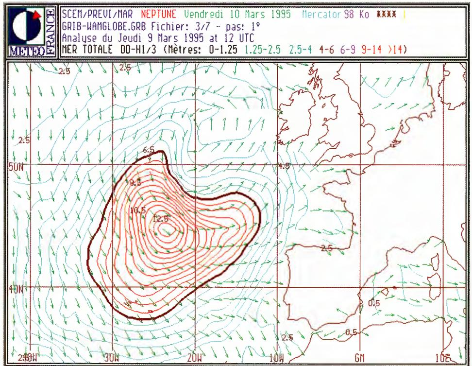
The data are transmitted via the Inmarsat-C satellite to an onboard desktop computer equipped with the appropriate interpretation software. The information can be viewed either in the form of a chart, or in a user-defined format if the extraction of particular information, such as waves exceeding a particular height, is required.
