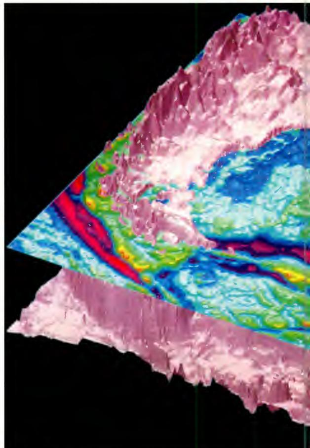
The Radar Altimeter measures the height of the satellite above the sea surface to an accuracy of approximately 10 cm, allowing the inferral of gravity anomalies arising from subsea geological structures with oil-bearing potential.
