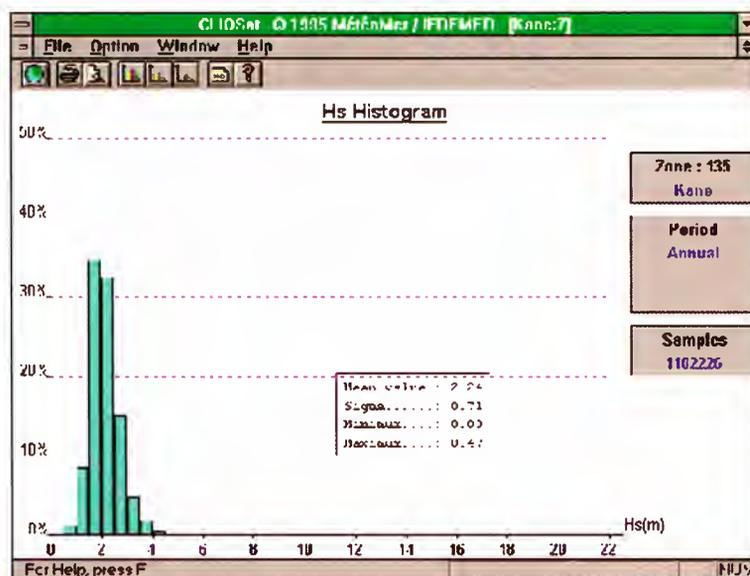
Two sample products from CLIOSat: a histogram of the distribution of the wave direction on an annual basis for an area in the Central Atlantic (above) and a histogram of the wave heights for the same area on an annual basis (below)
