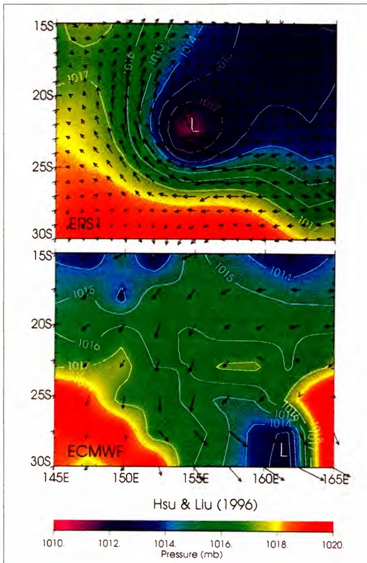
Surface wind vectors (dark arrows) and surface pressures around tropical cyclone Oliver, derived from ERS-1 Scatterometer data and from ECMWF data at 12 UTC on 11 February 1993. The cyclone was located in the Southern Pacific, where in-situ observations are sparse. The improvement with ERS data in describing such features is self-evident
