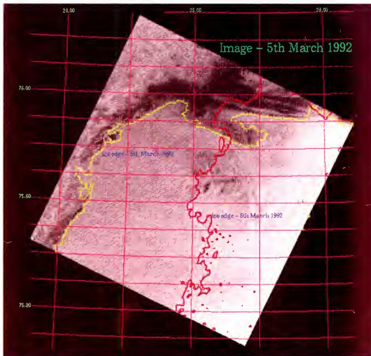
Typical ice-edge product from the Ice Prediction and Analysis Platform (IPAP) experiment. The area to the west in the image consists of first-year ice with a fringing of grease ice. The image is overlaid by two edge lines, one generated from the displayed image, and one from the next overpass of the satellite three days later
