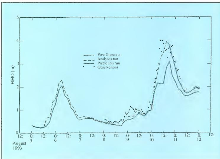
Effect of the assimilation of ERS Altimeter data on wave prediction: the forecast provided matched the reality very well
