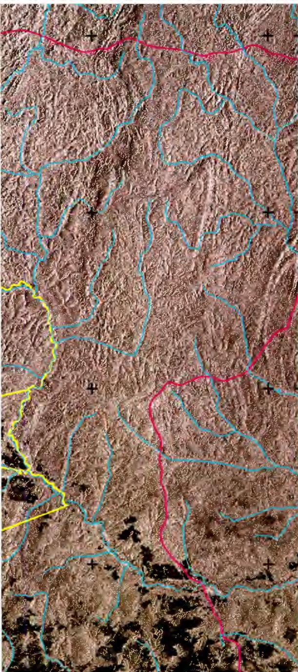
Differential interferometry allows one to measure surface movements with a sensitivity of the order of a few centimetres over large surfaces. This technique can be applied for subsidence monitoring and in the observation of active volcanoes, earthquakes and faults.
