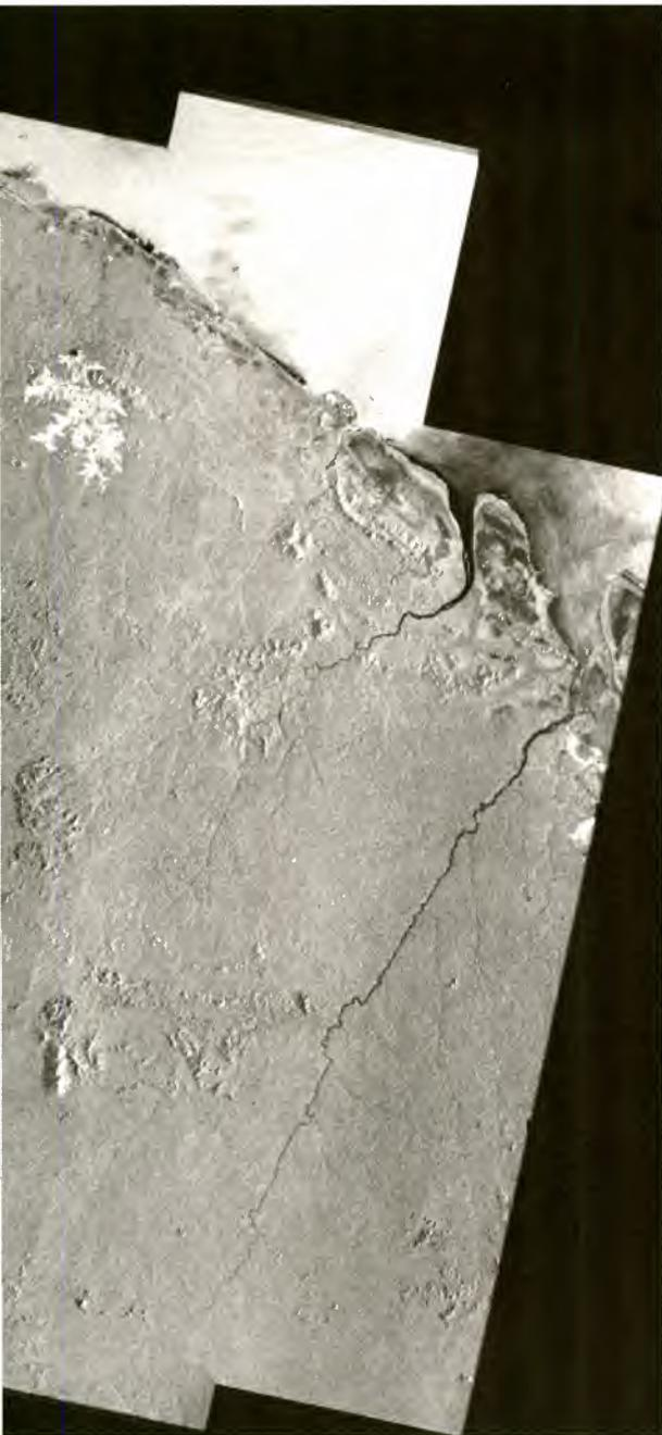
*ERS SAR mosaic image of French Guiana based on data acquired in descending mode. It was generated by merging two groups of 18 PRI ERS images in descending mode, acquired at two different time periods, in 1992 and in 1993-94, respectively. In addition, a strip of five scenes acquired in ascending mode has been used for localisation purposes, including height references*
