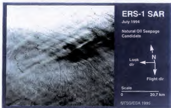
ERS-1 SAR image data examples: Confirmed oil spill (upper), candidate spills, ships, wind front (middle), and a seepage candidate (lower).
