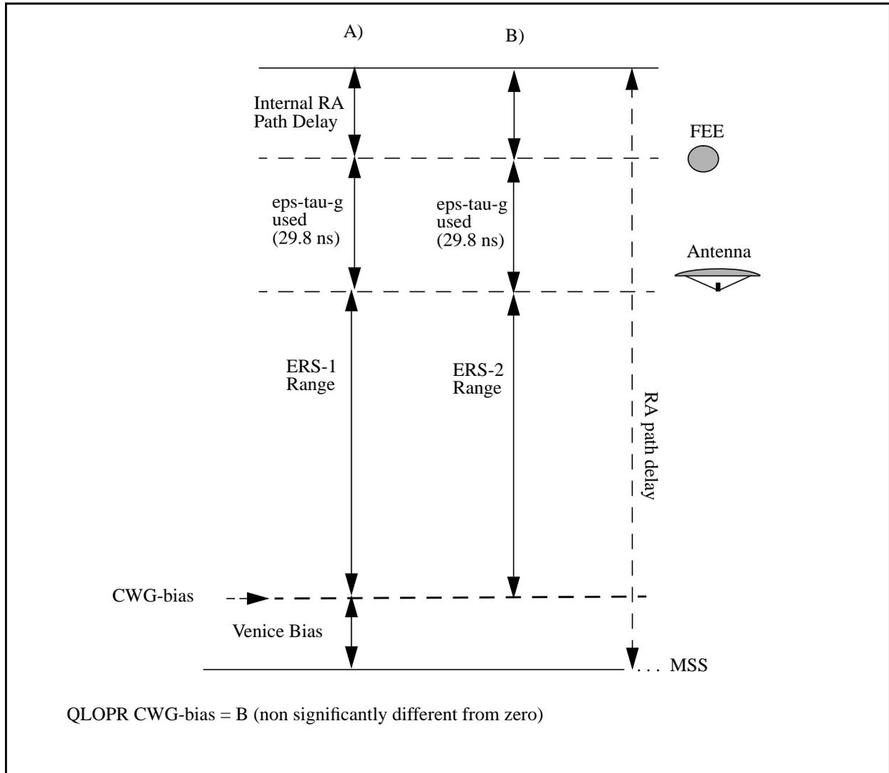
Figure I: Representation of the Radar Altimeter global path delay for the following configurations: A) Present ERS-1 QLOPR configuration, B) Present ERS-2 QLOPR configuration.
