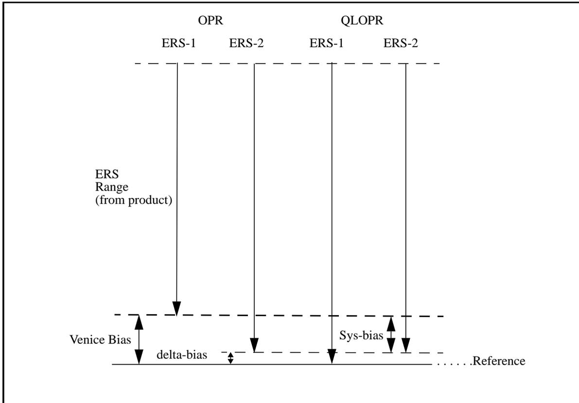
Figure III: Representation of the different ERS Altimetric Ranges as read from the products in the ERS Ground Segment Configuration as defined in chapter 4.
