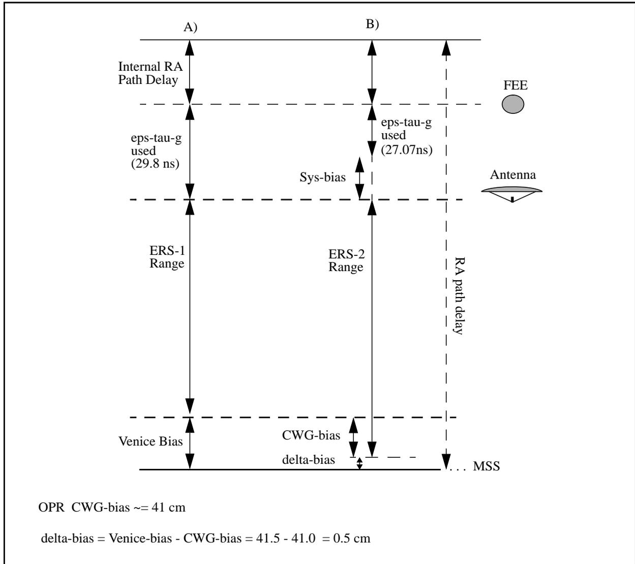
Figure II: Representation of the Radar Altimeter global path delay for the following configurations: A) Present ERS-1 OPR configuration., B) Present ERS-2 OPR configuration.
