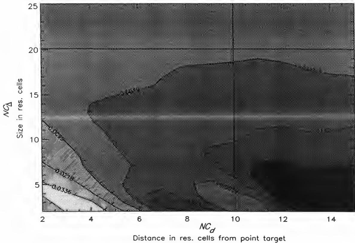
**Figure 2.** Calibration constant variations (in decibels) as a function of  $NC_d$  and  $NC_\Delta$ .
