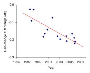
Fig. 1. Difference between the measured and reference antenna patterns at far range (+3° from boresight)
