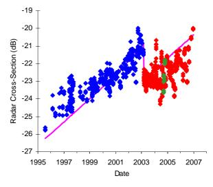
Fig. 9(a). ERS-2.SAR.PRI Noise Equivalent  $\sigma^{o}$  as a function of acquisition date
