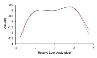
Fig. 2(a). Reference (blue) and new (red) ERS-2 SAR elevation antenna patterns
