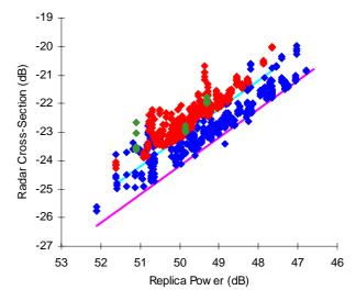
Fig. 9(b). ERS-2.SAR.PRI Noise Equivalent  $\sigma^{o}$  as a function of replica pulse power
