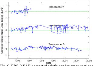
Fig. 6. ERS-2 SAR corrected relative radar cross-sections for the ESA transponders (up to November 2001)
