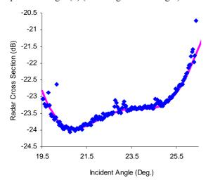
Fig. 9(d). ERS-2.SAR.PRI Noise Equivalent  $\sigma^{\circ}$  from Orbit 16652, Frame 2403 (27<sup>th</sup> June 1998)
