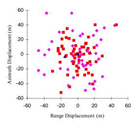
Fig. 12. ERS-2.SAR.PRI image localisation using the ESA transponders (blue triangles for transponder#1, purple diamonds for transponder#2 and red squares for transponder#3)
