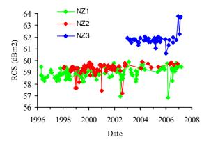
Fig. 8(b). Neustrelitz radar cross-section
