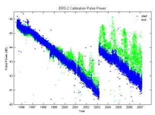
Fig. 4(a). ERS-2 SAR calibration pulse powers
