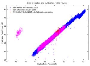
Fig. 4(c). Relationship between ERS-2 replica and calibration pulse powers. The purple symbols show the pulse powers since the end of February 2003.
