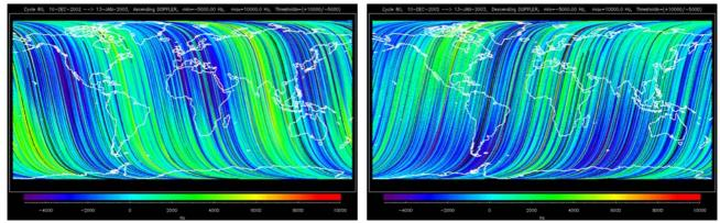
Fig. 11. ERS-2 Doppler Centroid Frequency during Repeat Cycle 80 (December 2002-January 2003) for ascending passes (left) and descending passes (right). Blue is -5000Hz and red is 10000Hz
