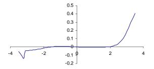
Fig. 2(b). Difference between the reference and new elevation antenna patterns
