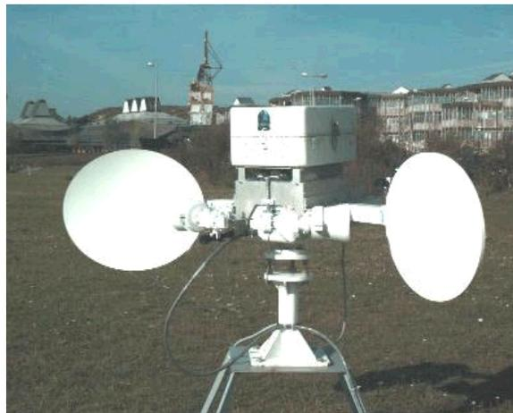
**Figure 2.4: Prototype ASAR Transponder**
