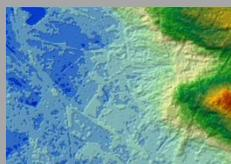
The **digital terrain model layer** contains the height values as a geocoded raster file. This layer is derived from a DSM and shows the terrain heights (vegetation and buildings removed). With the DTM, a mask layer is also provided to be able to trace the DSM to DTM conversion. For the DTM product the availability and accuracy depends on the specific area of interest.
