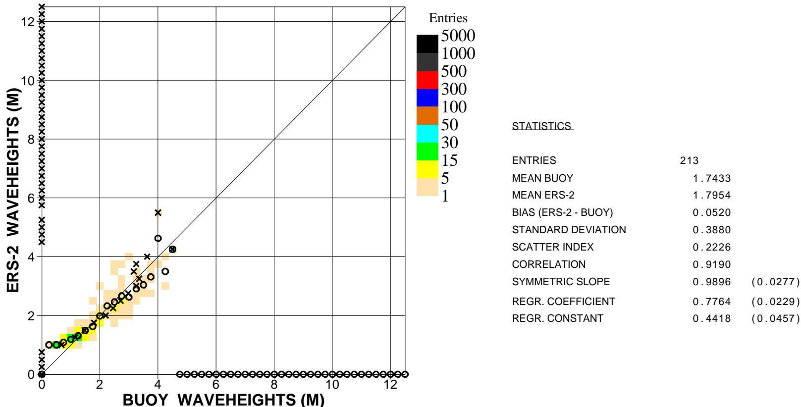
Figure 21. Comparison of buoy wave height observations with ERS2 Altimeter wave height data for September 2009 (global)
