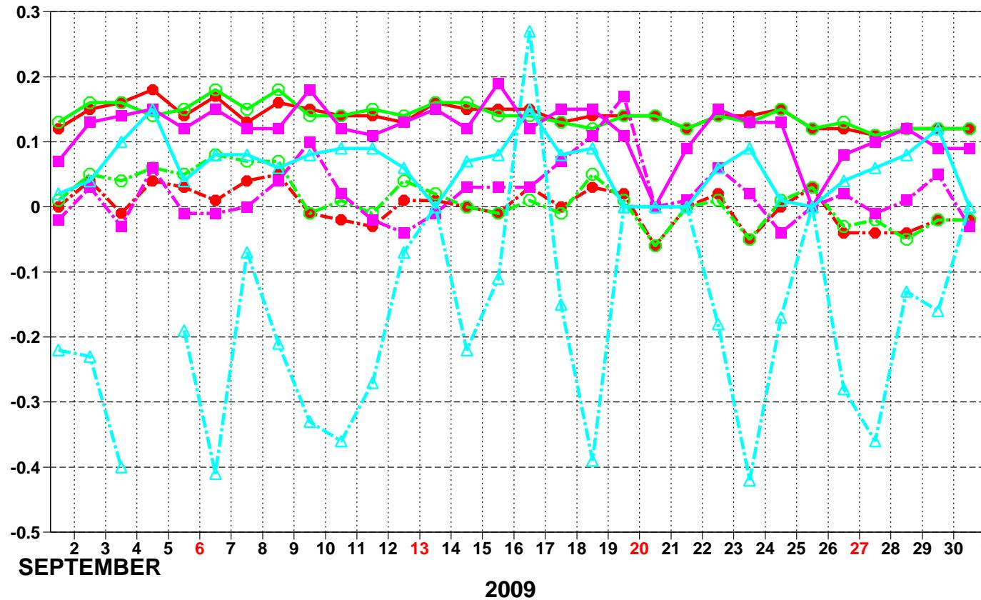
Figure 24: ERS-2 Altimeter wave heights: Timeseries of bias (ERS-2 - model) and scatter index (SI)
