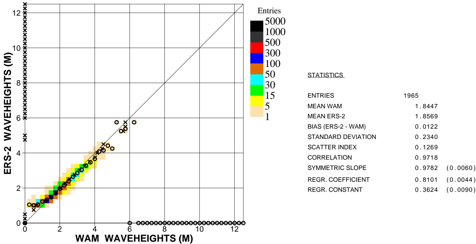
Figure 19. Comparison of ECMWF wave height results with ERS2 Altimeter wave height data for September 2009 (tropics)
