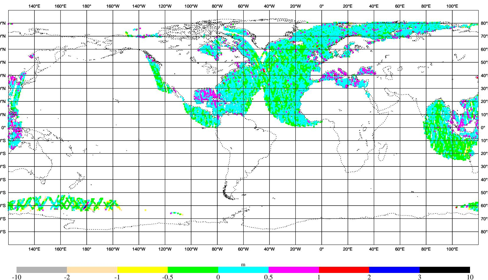
Figure 27: Significant wave height: Monthly mean difference of ERS-2 altimeter data minus wave model results for September 2009.
