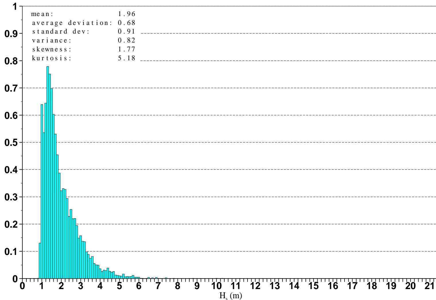
Figure 15: Distribution of ERS-2 Altimeter wave heights after along track averaging for September 2009
