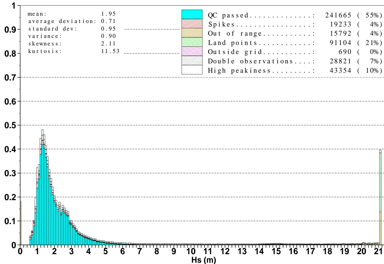
Figure 14: Distribution of the ERS-2 Altimeter wave heights after QC for September 2009
