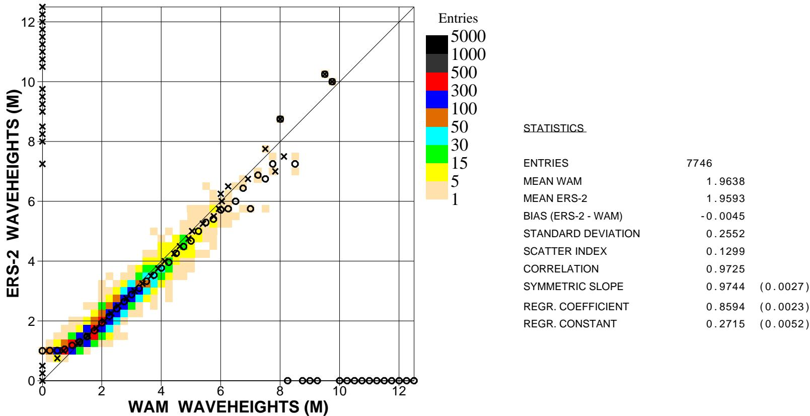
Figure 17. Comparison of ECMWF wave height results with ERS2 Altimeter wave height data for September 2009 (global)
