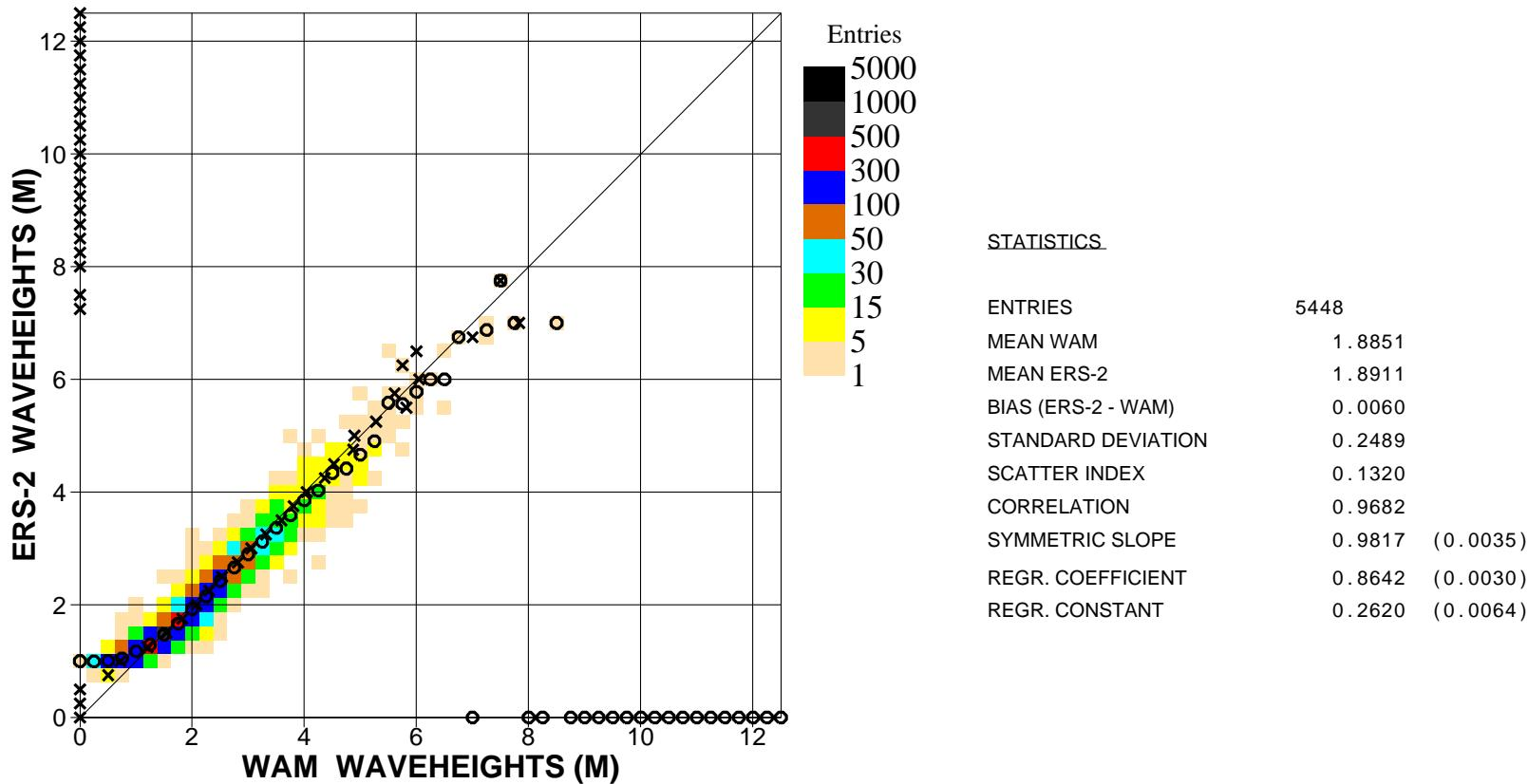
Figure 18. Comparison of ECMWF wave height results with ERS2 Altimeter wave height data for September 2009 (n.hem.)
