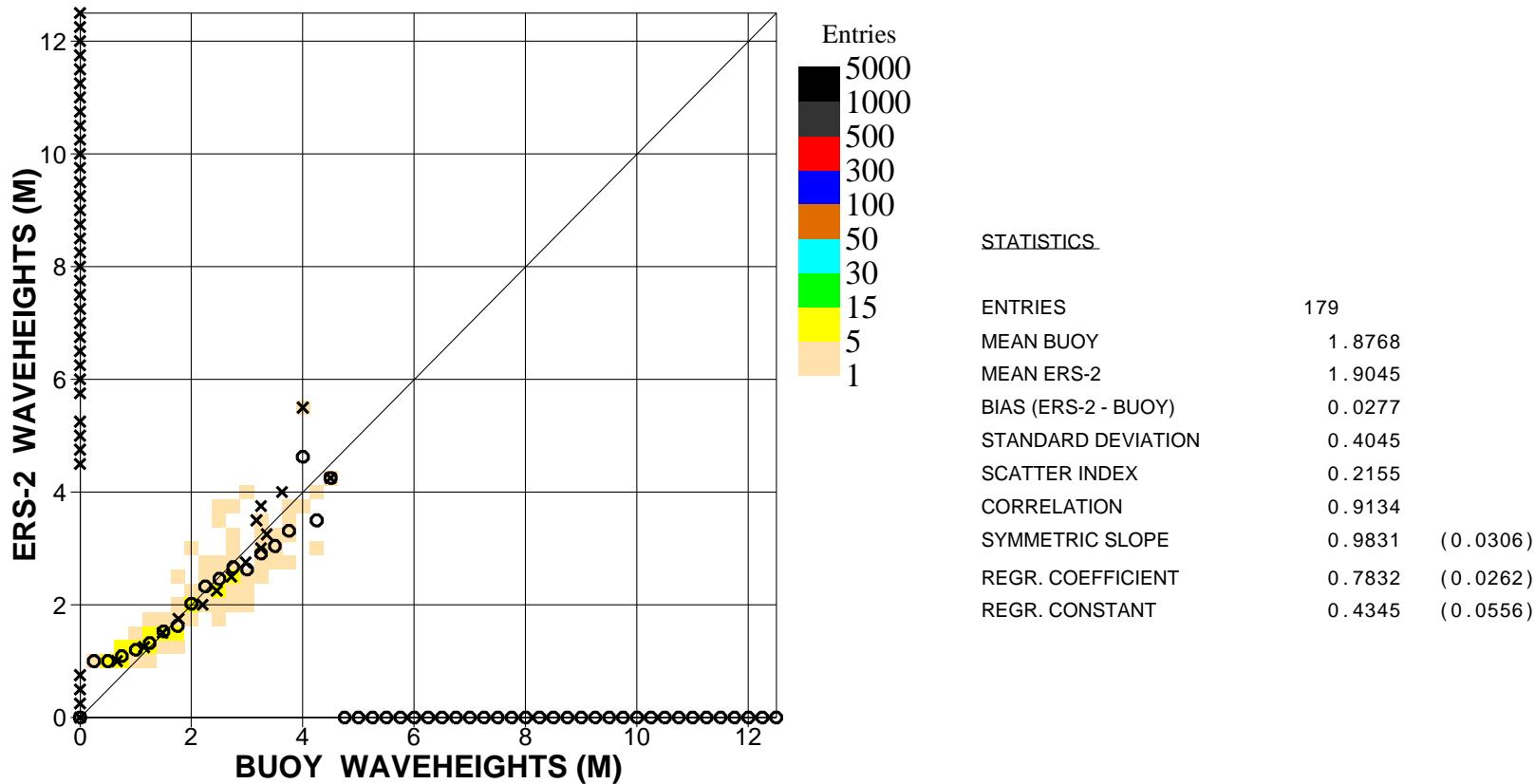
Figure 22. Comparison of buoy wave height observations with ERS2 Altimeter wave height data for September 2009 (n.hem.)
