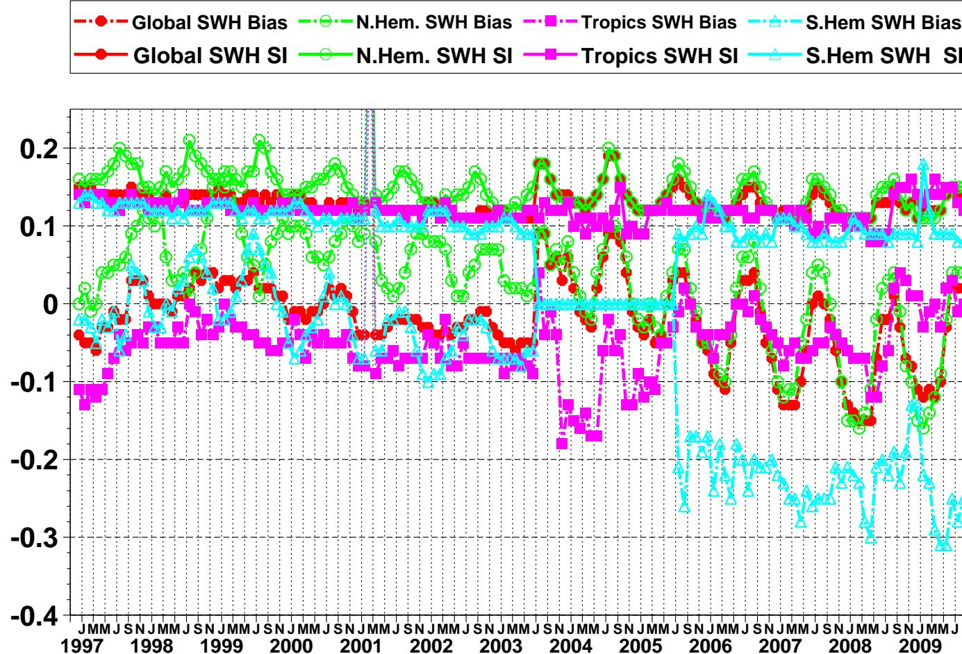
Figure 25: ERS-2 Altimeter wave heights: Timeseries of bias (ERS-2 - model) and scatter index (SI)
