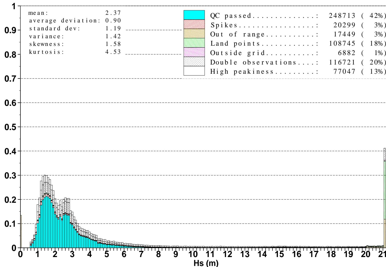
Figure 14: Distribution of the ERS-2 Altimeter wave heights after QC for March 2009
