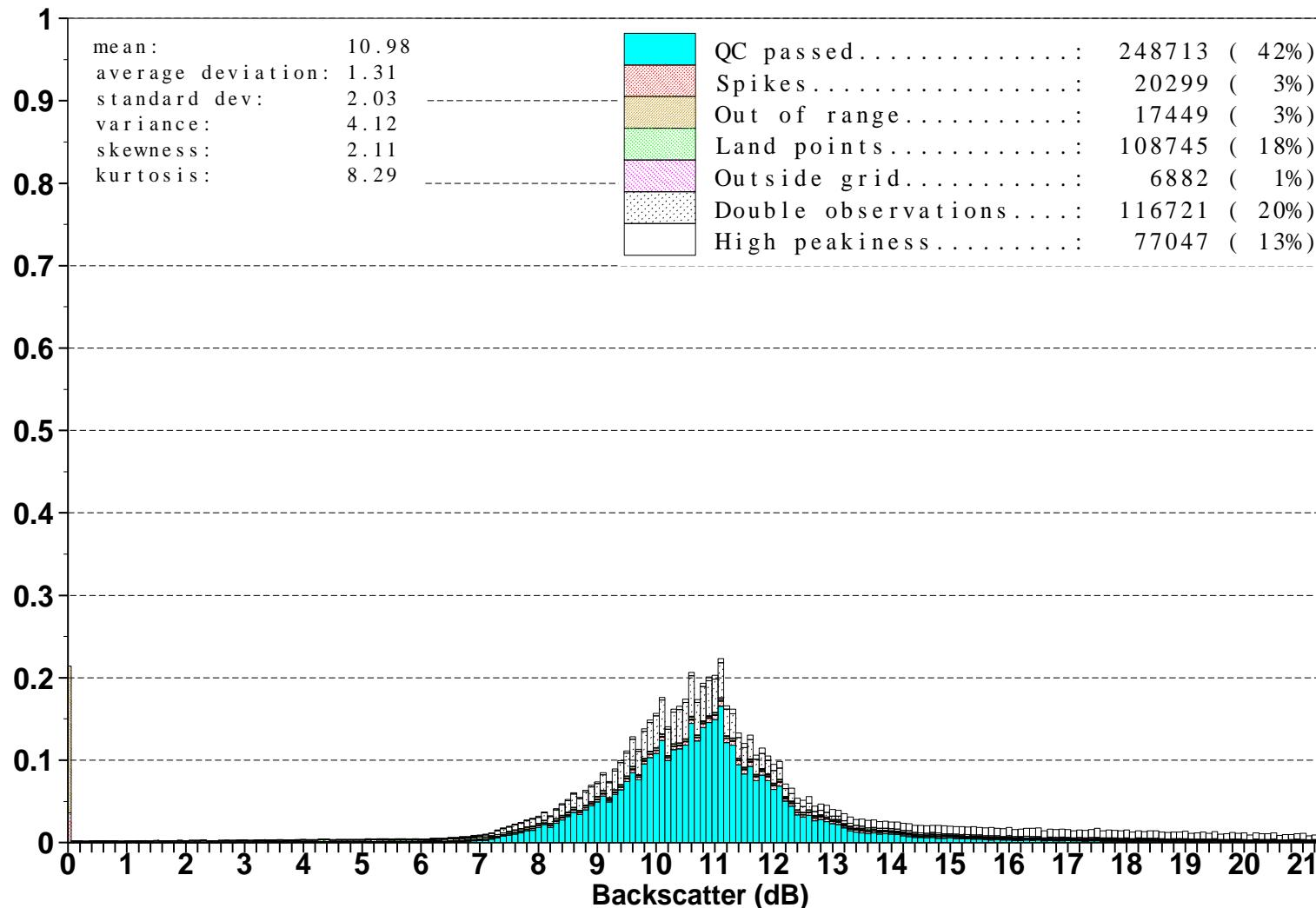
Figure 2: Distribution of the ERS-2 Altimeter backscatter after QC for March 2009
