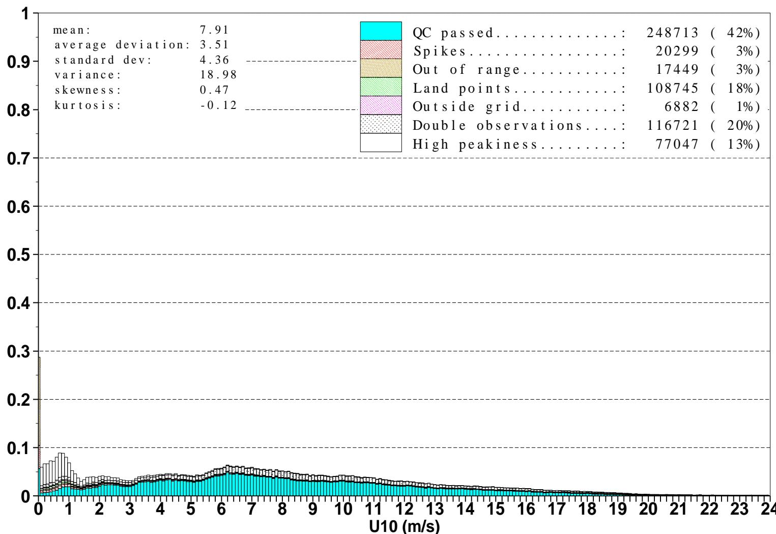
Figure 3: Distribution of the ERS-2 Altimeter wind speeds after QC for March 2009
