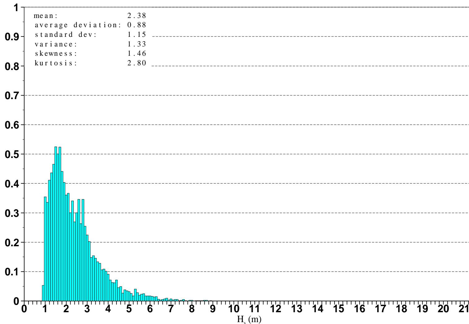
Figure 15: Distribution of ERS-2 Altimeter wave heights after along track averaging for March 2009
