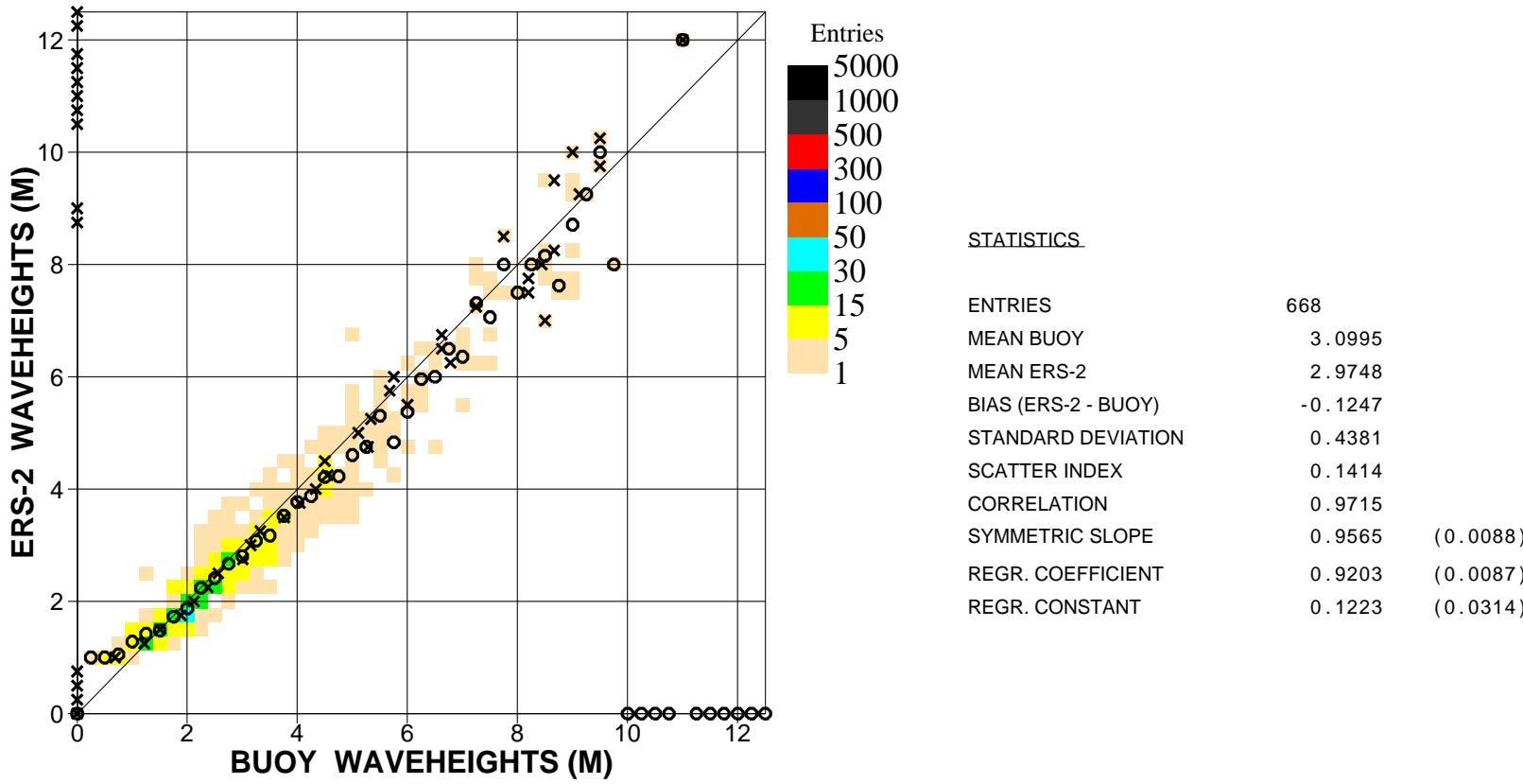
Figure 22. Comparison of buoy wave height observations with ERS2 Altimeter wave height data for March 2007 (n.hem.)
