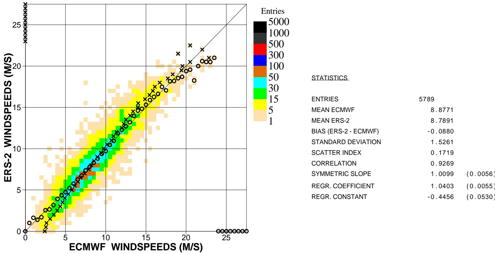
Figure 7. Comparison of ECMWF wind speed results with ERS2 Altimeter wind speed data for March 2007 (n.hem.)
