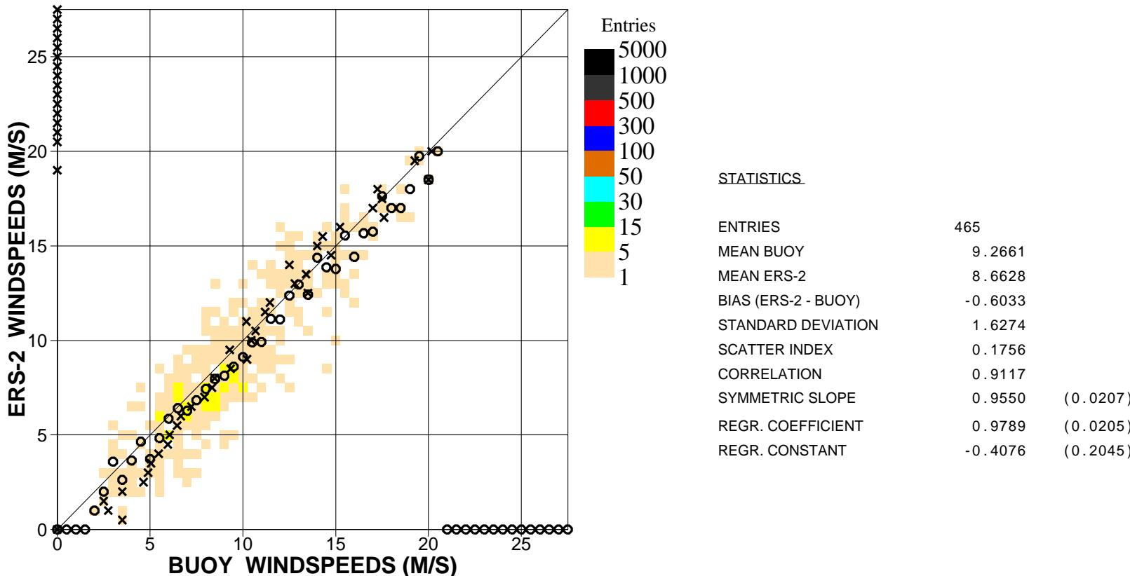
Figure 10. Comparison of buoy wind speed observations with ERS2 Altimeter wind speed data for March 2007 (global)
