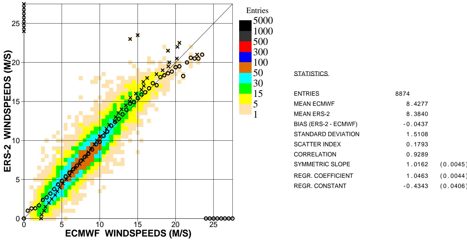
Figure 6. Comparison of ECMWF wind speed results with ERS2 Altimeter wind speed data for March 2007 (global)
