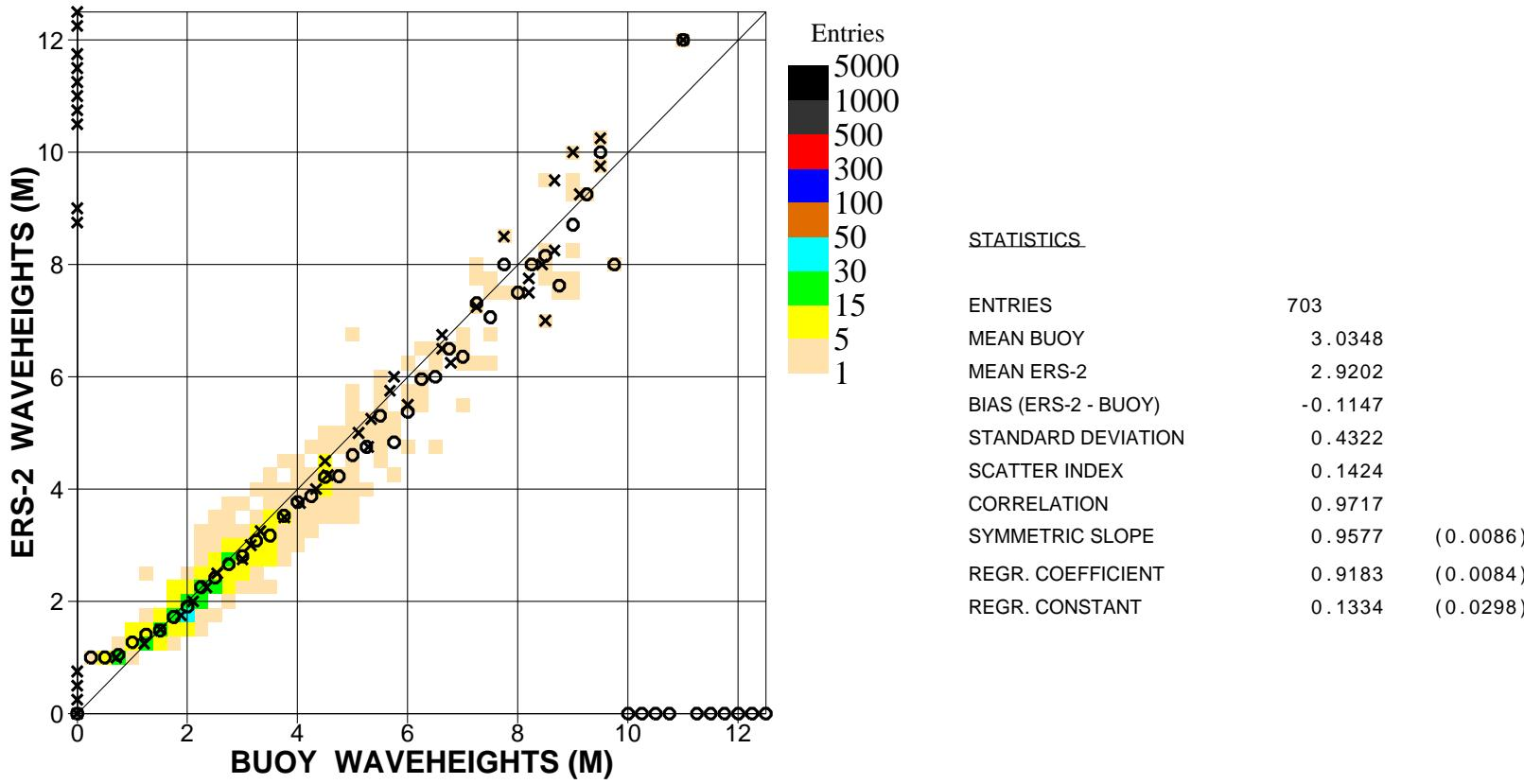
Figure 21. Comparison of buoy wave height observations with ERS2 Altimeter wave height data for March 2007 (global)
