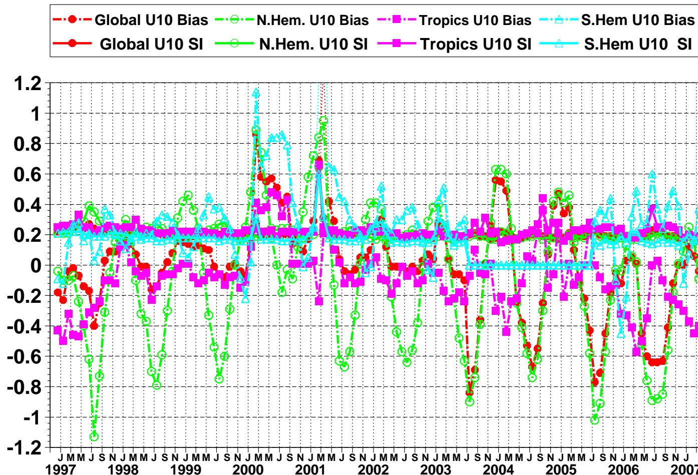
Figure 26: ERS-2 Altimeter wind speeds: Timeseries of bias (ERS-2 - model) and scatter index (SI)
