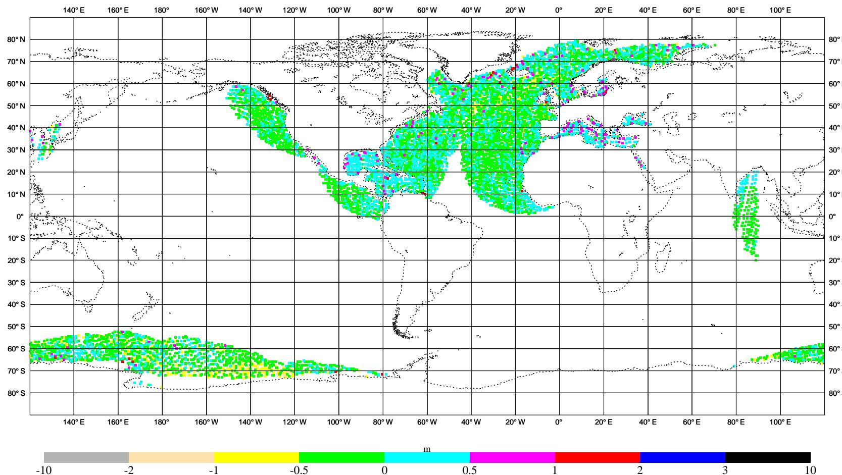
Figure 27: Significant wave height: Monthly mean difference of ERS-2 altimeter data minus wave model results for March 2007
