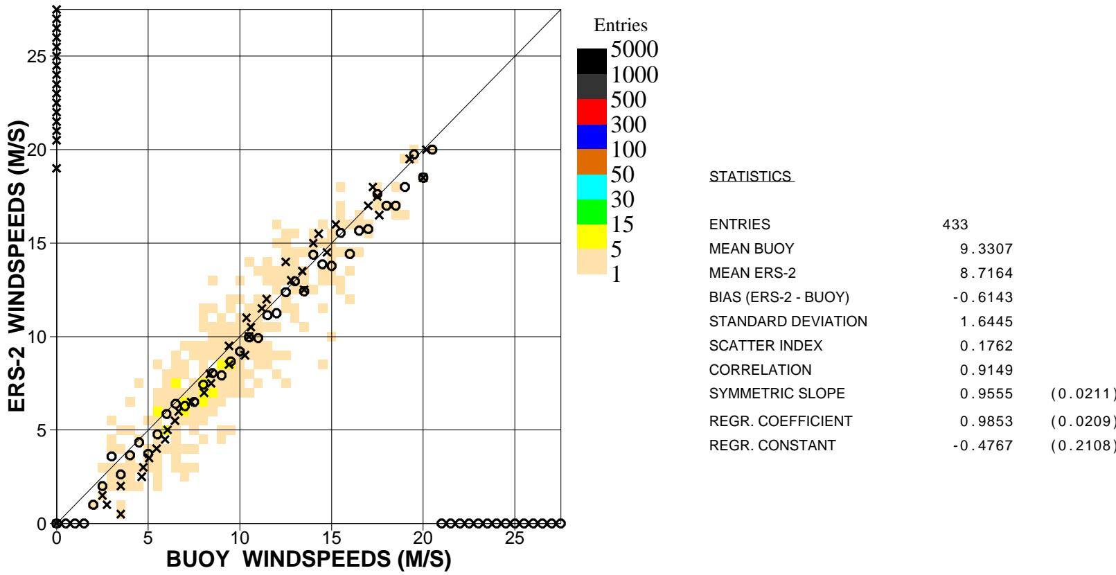
Figure 11. Comparison of buoy wind speed observations with ERS2 Altimeter wind speed data for March 2007 (n.hem.)
