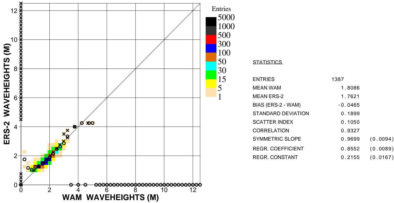
Figure 19. Comparison of ECMWF wave height results with ERS2 Altimeter wave height data for March 2007 (tropics)
