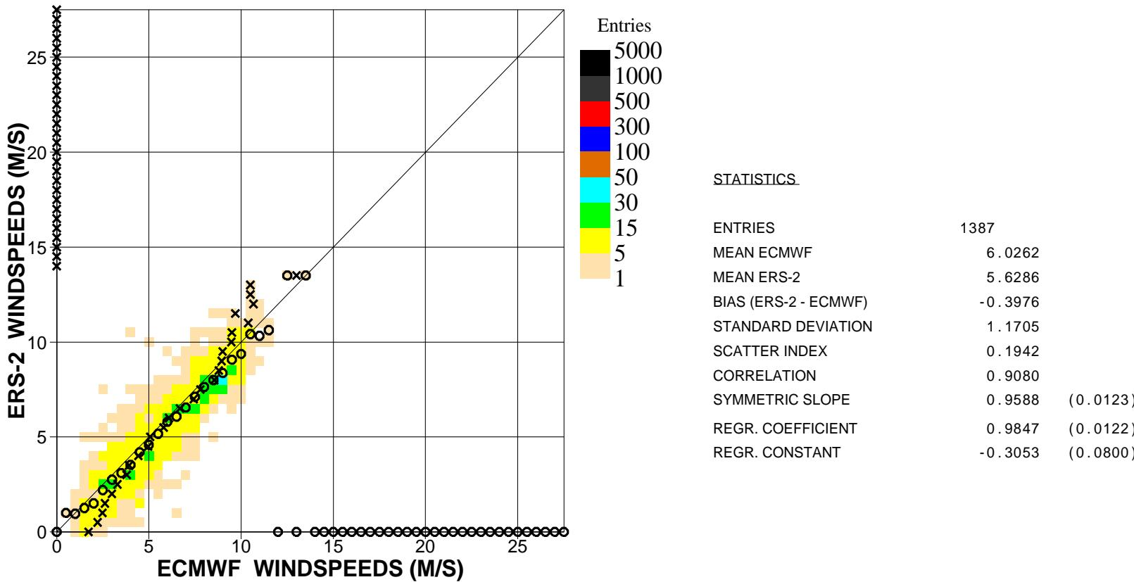
Figure 8. Comparison of ECMWF wind speed results with ERS2 Altimeter wind speed data for March 2007 (tropics)
