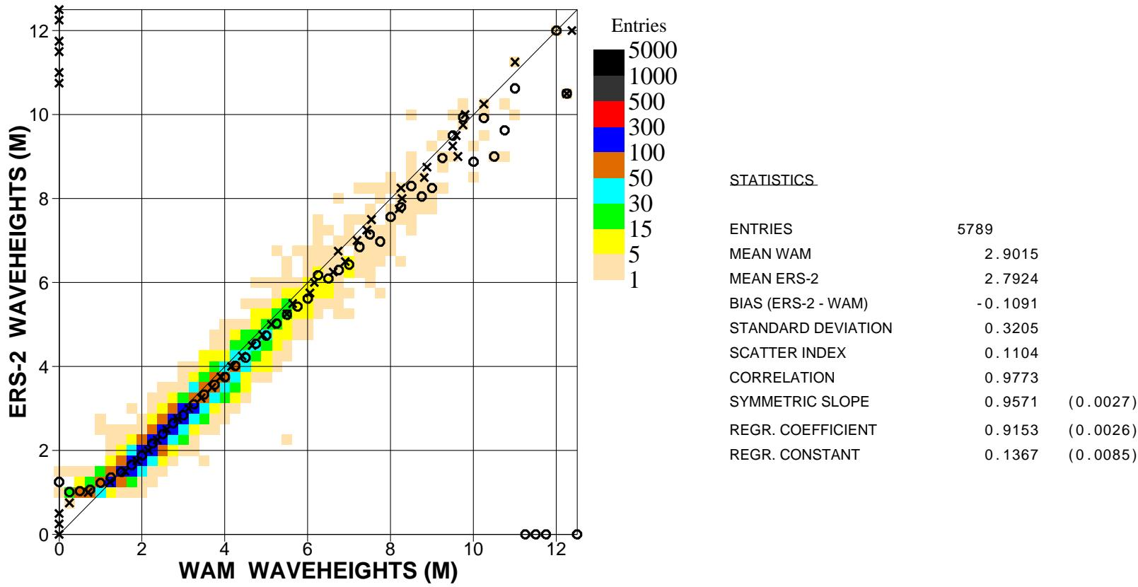
Figure 18. Comparison of ECMWF wave height results with ERS2 Altimeter wave height data for March 2007 (n.hem.)
