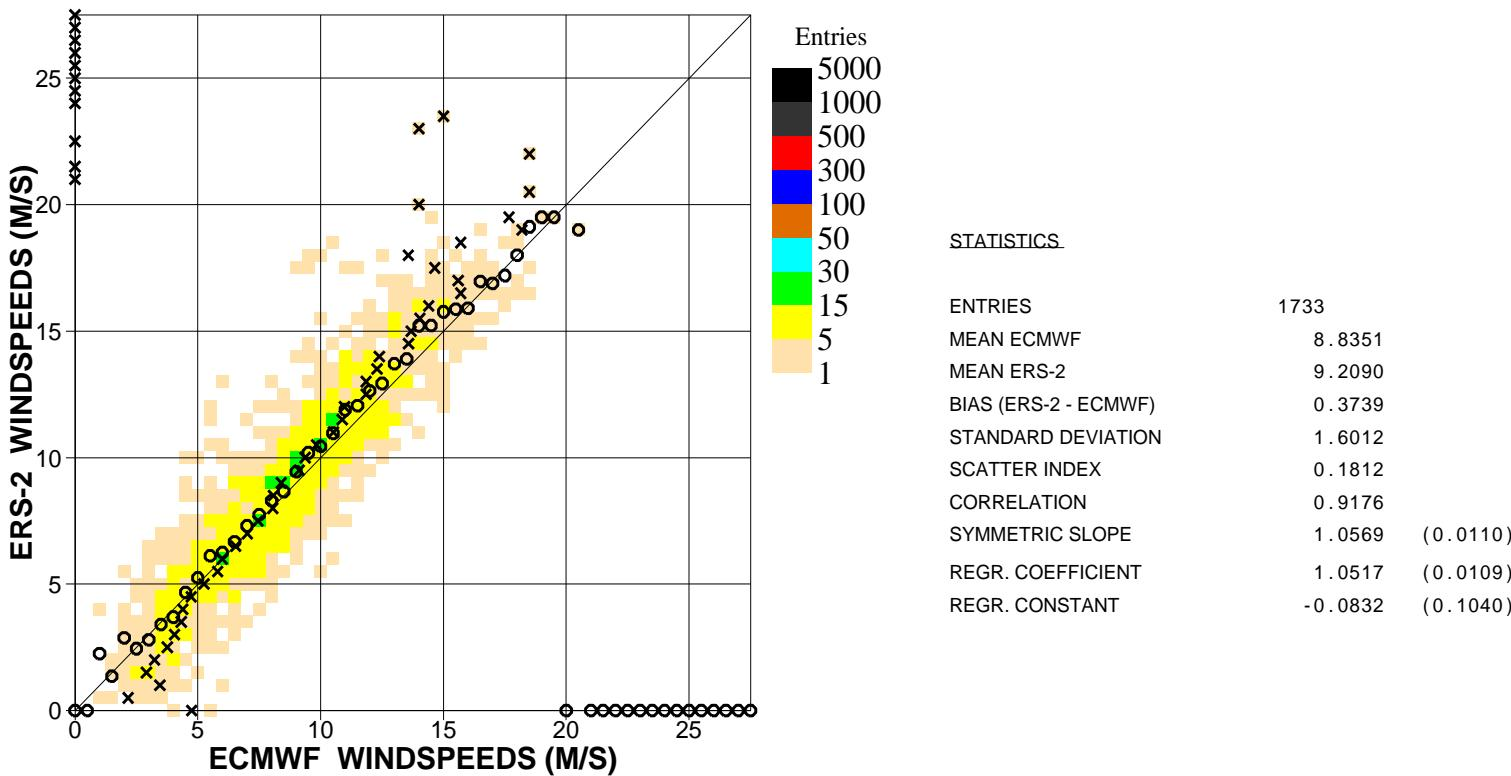
Figure 9. Comparison of ECMWF wind speed results with ERS2 Altimeter wind speed data for March 2007 (s.hem.)
