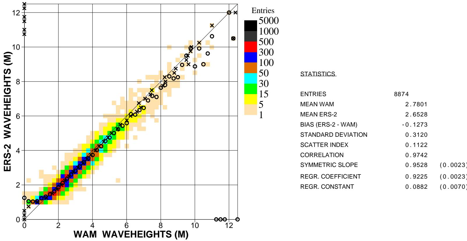
Figure 17. Comparison of ECMWF wave height results with ERS2 Altimeter wave height data for March 2007 (global)
