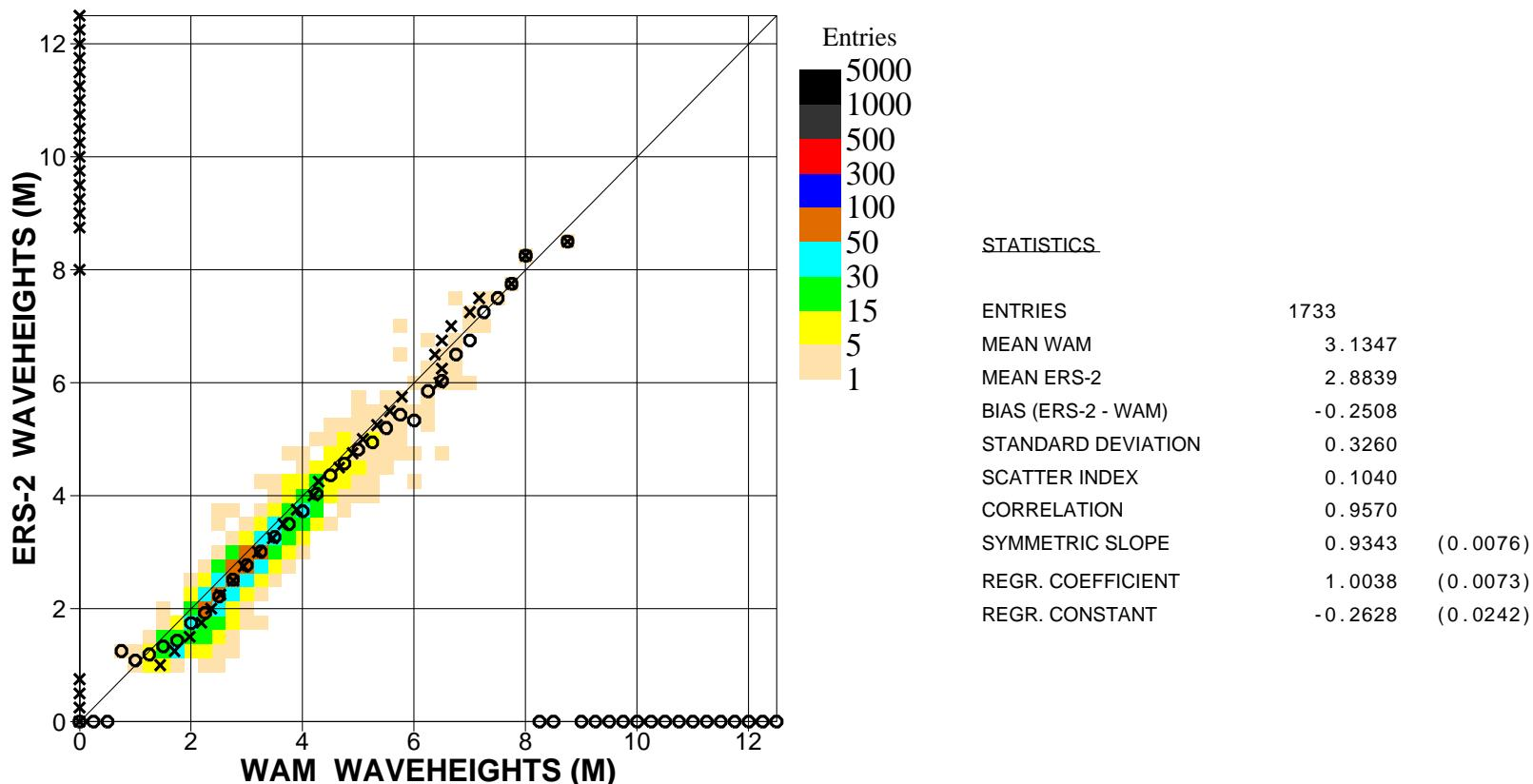
Figure 20. Comparison of ECMWF wave height results with ERS2 Altimeter wave height data for March 2007 (s.hem.)
