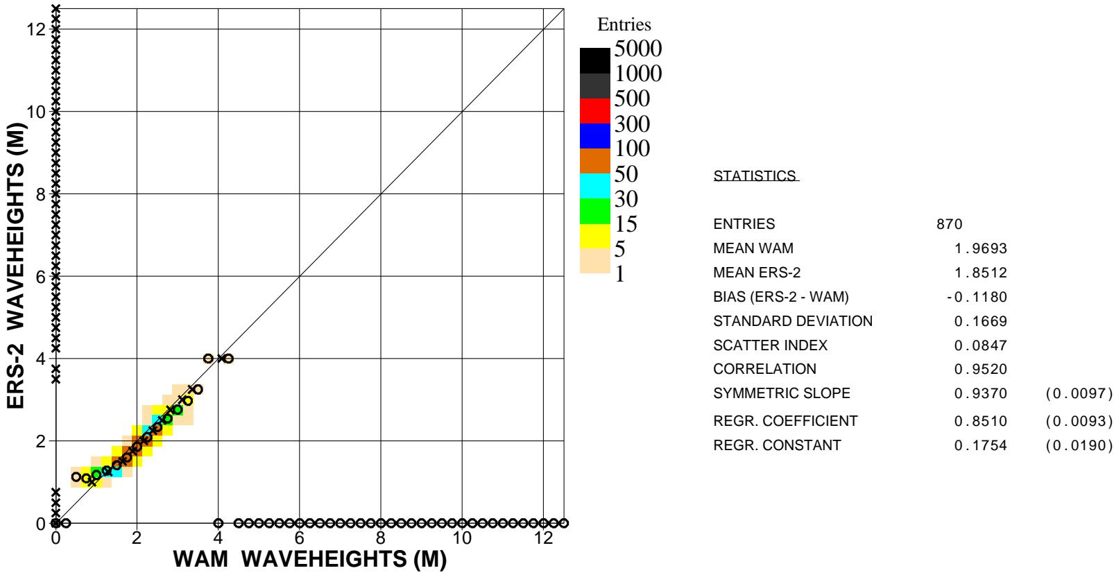
Figure 19. Comparison of ECMWF wave height results with ERS2 Altimeter wave height data for April 2008 (tropics)
