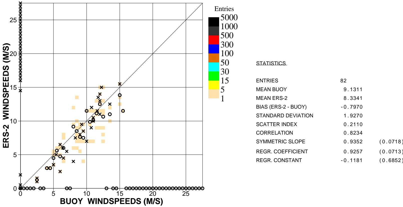
Figure 10. Comparison of buoy wind speed observations with ERS2 Altimeter wind speed data for April 2008 (global)
