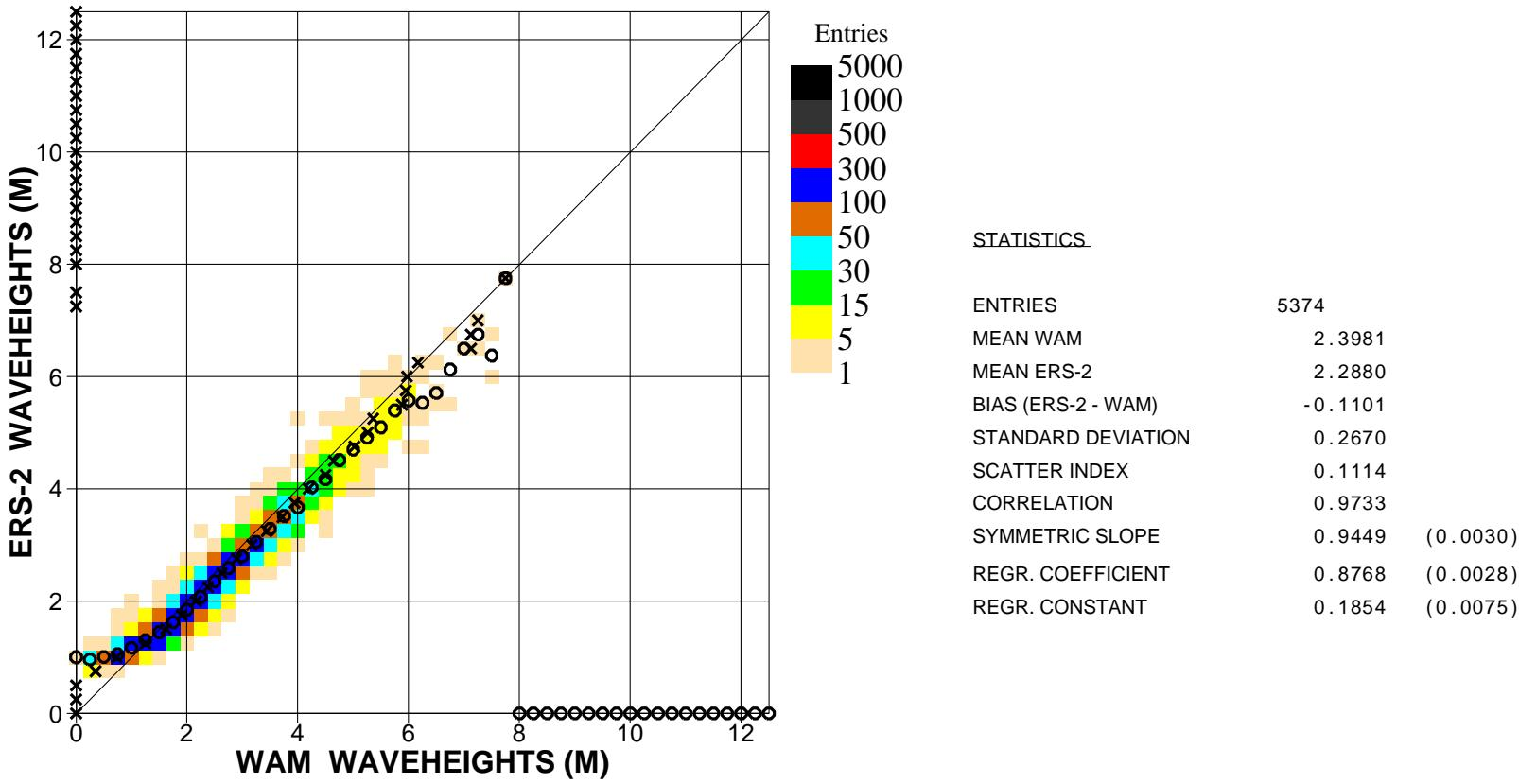
Figure 18. Comparison of ECMWF wave height results with ERS2 Altimeter wave height data for April 2008 (n.hem.)
