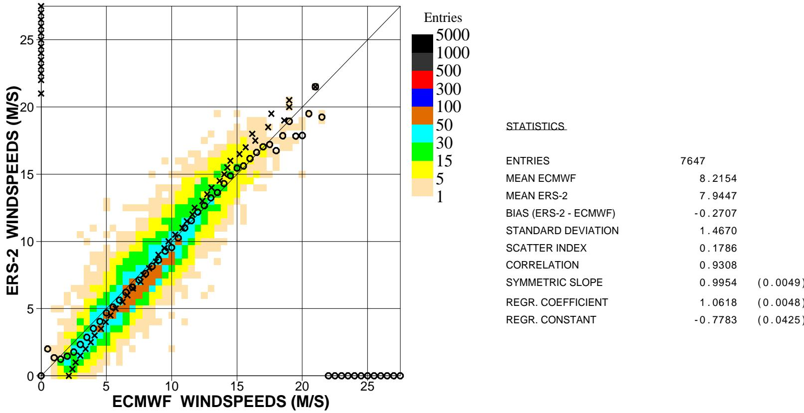
Figure 6. Comparison of ECMWF wind speed results with ERS2 Altimeter wind speed data for April 2008 (global)
