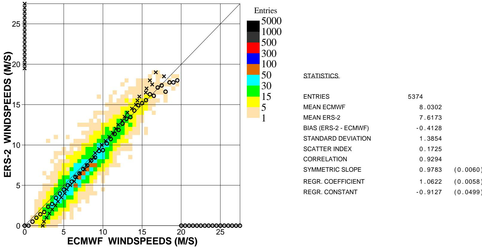
Figure 7. Comparison of ECMWF wind speed results with ERS2 Altimeter wind speed data for April 2008 (n.hem.)
