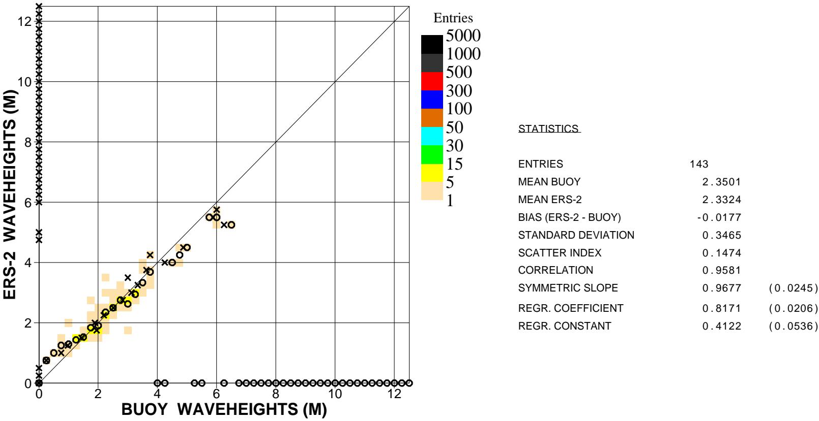
Figure 21. Comparison of buoy wave height observations with ERS2 Altimeter wave height data for April 2008 (global)
