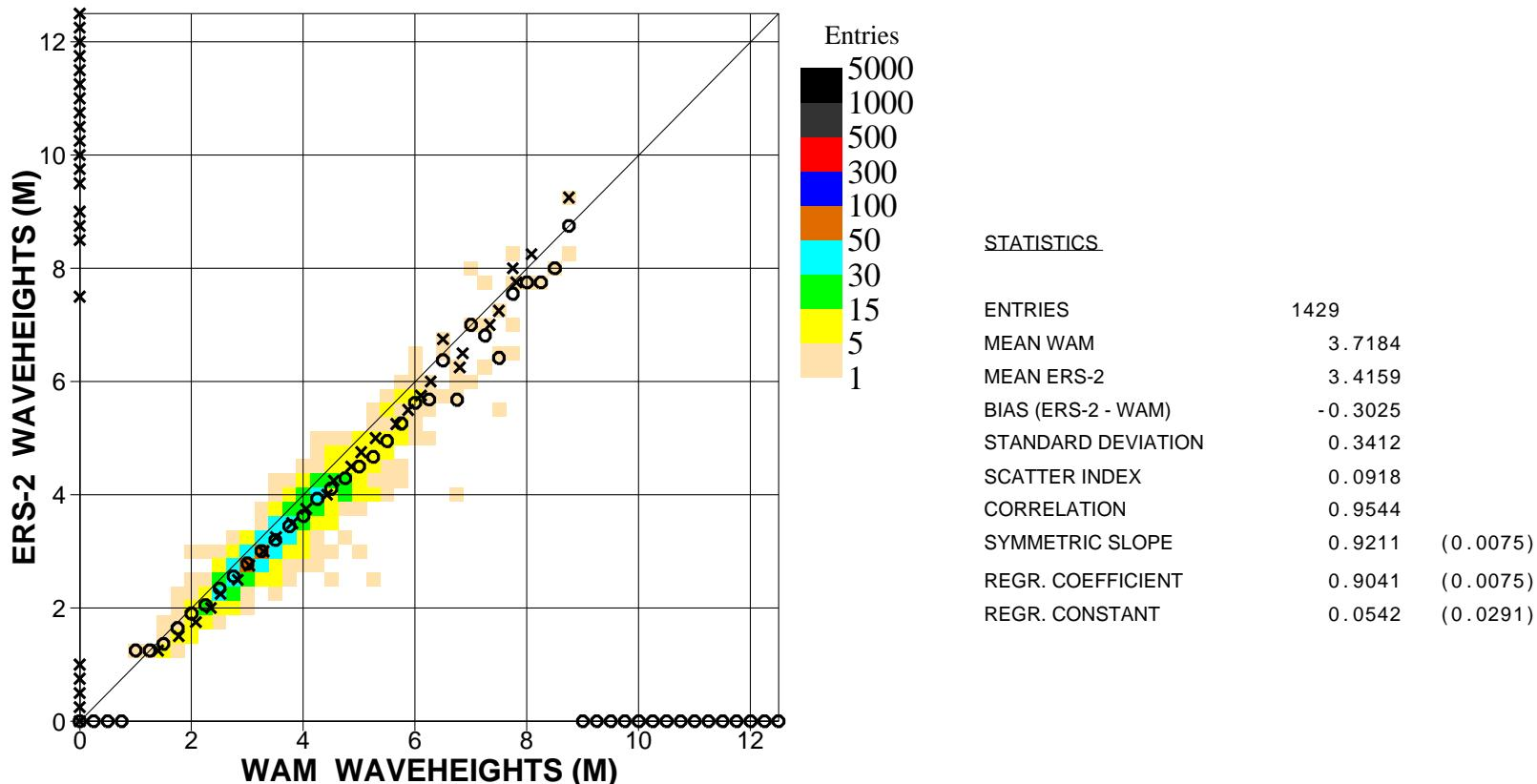
Figure 20. Comparison of ECMWF wave height results with ERS2 Altimeter wave height data for April 2008 (s.hem.)
