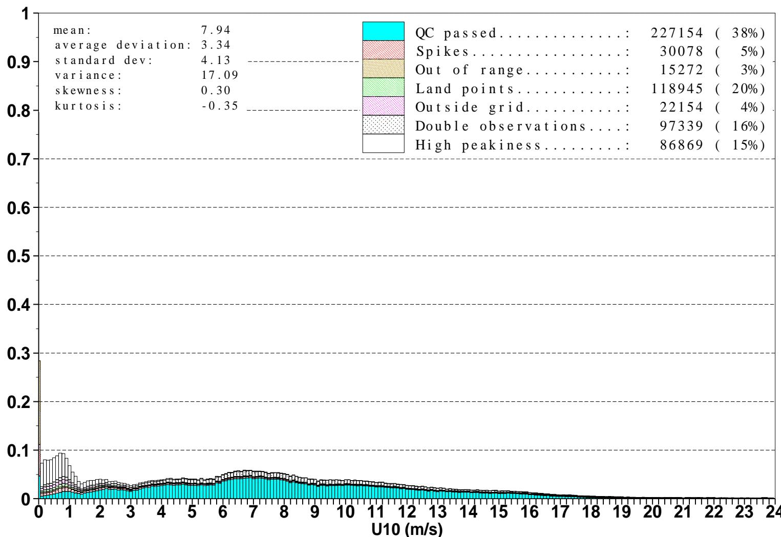
Figure 3: Distribution of the ERS-2 Altimeter wind speeds after QC for April 2008
