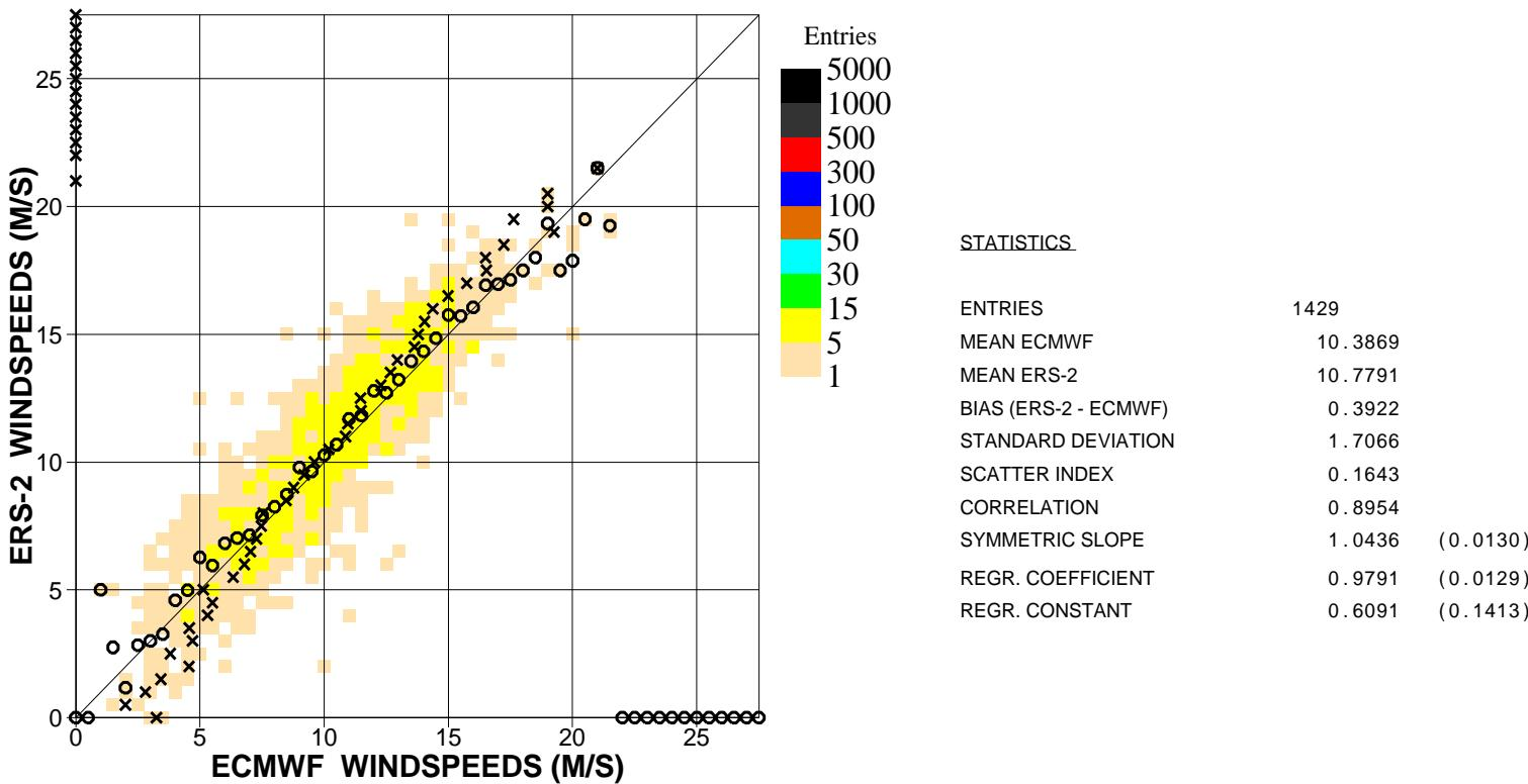
Figure 9. Comparison of ECMWF wind speed results with ERS2 Altimeter wind speed data for April 2008 (s.hem.)
