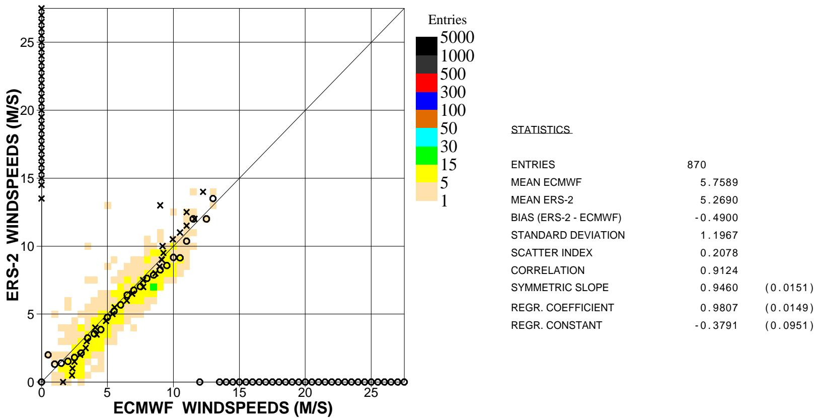
Figure 8. Comparison of ECMWF wind speed results with ERS2 Altimeter wind speed data for April 2008 (tropics)
