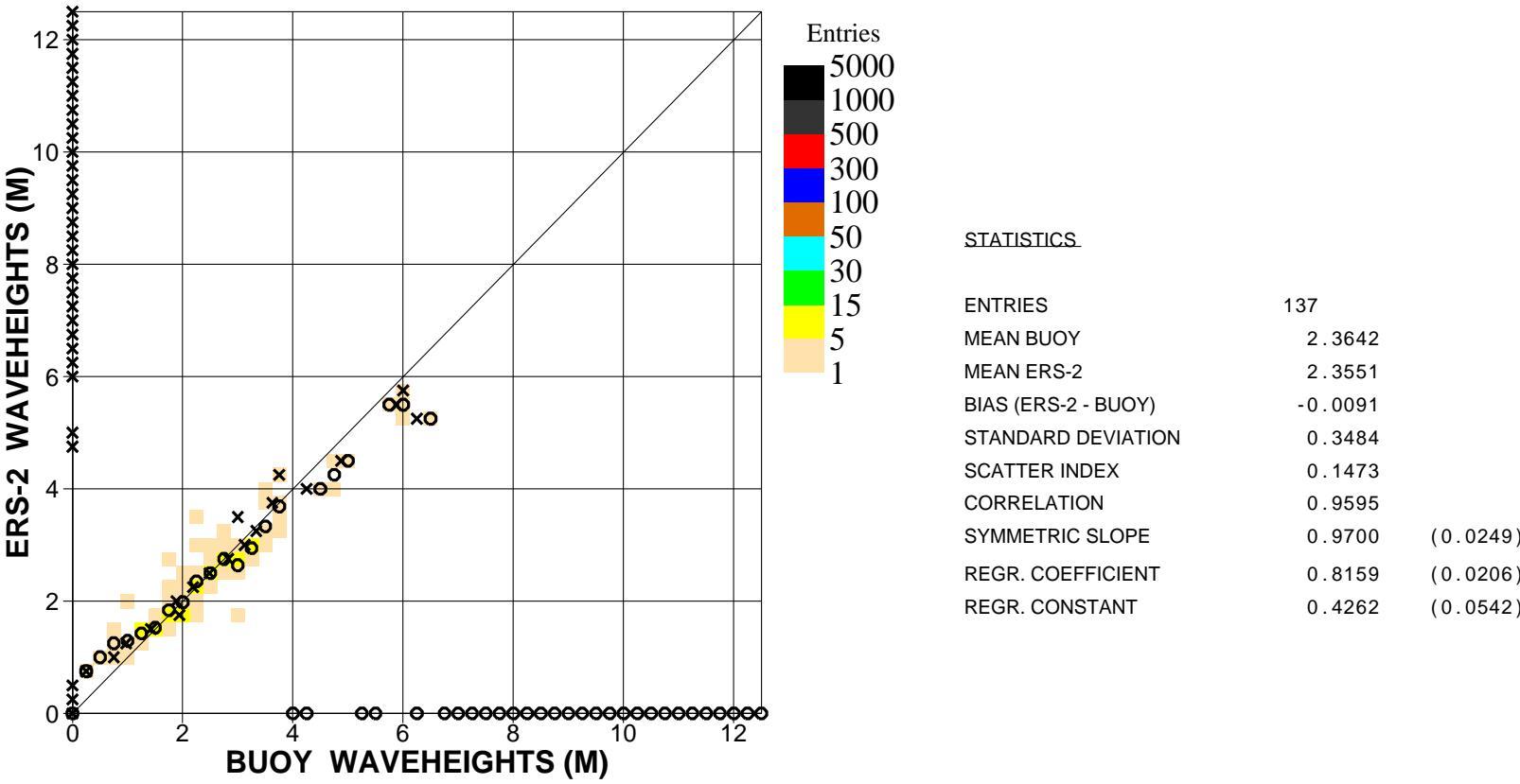
Figure 22. Comparison of buoy wave height observations with ERS2 Altimeter wave height data for April 2008 (n.hem.)
