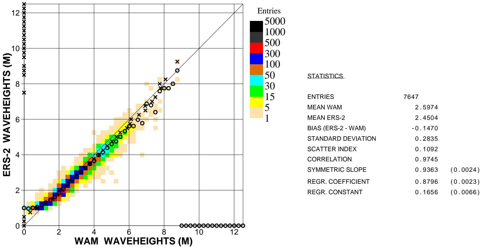
Figure 17. Comparison of ECMWF wave height results with ERS2 Altimeter wave height data for April 2008 (global)
