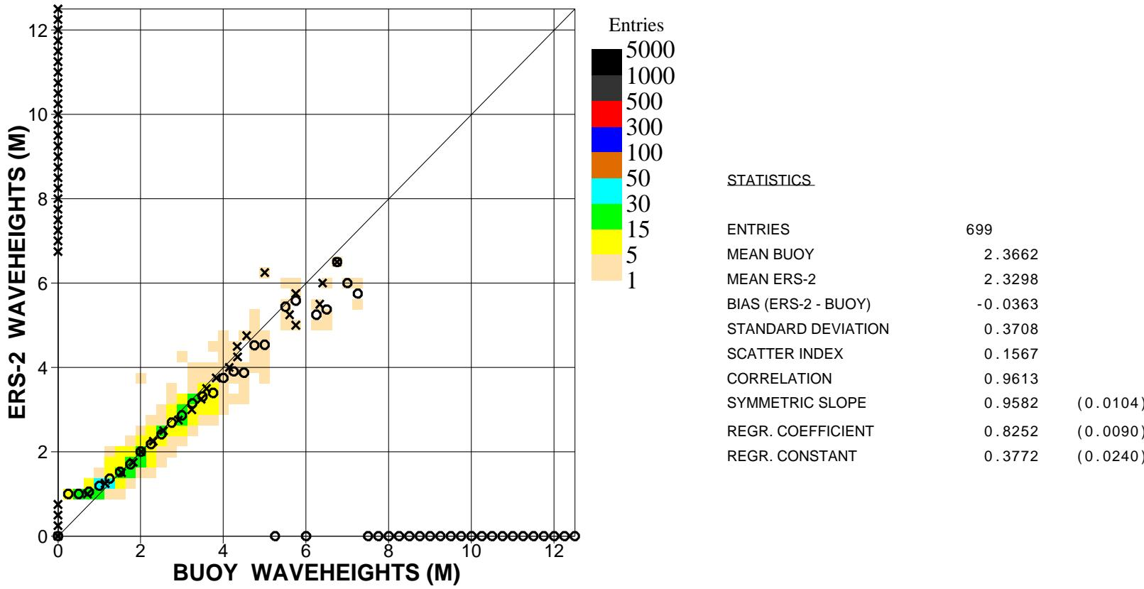
Figure 22. Comparison of buoy wave height observations with ERS2 Altimeter wave height data for April 2007 (n.hem.)
