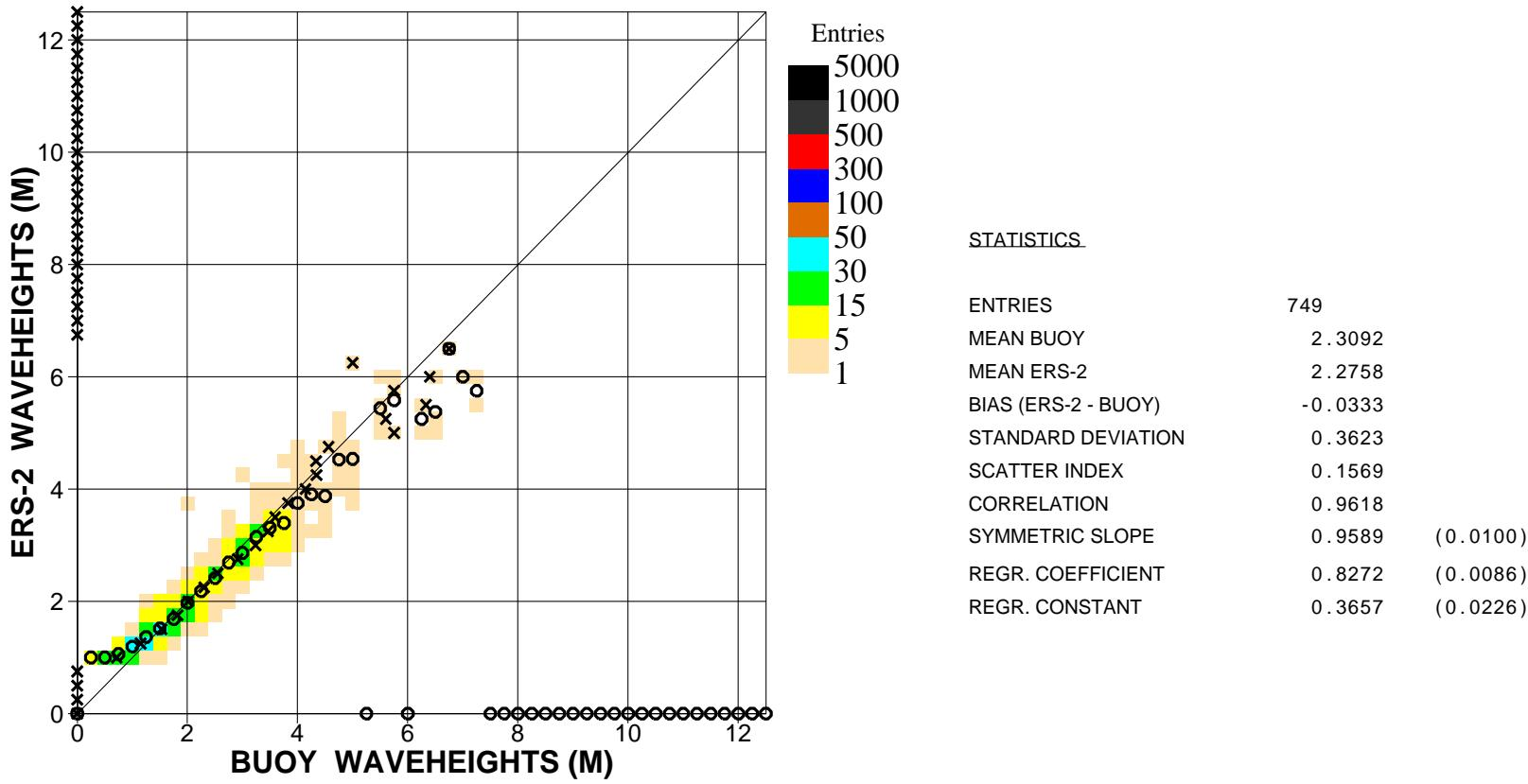
Figure 21. Comparison of buoy wave height observations with ERS2 Altimeter wave height data for April 2007 (global)
