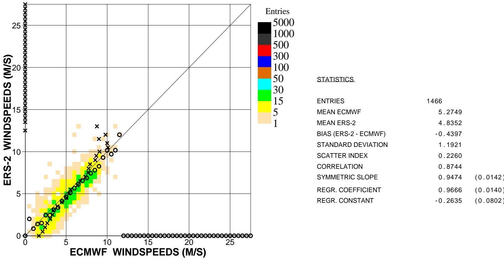
Figure 8. Comparison of ECMWF wind speed results with ERS2 Altimeter wind speed data for April 2007 (tropics)
