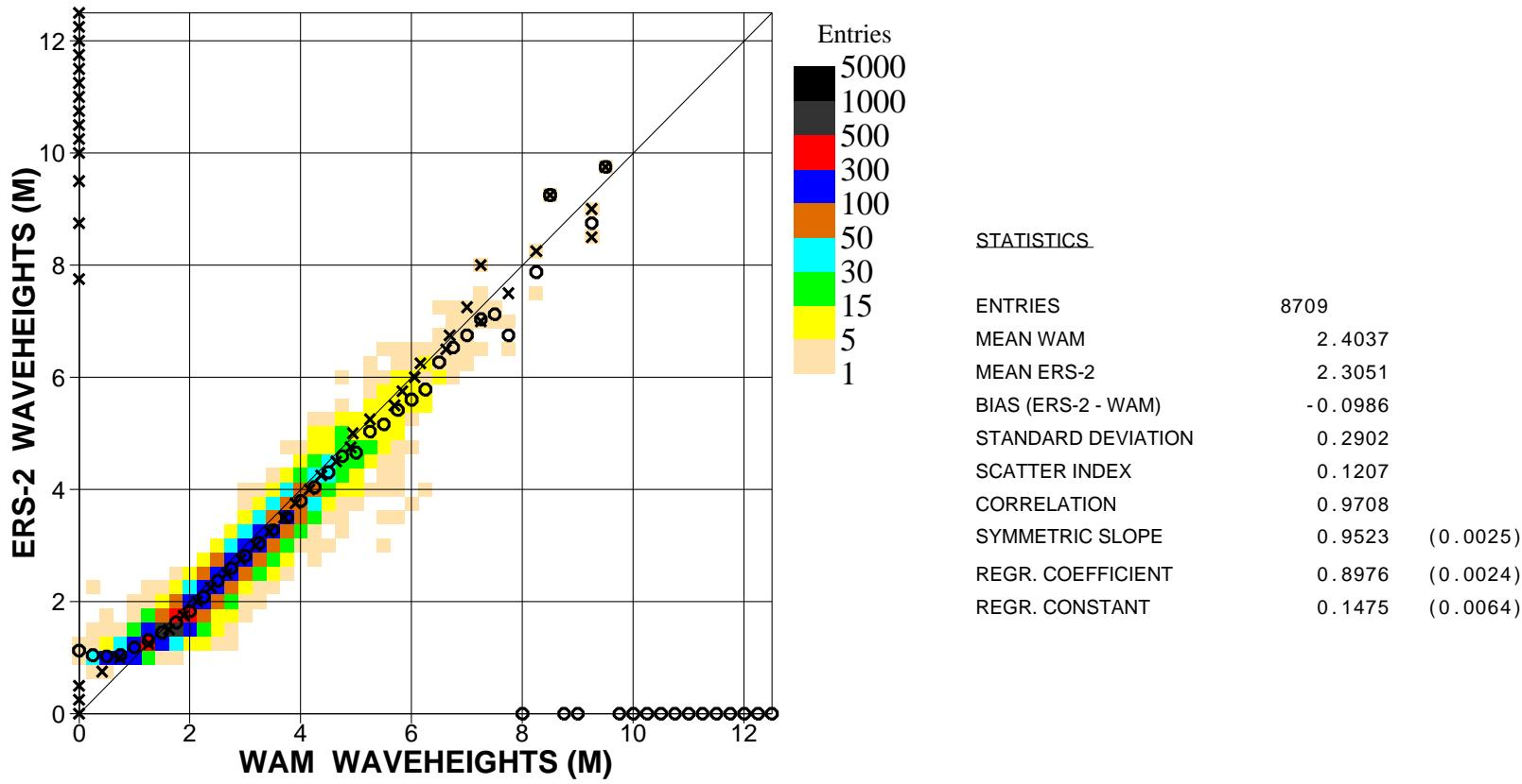
Figure 17. Comparison of ECMWF wave height results with ERS2 Altimeter wave height data for April 2007 (global)
