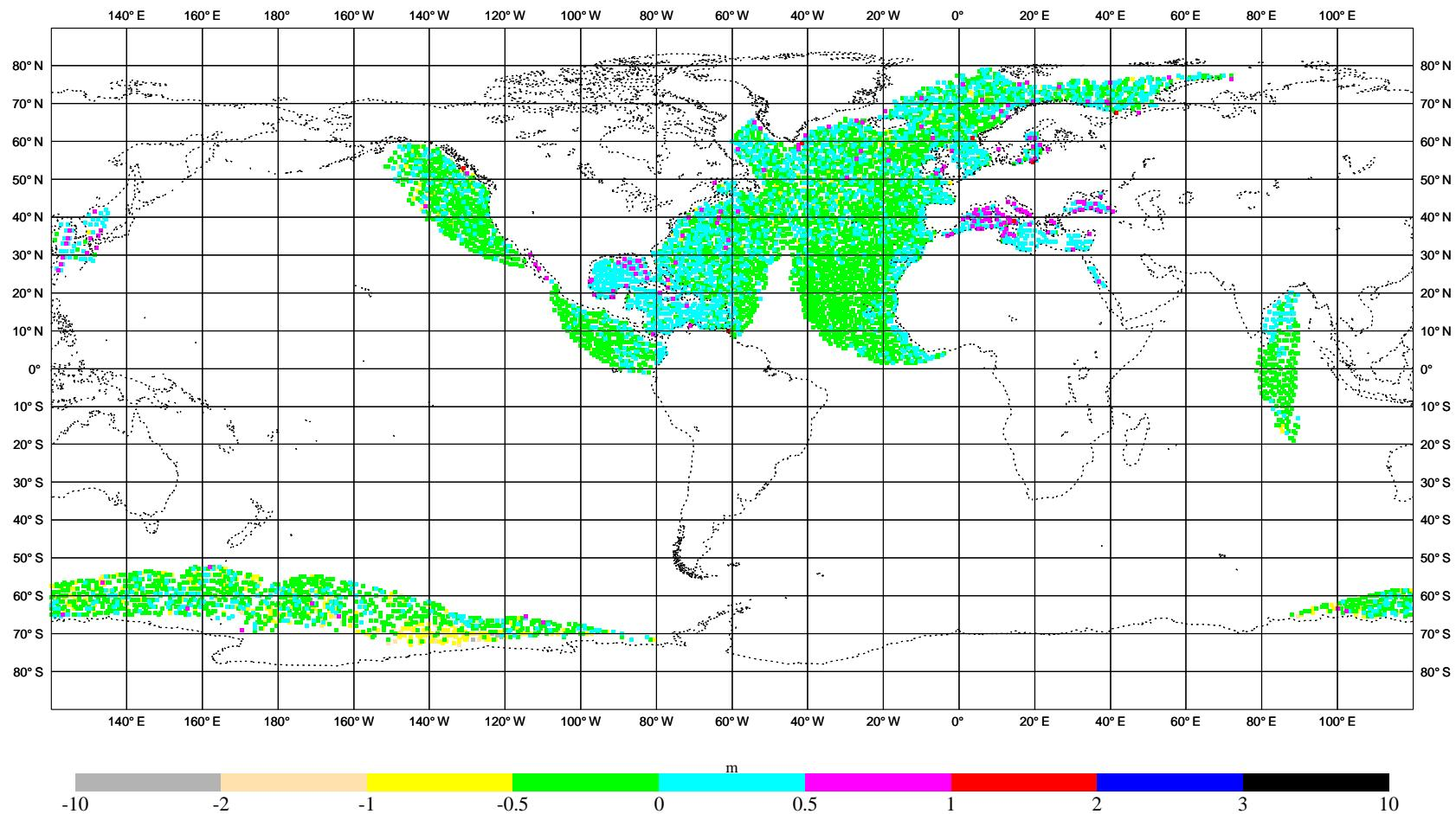
Figure 27: Significant wave height: Monthly mean difference of ERS-2 altimeter data minus wave model results for April 2007.
