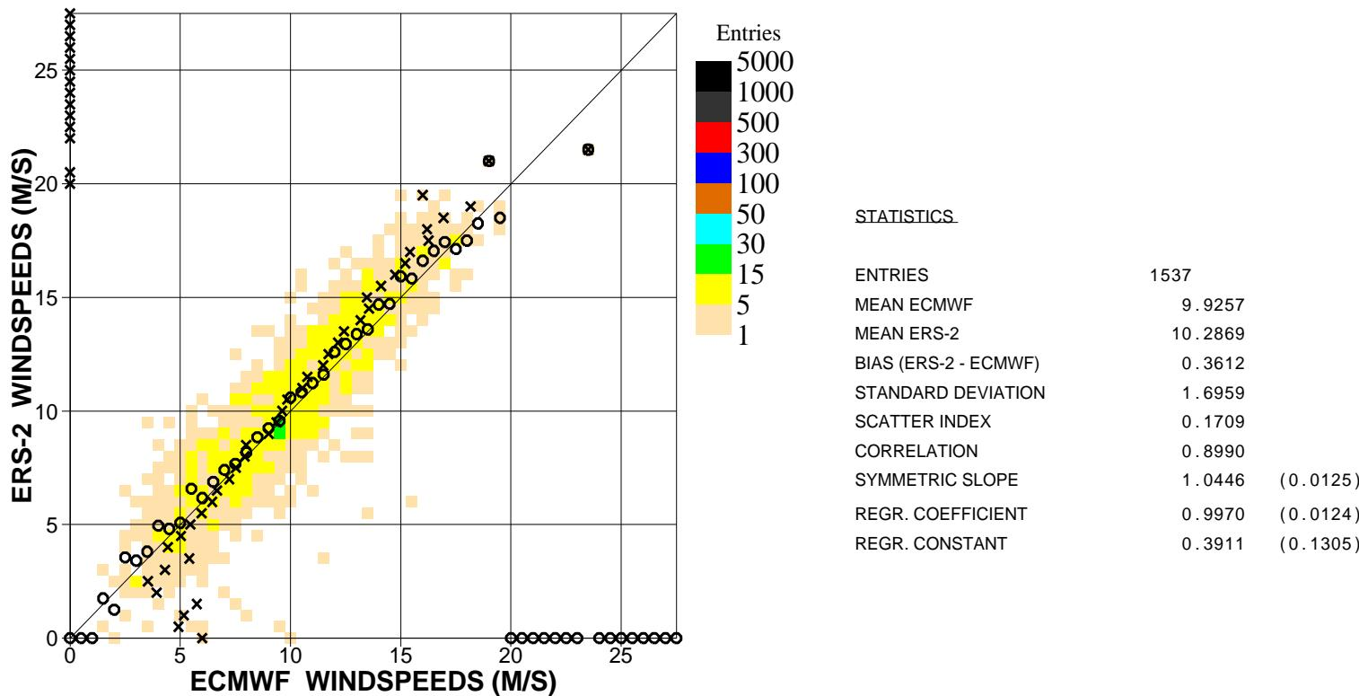
Figure 9. Comparison of ECMWF wind speed results with ERS2 Altimeter wind speed data for April 2007 (s.hem.)
