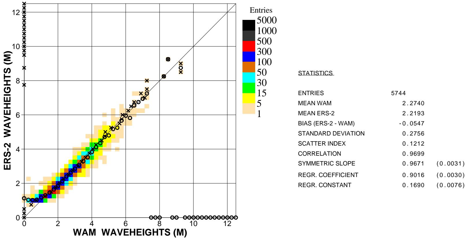
Figure 18. Comparison of ECMWF wave height results with ERS2 Altimeter wave height data for April 2007 (n.hem.)
