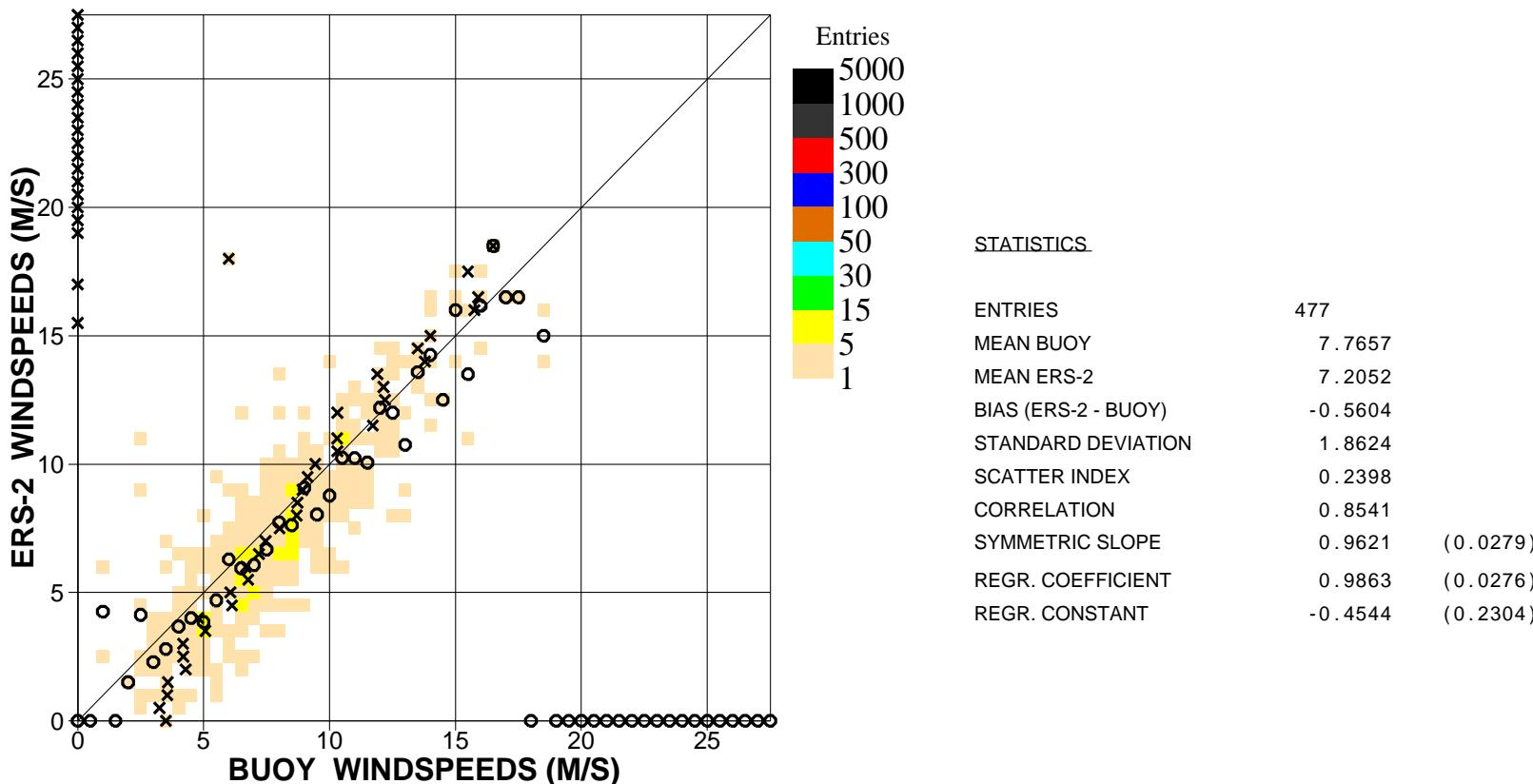
Figure 10. Comparison of buoy wind speed observations with ERS2 Altimeter wind speed data for April 2007 (global)
