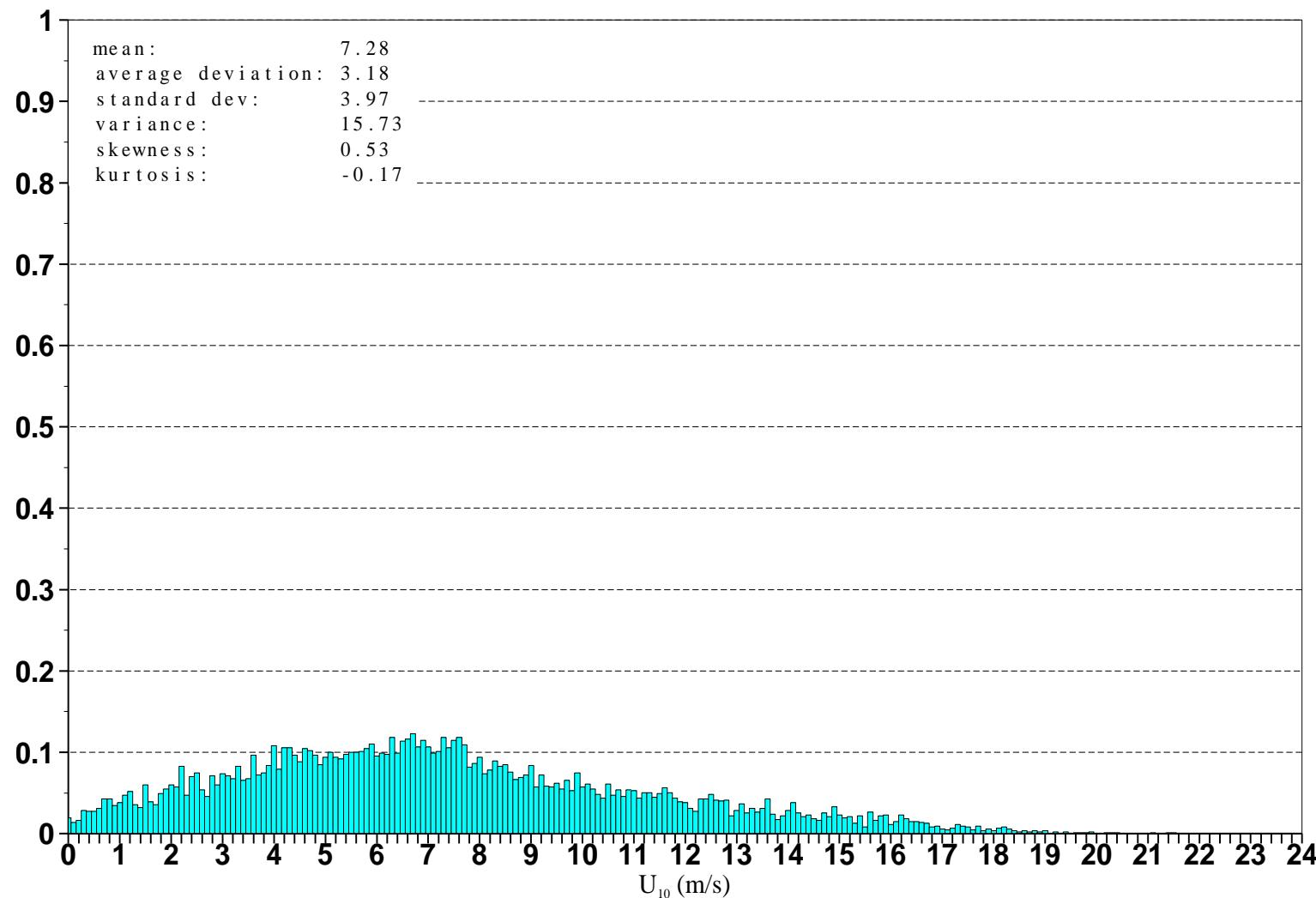
Figure 4: Distribution of ERS-2 Altimeter wind speeds after along track averaging for April 2007
