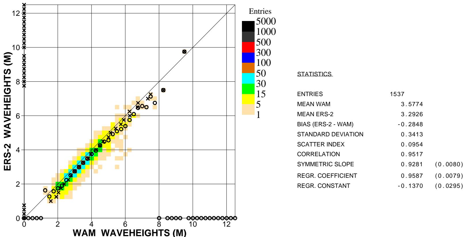
Figure 20. Comparison of ECMWF wave height results with ERS2 Altimeter wave height data for April 2007 (s.hem.)
