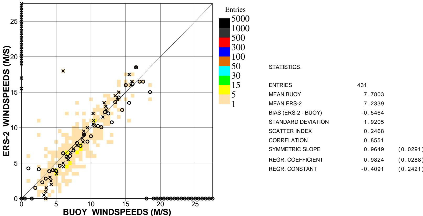
Figure 11. Comparison of buoy wind speed observations with ERS2 Altimeter wind speed data for April 2007 (n.hem.)
