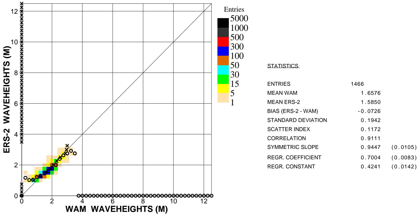
Figure 19. Comparison of ECMWF wave height results with ERS2 Altimeter wave height data for April 2007 (tropics)
