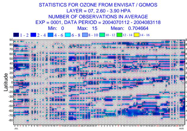
Fig. 2. Hovmoeller diagram of zonal mean number of data of ENVISAT GOMOS NRT ozone data per 6-hour cycle for July and August 2004.
