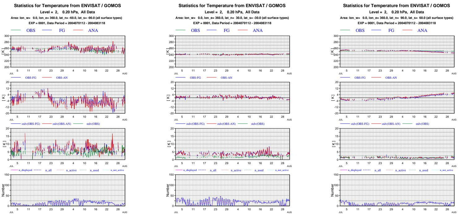
Fig. 21. Time series of mean ENVISAT GOMOS NRT temperature data, first guess and analysis values (top panel), first-guess and analysis departures (second panel), standard deviations (third panel) and number of data (bottom panel) per 6-hour cycle for level 2 (0.2 hPa) 90-60N, 30N-30S, 60-90S for July and August 2004.
