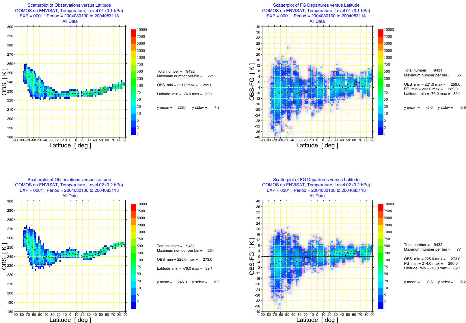
Fig. 9. Scatter plot of ENVISAT GOMOS NRT temperature data against latitude and scatter plot of first-guess departures of ENVISAT GOMOS NRT temperature data (right) against latitude for August 2004 for level 1 (0.1 hPa) and level 2 (0.2 hPa). The colours show the number of data per bin, the black dots the mean value per bin.
