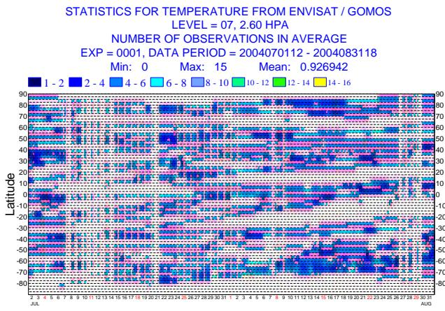
Fig. 2. Hovmoeller diagram of zonal mean number of data of ENVISAT GOMOS NRT temperature data per 6-hour cycle for July and August 2004.
