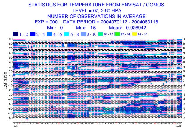
Fig. 2. Hovmöller diagram of zonal mean number of data of ENVISAT GOMOS NRT temperature data per 6-hour cycle for July and August 2004.
