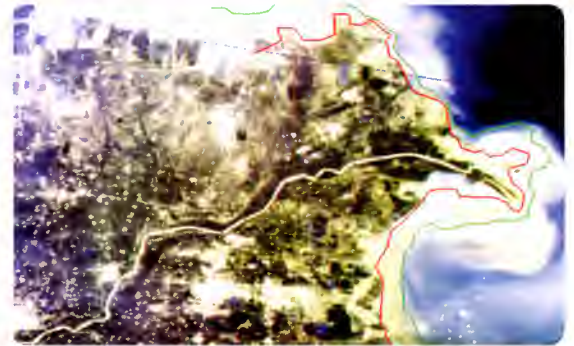
↑ Analysis of time series of optical satellite imagery allows to map the shore line (in red) and inter-tidal zone (in green) - Yellow River Delta, Bohai Sea
