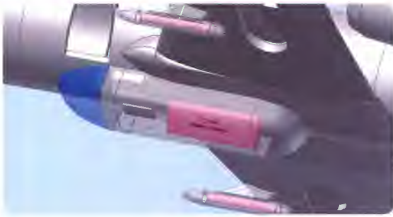
↑ Graphic shows dual frequency X/P band SARs and mounting on aircraft
