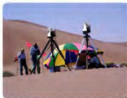
↑ Desert region – calibration of the passive microwave radiometer (GBMR)
