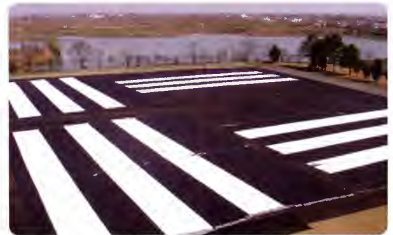
↑ In-situ calibration target, Beijing-1 Calibration Campaign in An'hui, China, March 2006. Courtesy of Beijing Landview Mapping Information Technology Co. Ltd. (BLMIT)
