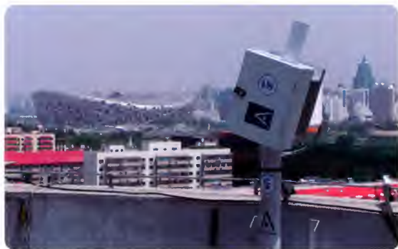
↑ MaxDOAS at Institute of Atmospheric Physics, Beijing (Bird's nest Olympic stadium in background)
