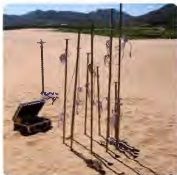
↑ Typical set-up for a desert soil moisture sampling station, multiple probes ensure reliability of measurements
