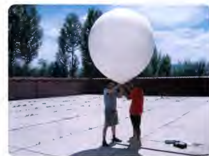
↑ Collection of atmospheric sounding data by balloon
