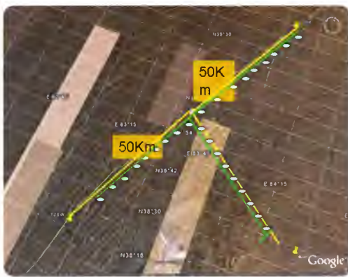
↑ Proposed layout of soil moisture sampling stations (white points) and passive microwave measurements for SMOS-MIRAS calibration during the commissioning phase Taklamakan Sand Desert reference site
