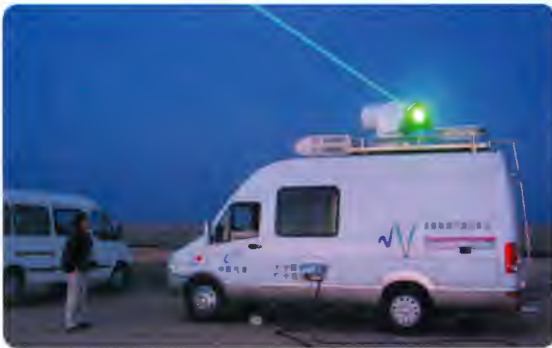
↑ Mobile Doppler wind lidar during Shenzhou 7 Spacecraft landing campaign.
