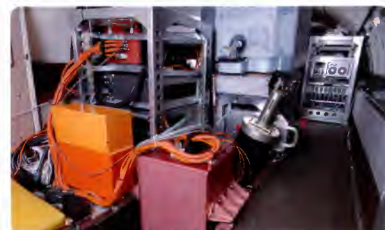
↑ The 2-µm wind lidar (front) and the ADM-Aeolus prototype (back) wind lidar installed in the DLR Falcon 20 aircraft.
