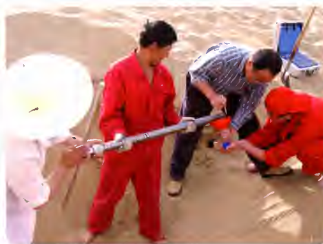
↑ Soil moisture probes being placed in the desert
