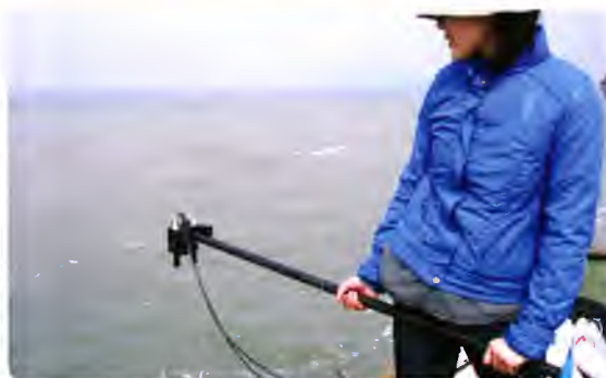
↑ Water reflectance of Lake Taihu measured with an ASD Field Spec FR spectroradiometer (Courtesy of Hongtao Duan, NIGLAS, CAS)
