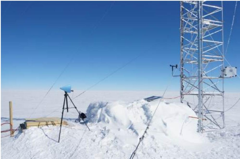
Figure 6. Location and directions of the RFI measurements (top) and measurement setup below the US tower (bottom).
