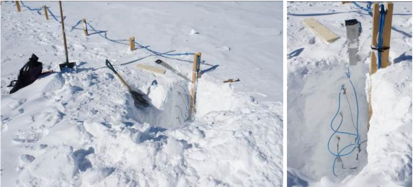
**Figure 2.** The snow pit in which are located the snow temperature probes (left) after the re-alignment to their nominal depth. The image on the right shows a particular of the probes.
