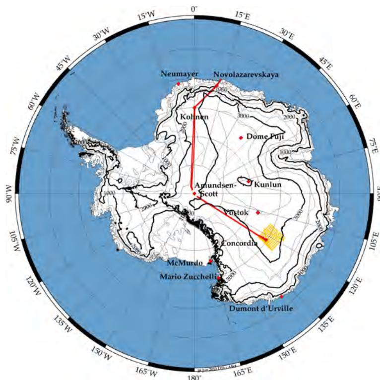
Figure 1: Overview on all DOMECAir 2013 flight, yellow lines represent the survey profiles, red lines the transit legs.
