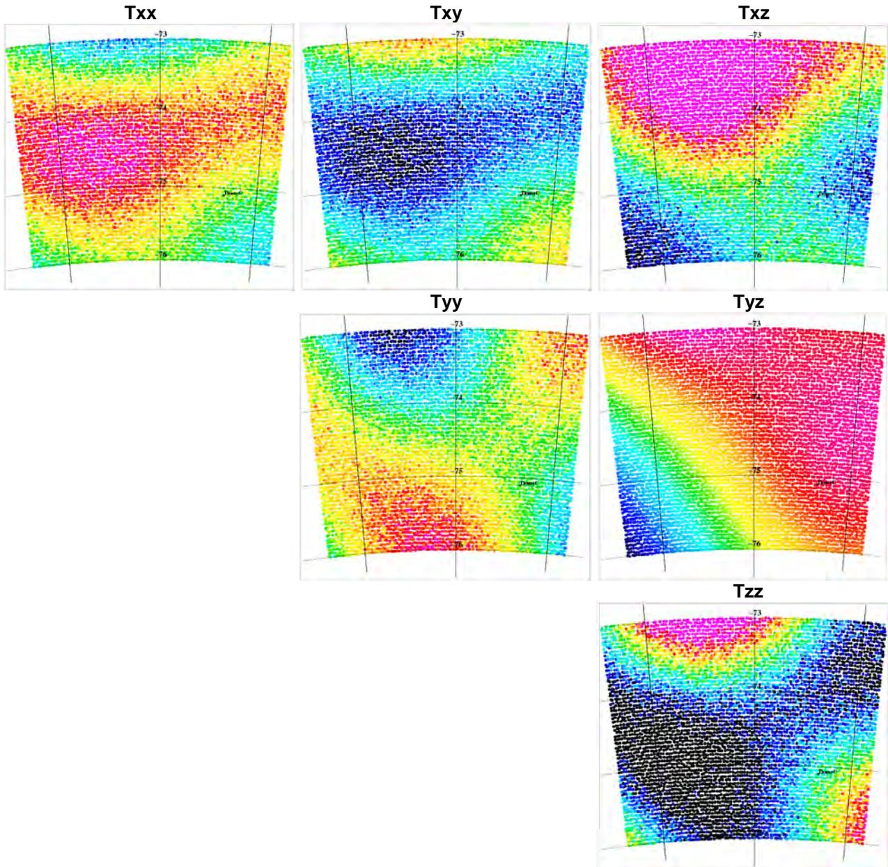
*Fig 11. Predicted gradients at GOCE points, minus EGM08 to degree 60. Colour scale is -0.08 to 0.08 Eotvos (except for the “weak” Tyz component, cf. Table 2)*
