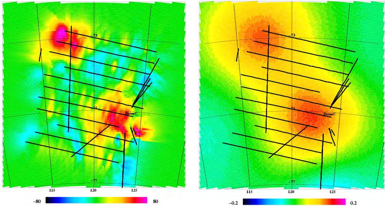
Fig. 7. Gravity anomalies minus EGM08 to degree 60 (left, mGal) and similar  $T_{zz}$  values minus EGM08 at 250 km (right, Eotvos units).
