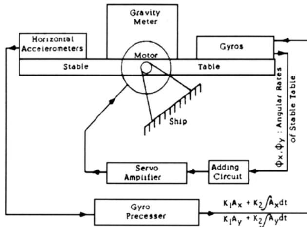
Fig. 1. Principle of the gyrostabilized platform for the LCR gravimeter. From Valiant (1991)
