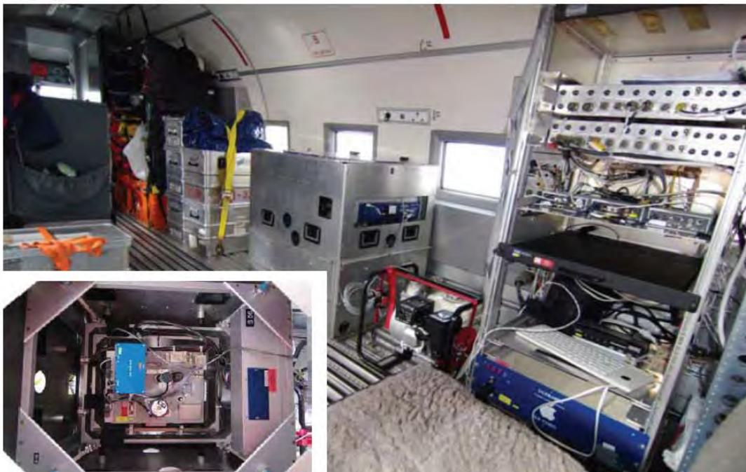
*Fig. 16. Gravimeter installation in crash-proof box in the Polar-6 (center of image). The image insert lower left shows the Lacoste and Romberg air-sea gravimeter, with gyrostabilized platform gimbals and gyros and accelerometers mounted outside the inner housing, carrying the ultrasensitive zero-length spring sensor.*
