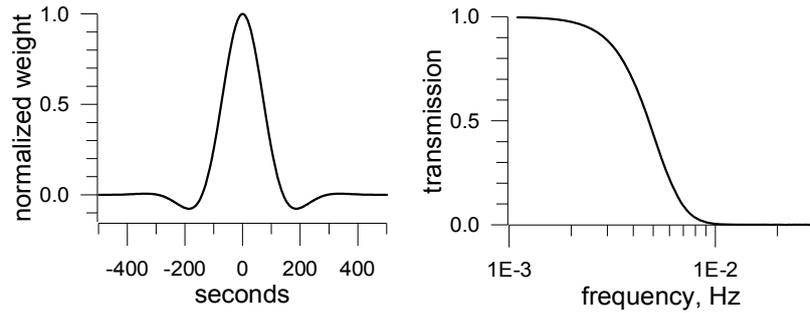
Fig. 2b. Example of the space domain (left) and frequency domain (right) filter applied in the aerogravity processing scheme of Fig 2a in rough turbulent conditions (impulse response of a triple forward/backward Butterworth filter, time constant 200 sec). All quantities in Fig. 2a are consistently along track filtered.
