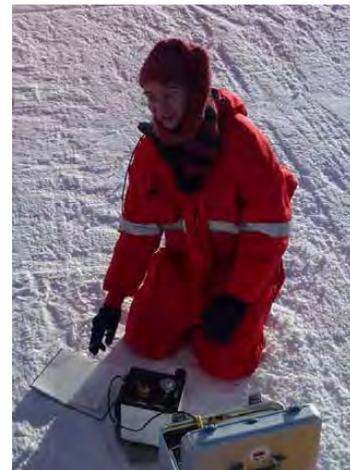
*Fig. 17. Portable gravimeter base readings at South Pole station - gravity ties from the aircraft parking positions to gravity refence networks based on absolute measurements is an essential part of aerogravity.*
