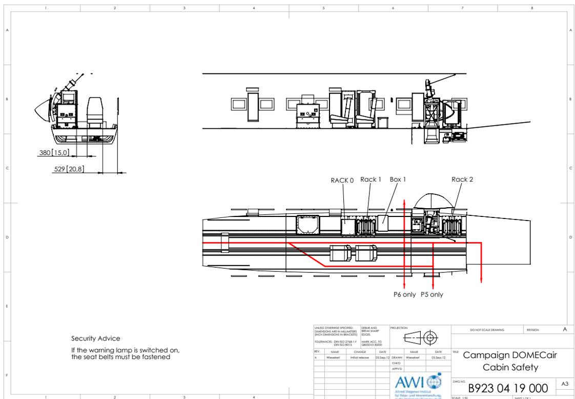
Figure 2: (a) Aircraft configuration. The drawing shows more instruments than were mounted during the survey;(b) cabin layout *POLAR 6* for the DOMEair configuration.
