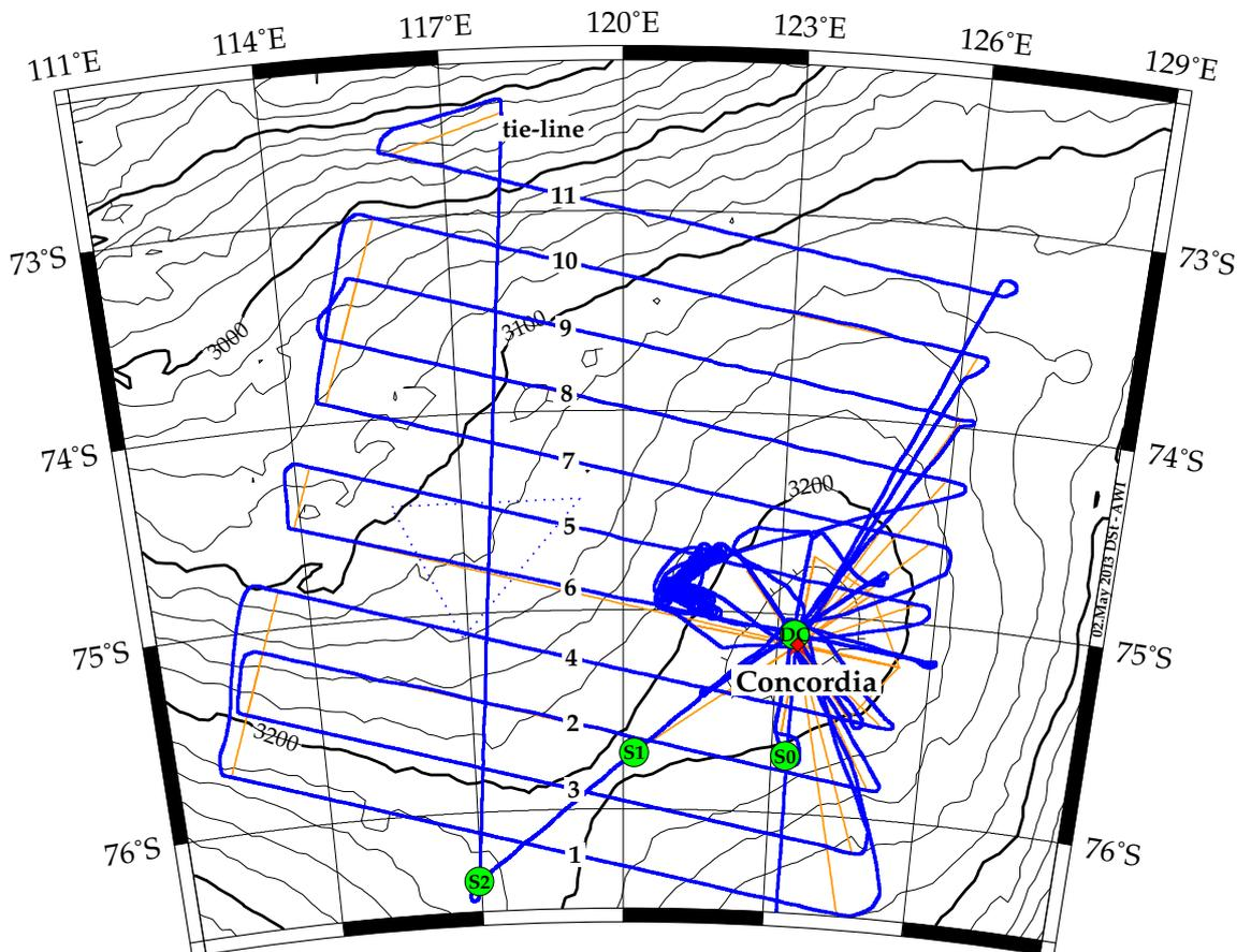
Figure 22: Map showing the actual flown tracks (blue lines) on top of planned pattern (yellow lines). The green dots indicate positions of glaciological fieldwork by Ghislain Picard et al.. The blue patches west von Concordia show the location of the two circle flights.
