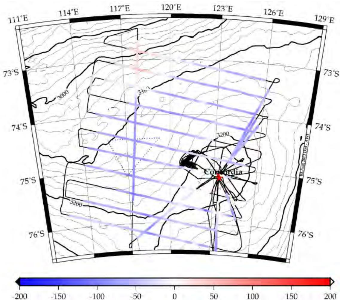
Fig. 3. Final Dome-C gravity disturbances, as processed by AWI, on top of flight lines. Units: mGal.
