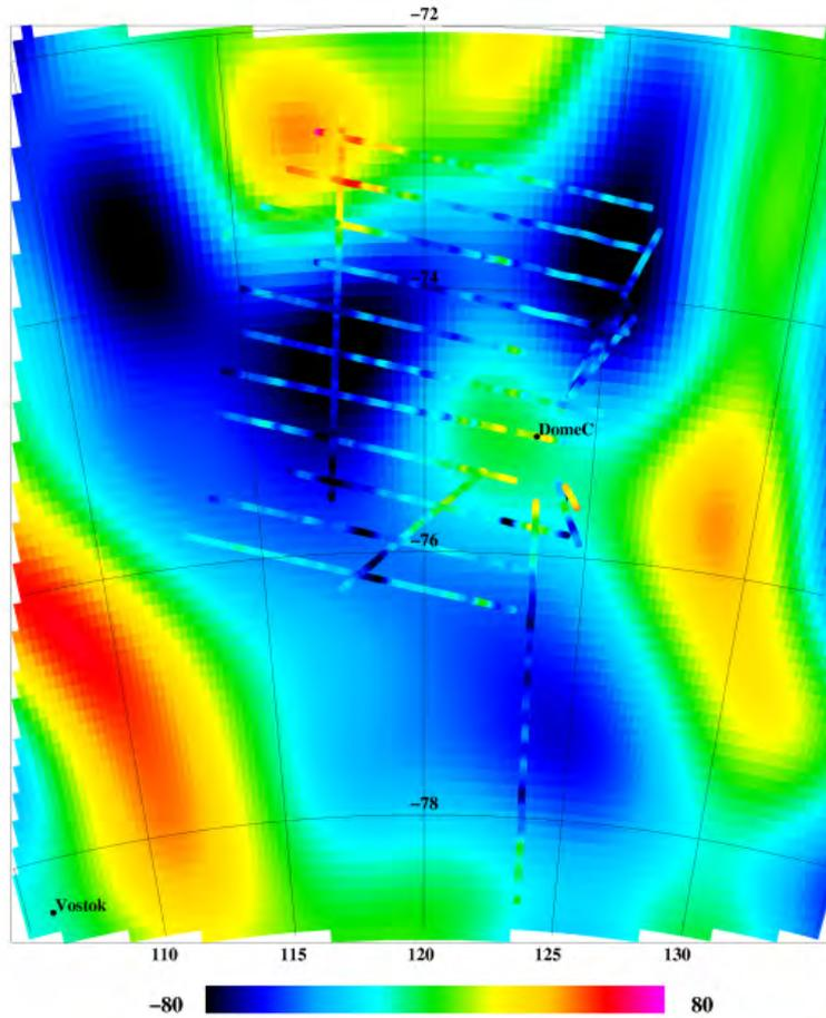
*Fig. 6. Airborne gravity free-air anomalies and GOCE RL4 “direct” to degree 200. Colour scale in mGal.*
