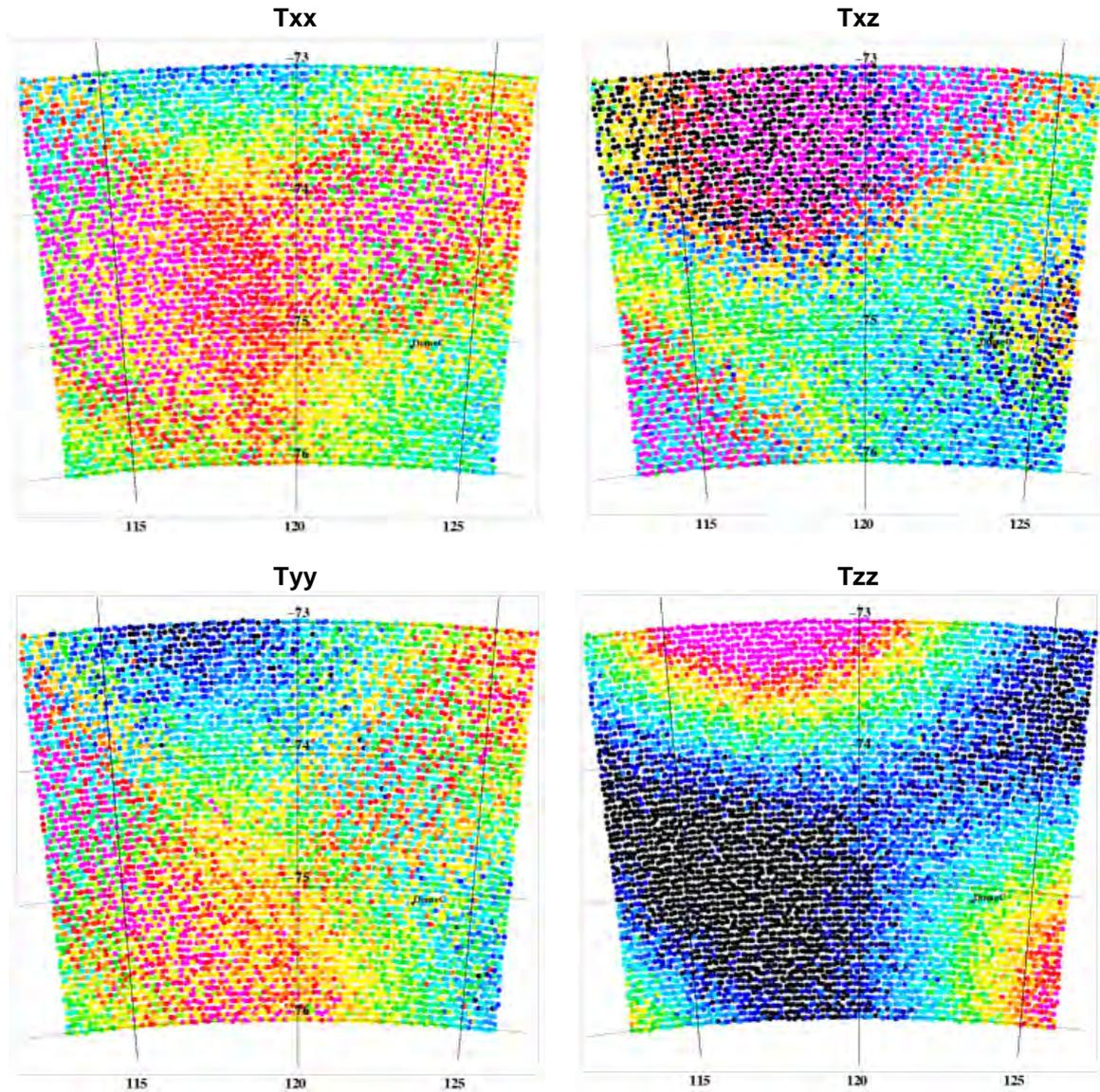
*Fig. 14. Predicted gradients at GOCE points, minus ITG-GRACE10S to degree 60. Colour scale -0.08 to 0.08 Eotvos. The noisy appearance of the data is due to the different heights of the selected GOCE data.*
