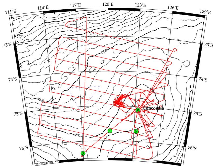
**Figure 3:** Map showing the coverage of the profiles with processed airborne laser scanner data. The underlying digital elevation model (RAMP V2) is taken from Liu et al., 2001.
