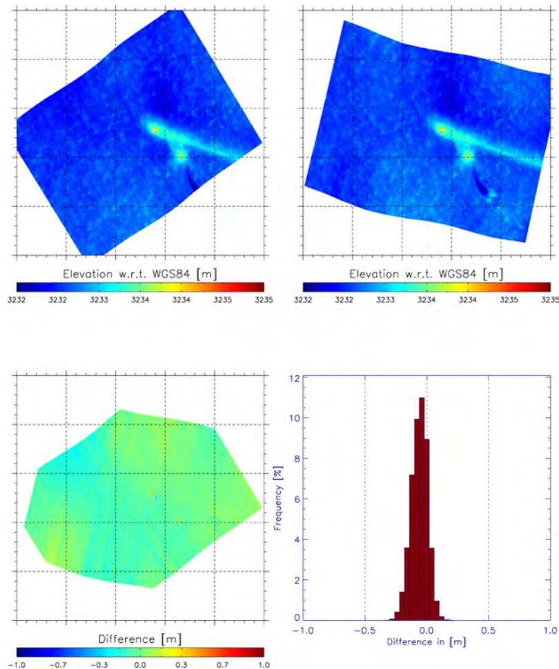
**Figure 2:** The upper line shows two geocoded segments of recorded ALS data of the star pattern, lower left shows the difference in elevation between both data sets after calibration, the lower right the associated histogram of the elevation differences.
