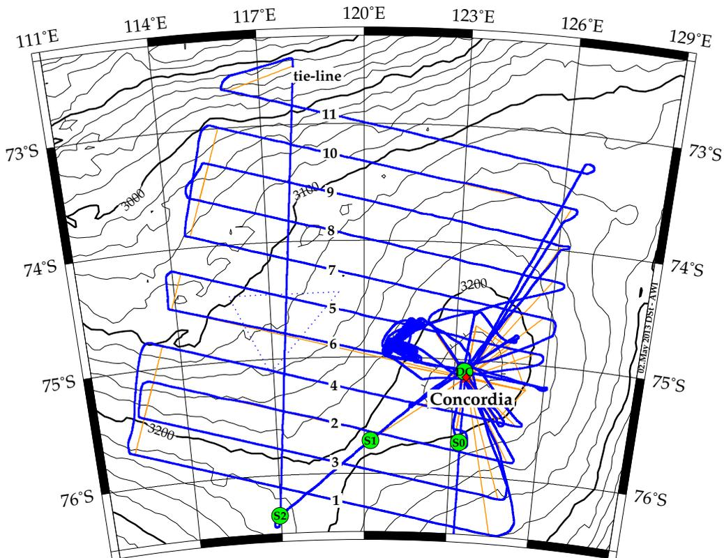
**Figure 1:** Flown profiles of the DOMCAir 2013 survey. The line spacing the parallel is 30 km, the length of lines is 300 km.
