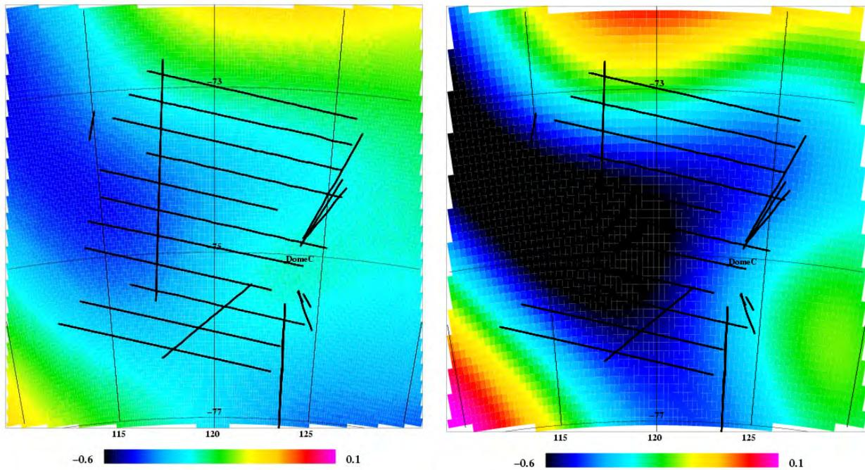
Fig. 8. Estimated  $T_{zz}$  values at 250 km, and the  $T_{zz}$  values from GOCE RL4 (Eotvos units). Large anomalies outside the survey region are evident from Fig. 6, and therefore the predicted  $T_{zz}$  values are underestimated.
