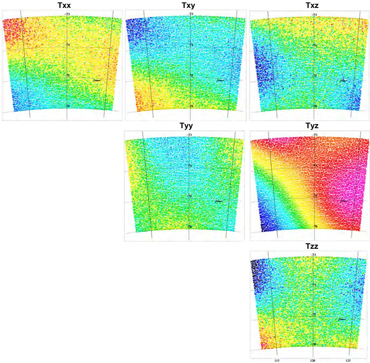
Fig 12. Difference between GOCE gradients and predictions. Colour scale -0.08 to 0.08 Eotvos (except  $T_{yz}$ )
