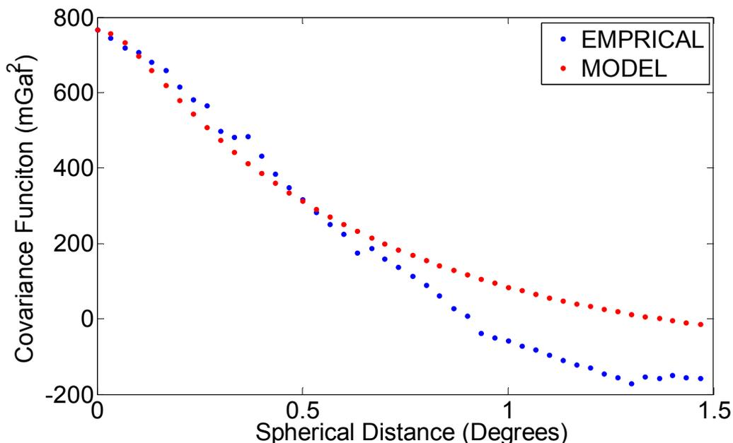
Fig. 9. The empirical covariance function (blue) derived from the airborne gravity data, and the corresponding fitted analytical Tscherning-Rapp covariance model (red). This is typical of a good fit.
