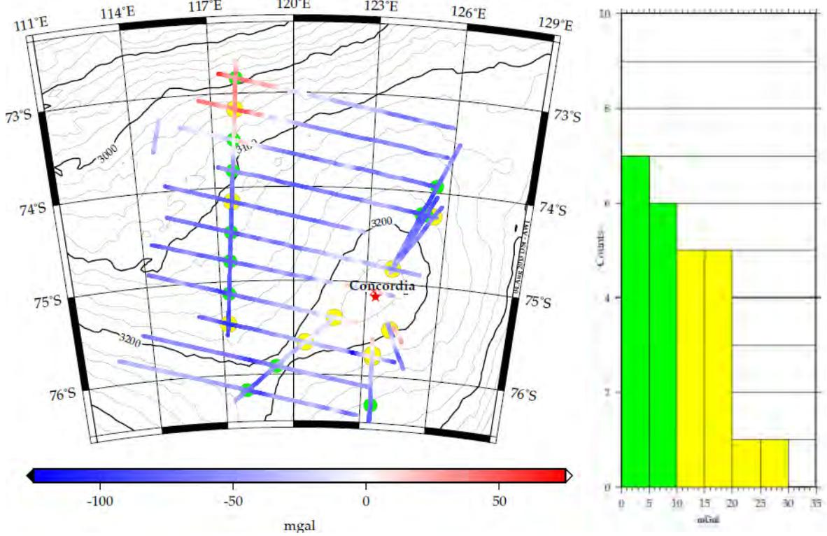
Fig. 4. Cross-over errors in the AWI-processed gravity anomalies of Dome C (left), and the histogram of the absolute value of the track misties (right; green are “good” and yellow “bad” x-overs relative to 10 mgal). The estimated r.m.s. error of the AWI-processed airborne survey, based on the x-over analysis, is 8.0 mGal.
