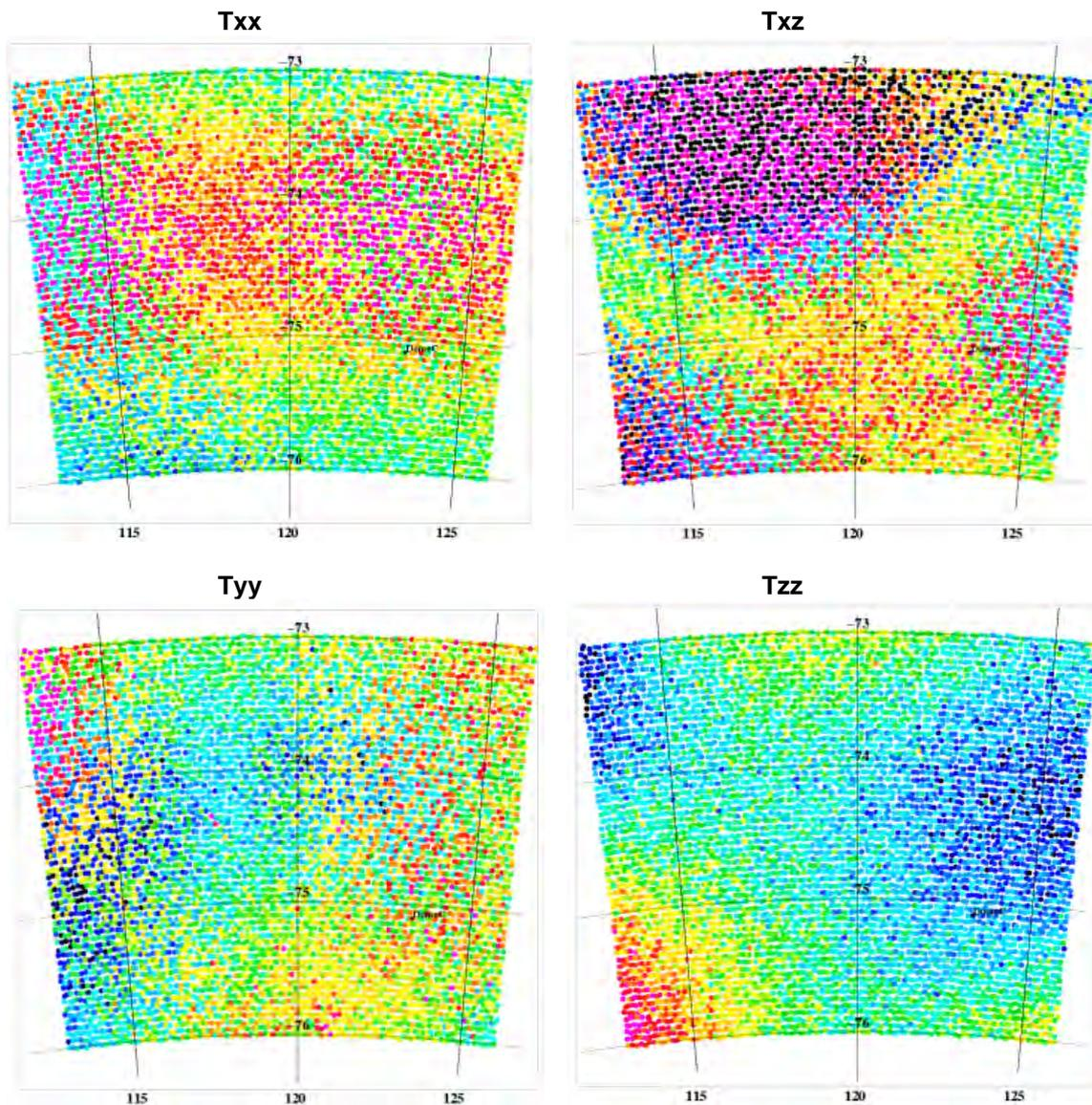
Fig. 15. Difference between GOCE gradients and predictions. Colour scale is -0.08 to 0.08 Eotvos.
