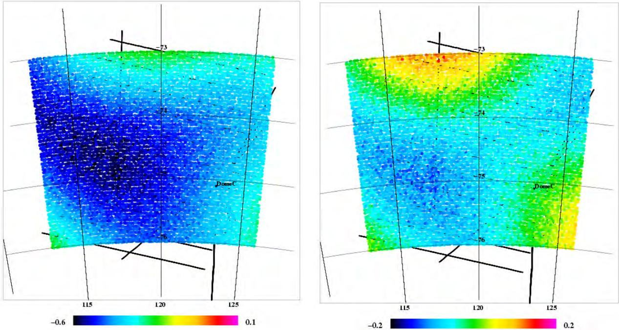
Fig. 11. Example of the role of subtracting the EGM08 (degree 60) reference field. Left: GOCE  $T_{zz}$  gradient anomaly observation points, colour scale as Fig. 8. Right: GOCE  $T_{zz}$  data minus EGM08 (to degree 60) reference field. Units: Eotvos. The “noise” is due to the different elevations.
