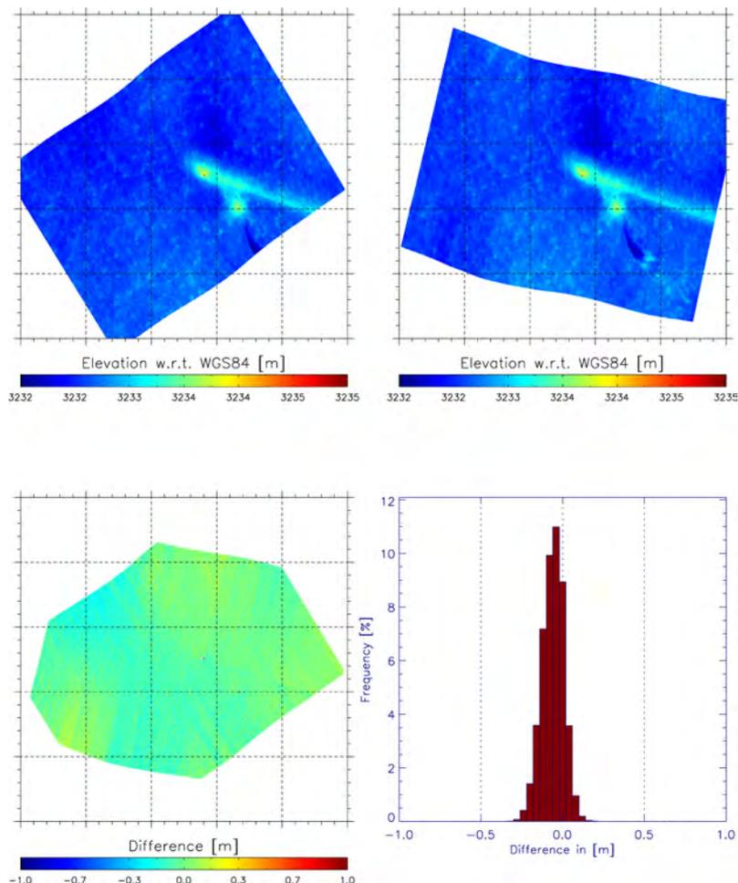
Figure 20: The upper line shows two geocoded segments of recorded ALS data of the star pattern, lower left shows the difference in elevation between both data sets after calibration, the lower right the associated histogram of the elevation differences.
