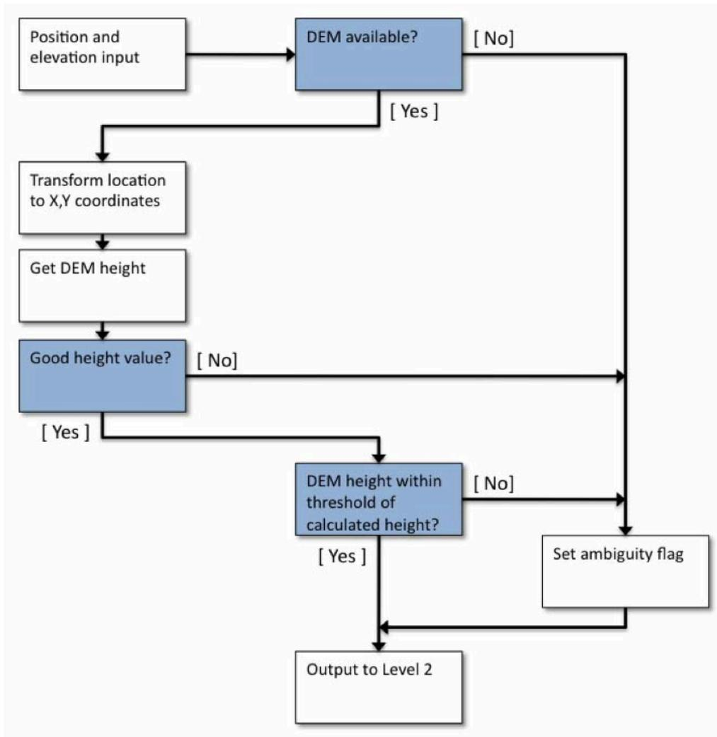
Figure 20: Ambiguity check logic for SARin
