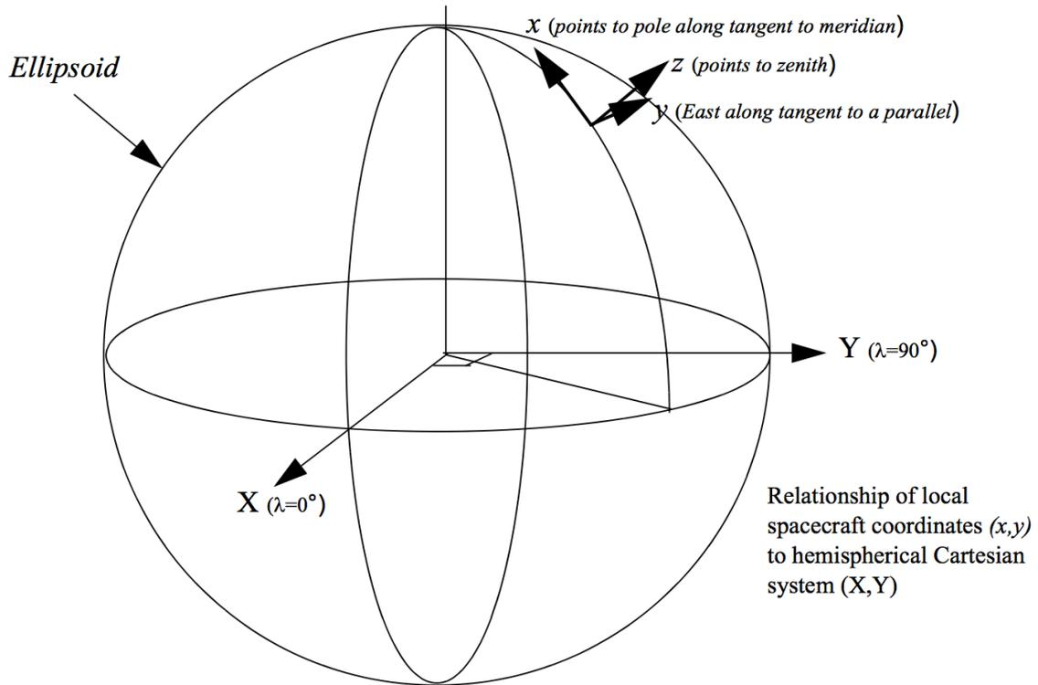
**Figure 6: Coordinate systems for the slope model correction**
