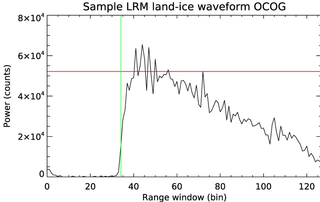
Figure 5: Example of an OCOG retrack on a land-ice echo in LRM mode
