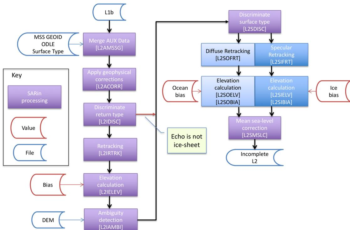
Figure 11: The SARin processing chain block diagram
