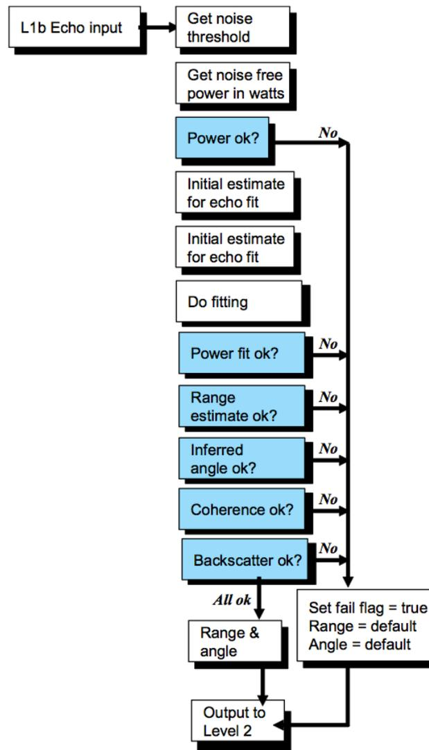
Figure 15: Echo analysis ('retracking') processing flow
