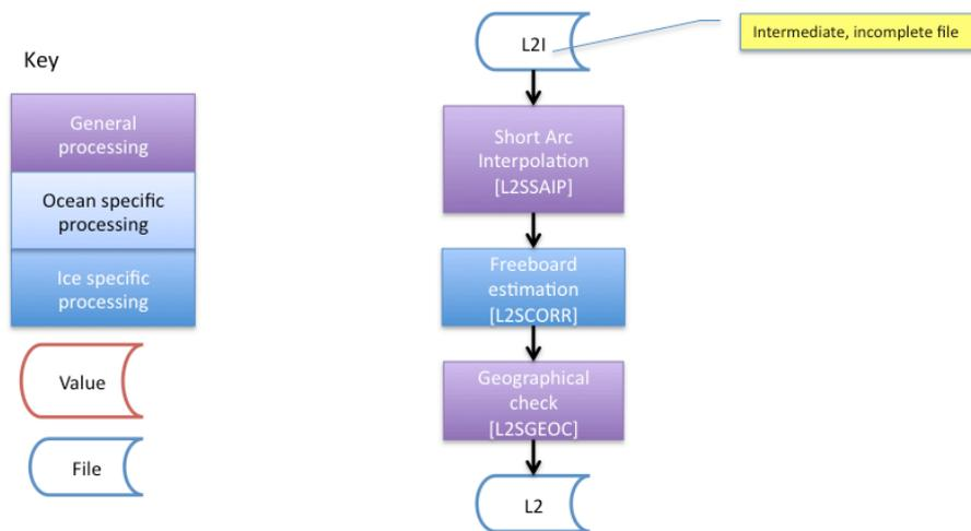
**Figure 8: The SAR/SARin sea-ice pass B processing chain**
