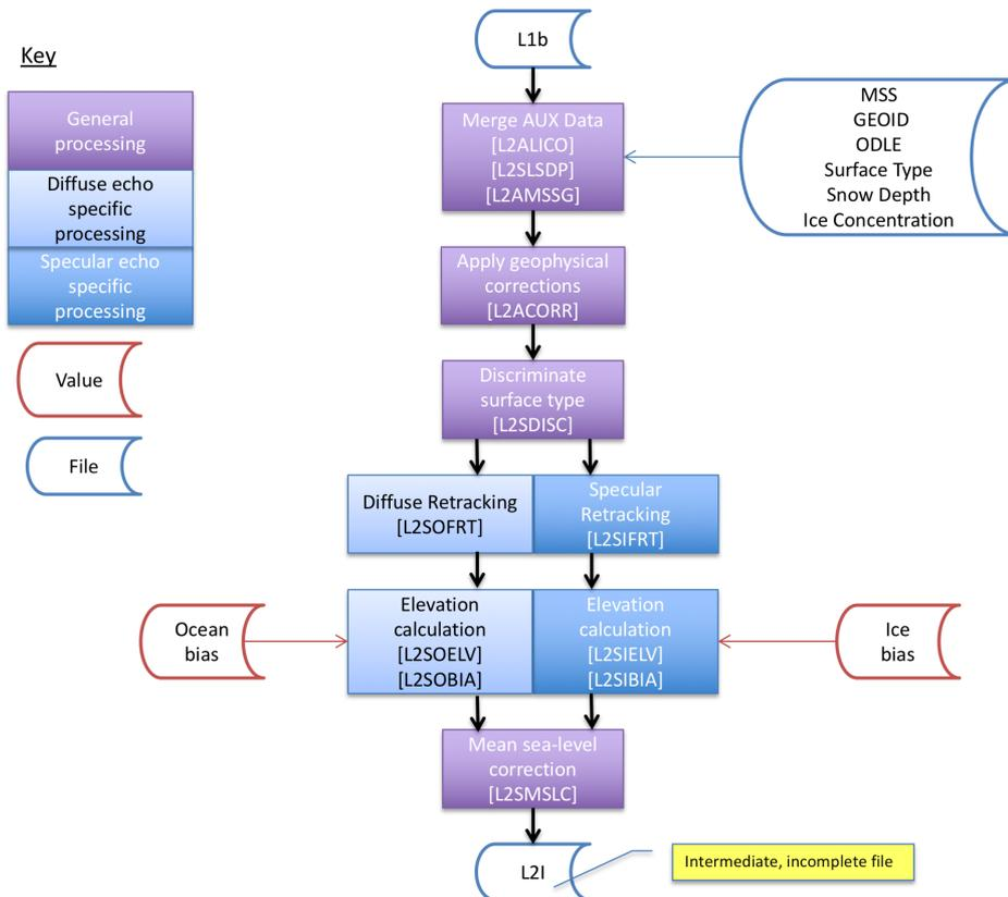
Figure 7: The SAR sea-ice pass A processing chain
