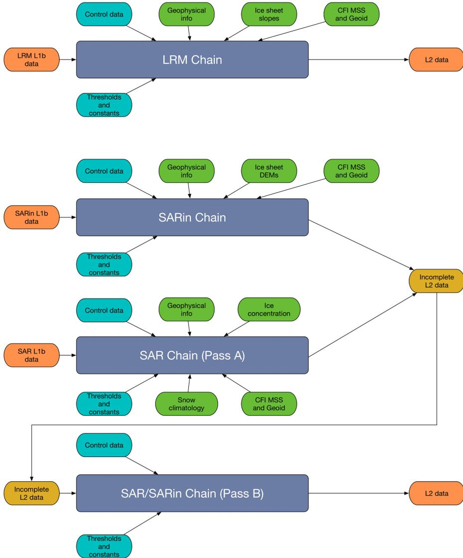
Figure 3: The processing chains within the CryoSat2 IPF2 processor
