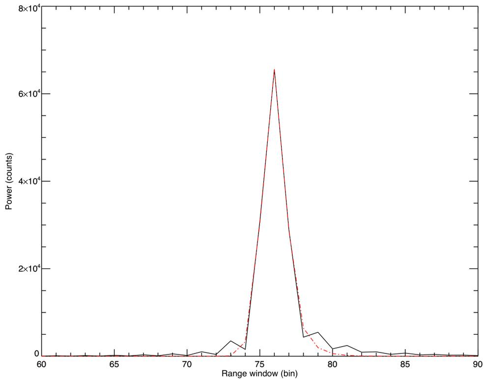
Figure 10: Typical specular SAR waveform from a lead and a corresponding model fit result (dashed)
