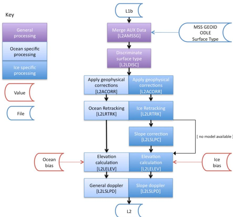
Figure 4: The CryoSat2 Level 2 LRM processing chain
