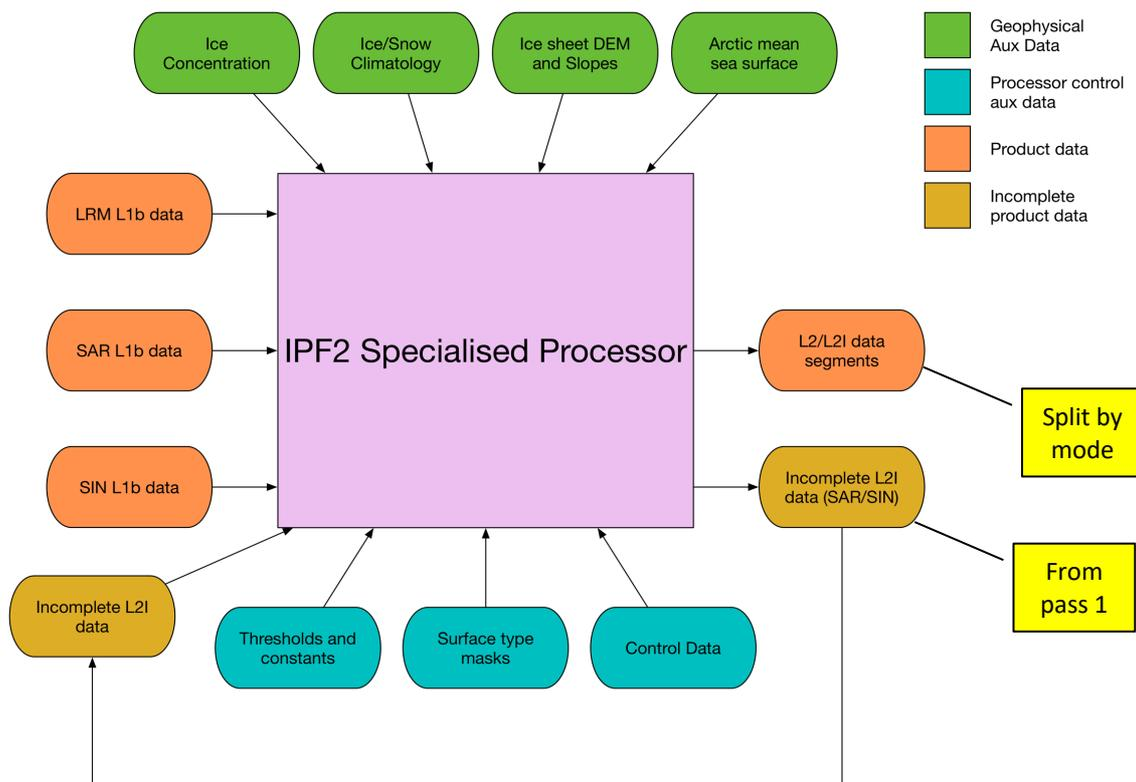
Figure 2: The context of the Level 2 specialised processor
