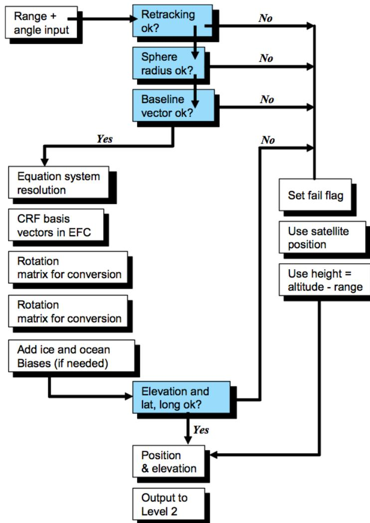
Figure 18: Elevation processing logic for SARin
