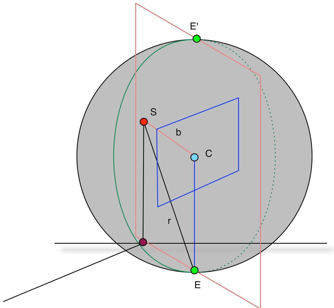
Figure 17: Geometry for SARin elevation calculation
