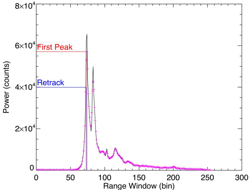
Figure 9: Typical diffuse SAR waveform from sea-ice
